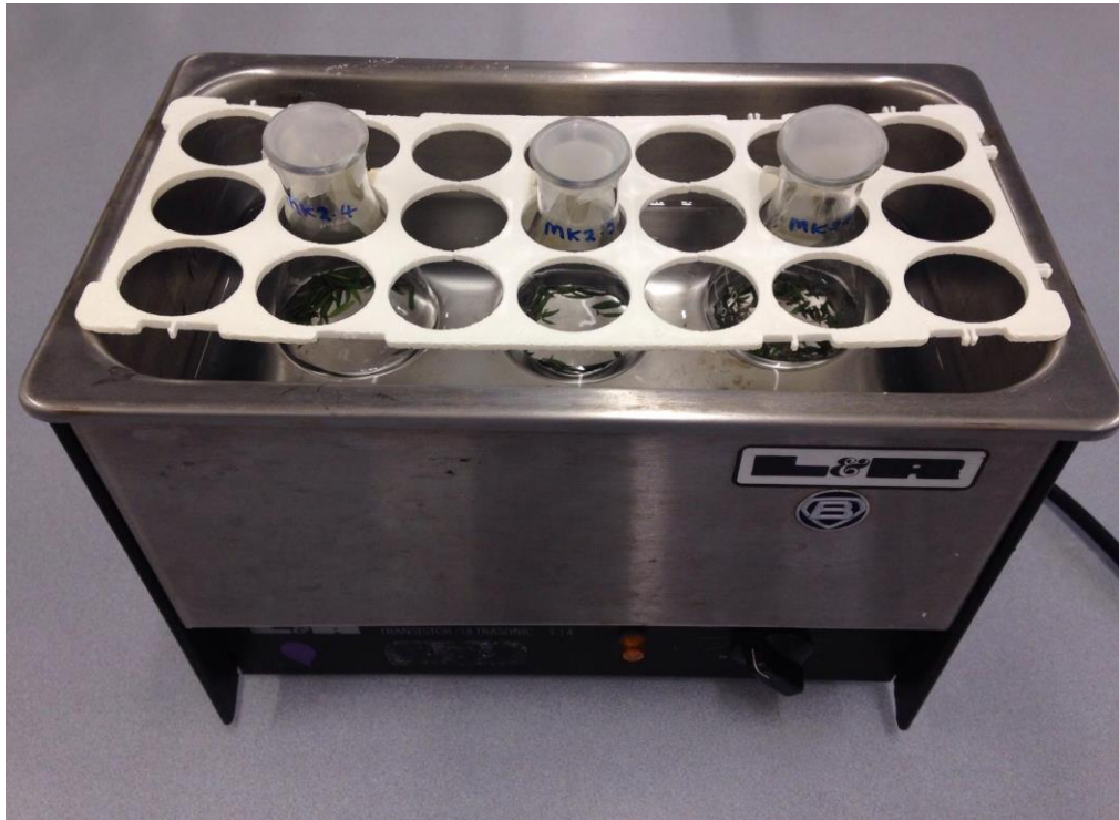
Figure 3.4: Manuka leaves submerged in 10 mL leaf wash buffer and placed in an ultrasonic cleaning bath
