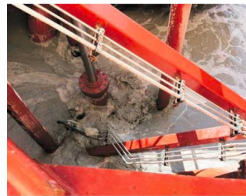
Image shows the structure of the discharge funnel from the hopper including the "green" or environmental valve. The purpose of the valve is to reduce the amount of air being discharged with the sediment, allowing the sediment to sink to the seabed faster, which reduces turbidity. Image: Willem de Lange.
