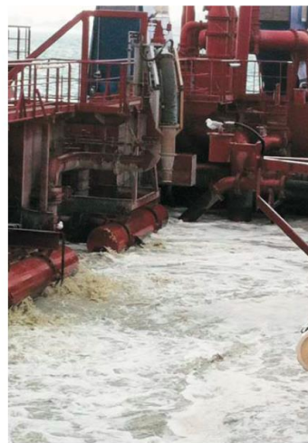
(Top image) This image shows the entrainment of air, which creates bubbles. At the top is an adjustable funnel that can be released and lowered to vary the rate of discharge, which also reduces the turbidity. Photo: Willem de Lange.
