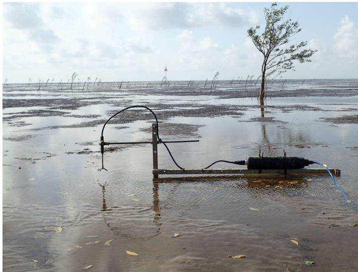
Figure 5.2: A solitary Vectrino Profiler deployed offshore of the mangrove fringe on the mudflat. Many juvenile Sonneratia caseolaris mangroves are visible in the distance.
