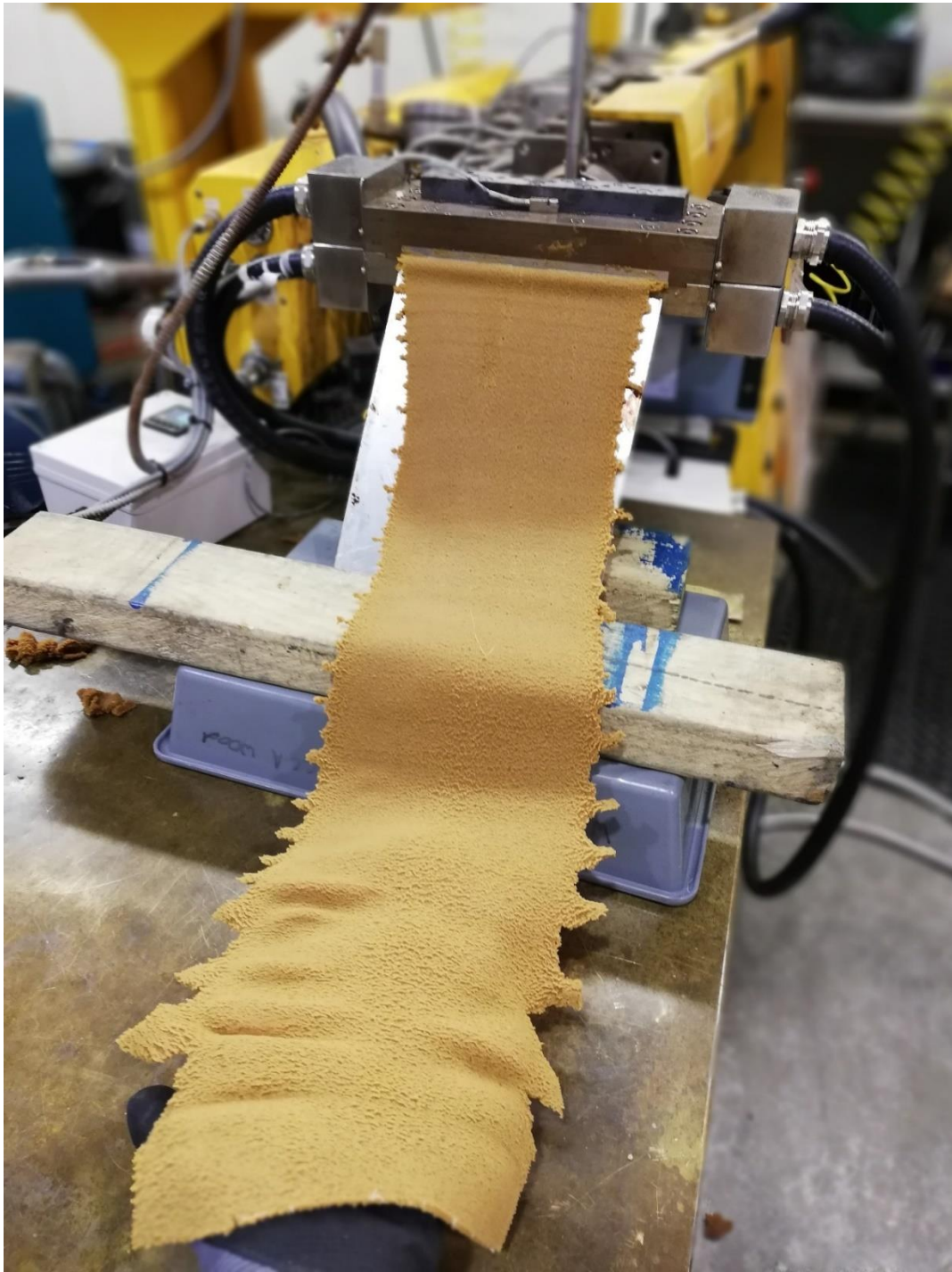
Figure 51: Twin-screw extrusion of DBT/PLA sheet using a LabTech twin screw co-rotating extruder.
