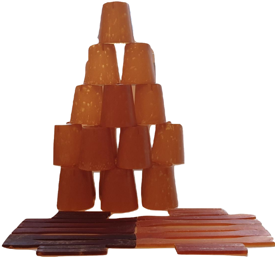
Figure 16: Agricultural plant pots and injection moulded samples made from decoloured thermoplastic
