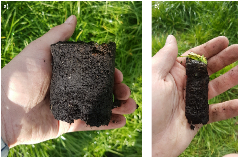
Figure 4.3 Soil cores: (a) large volumetric soil core used for soil physical property analysis and (b) small soil core used for soil chemical property analysis.
