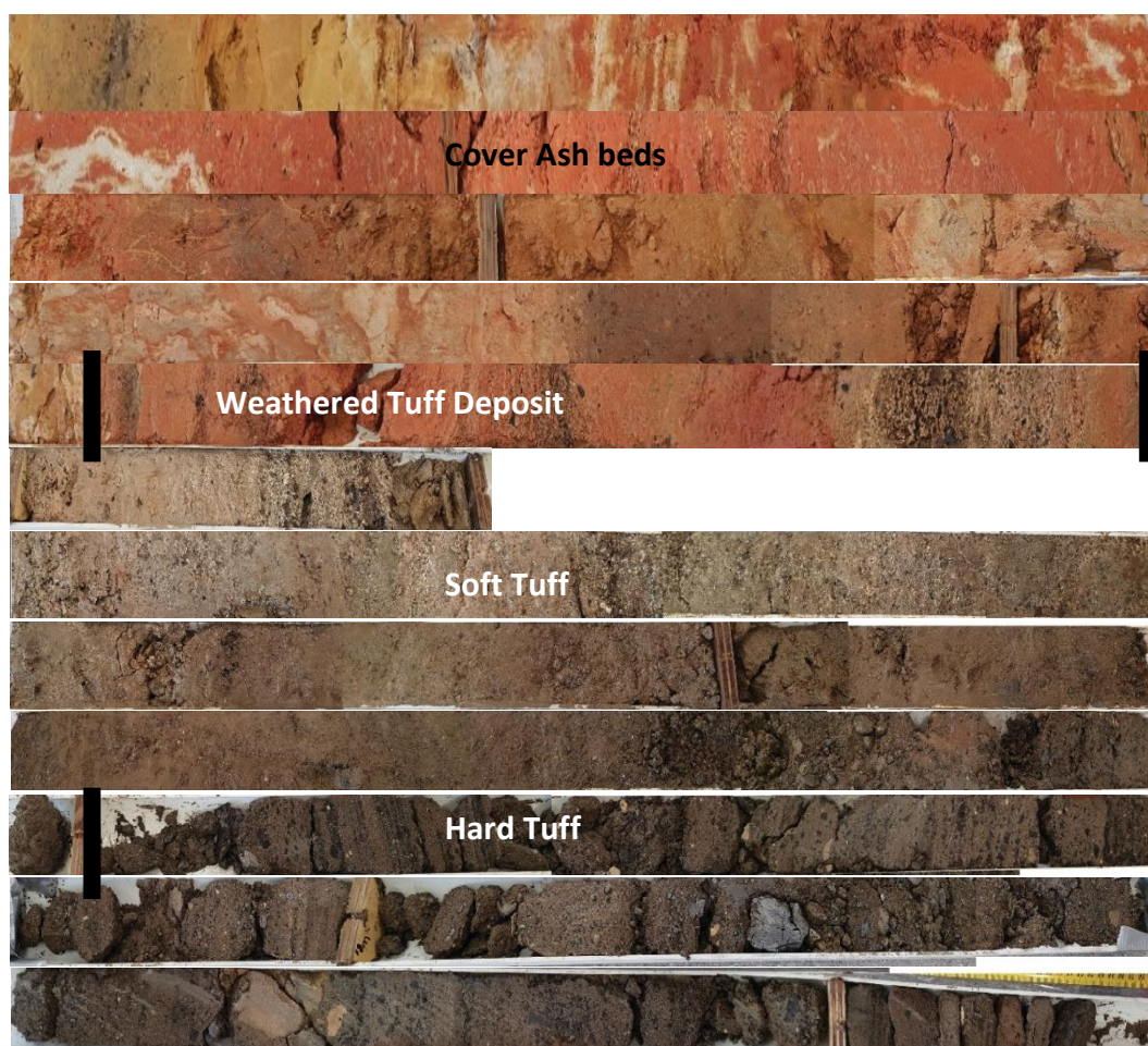
Figure 3.7: Material retrieved from DH2. The cover beds here are a different colour to those in DH1. Several sections of clay are interspersed with weathered basaltic material. Beneath the red clay is a grey matrix with basalt lapilli and lithics. The core material becomes consolidated near the base.
