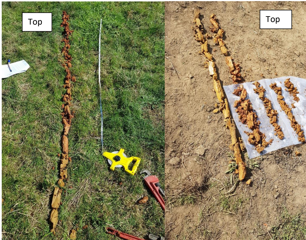
Figure 3.9: HA1 and HA2. These hand augers display the variation in cover clay beds over a small distance.
