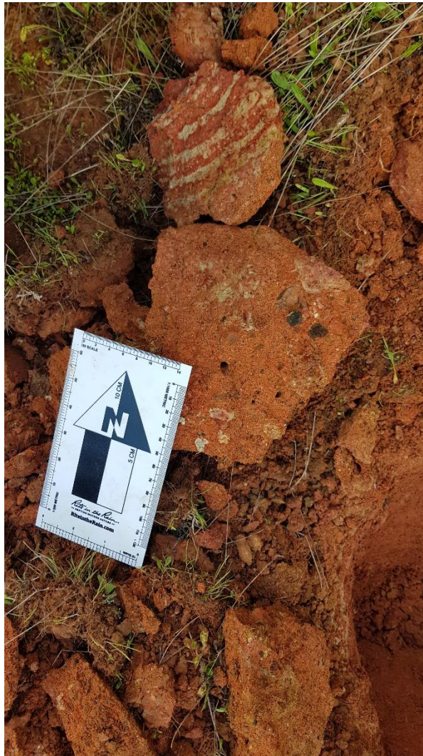
Figure 3.12: Weathered tuff found in a roadside swale. This image displays two distinct tuff patterns. Above is the layered red and grey clay and beneath is the orange to red clay with light and dark brown inclusions potentially of basalt lapilli and lithic material.
