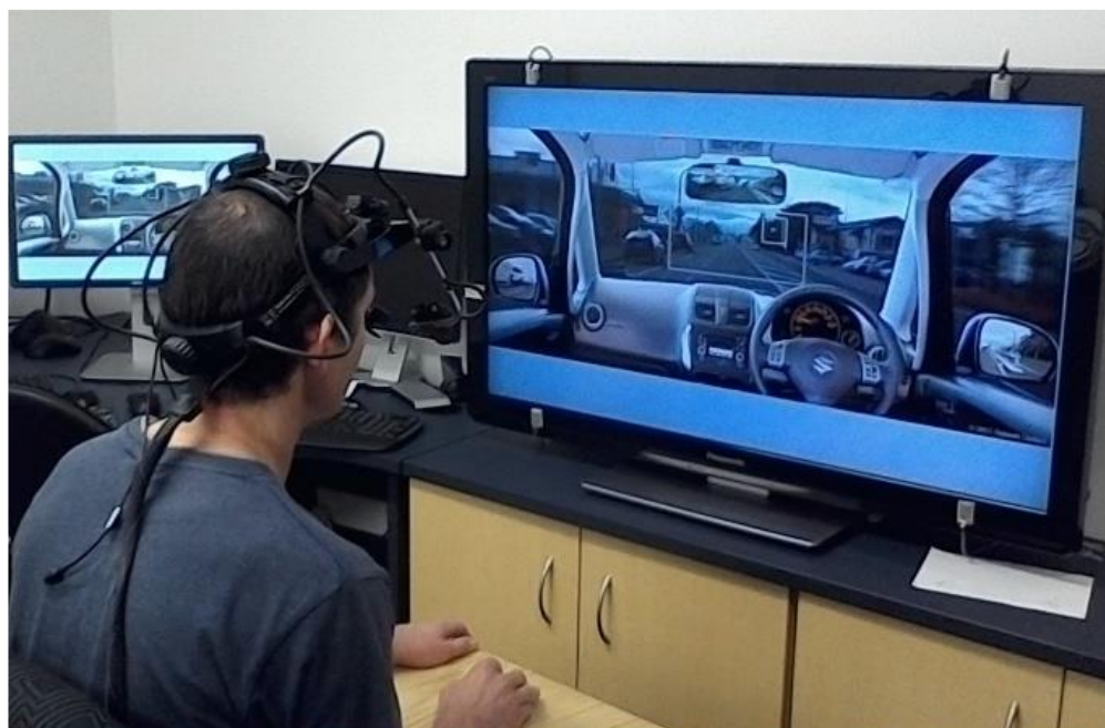
Figure 50: A participant demonstrating the use of the Head-mounted Eye-tracker while engaging in the Hazard Perception Task.
