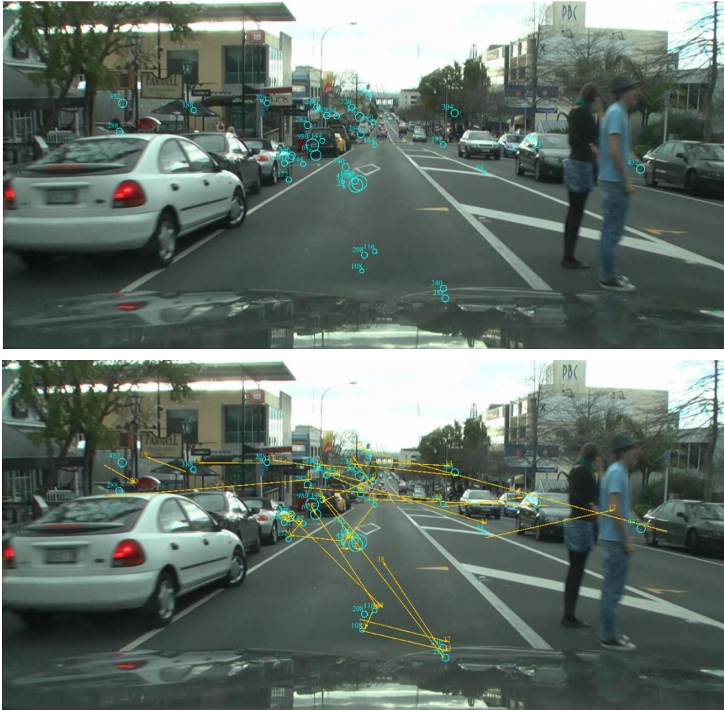
Figure 21: Fixations and Saccades, as shown in DataViewer™ (SR Research). Fixations are shown (top) as circles, with the diameter representing the duration. Saccadic eye movements (bottom) are presented as orange lines connecting fixations. The pattern of saccades, or ‘jumps’, between fixations can be used to determine the visual search strategy used.
