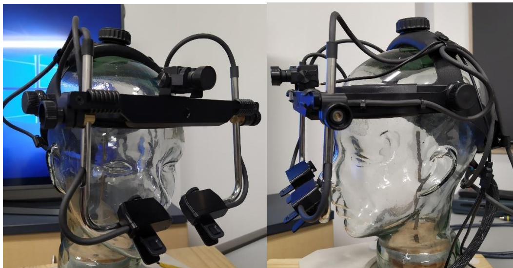
Figure 20: The binocular eye-tracker used throughout this thesis (EyeLink II™, SR Research). . As displayed, the Eye-tracker was secured to the participants head using three fastener straps, and two IR-cameras with IR-LEDs were used to record Binocular eye movements.
