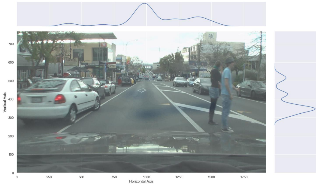
Figure 29: Representative Spatial Distribution of Fixations for Novice Drivers. Blue circles represent the Location of Fixations, and their size represents their Relative Duration in msec. The distribution plots show the horizontal and vertical spread of the distribution. The unit measure in pixels.
