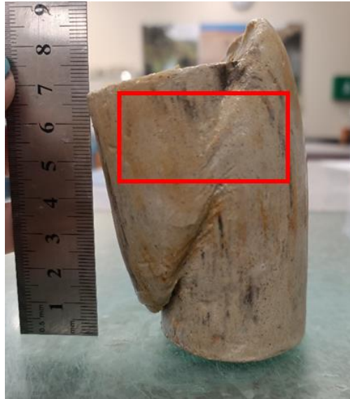
Figure 7.13. Image depicting the location on the core where the thin section was taken from, adjacent to the failure surface.
