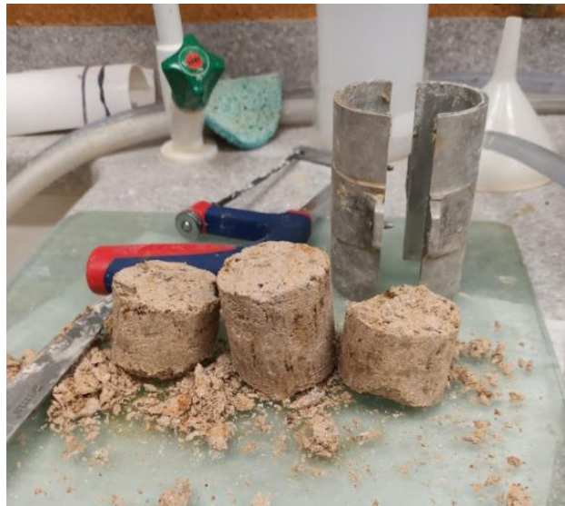
Figure 7.19. Image showing the condition of the TV2 cores during extraction. The granular nature of the cores in addition to the moisture content disallowed successful core extraction and trimming.
