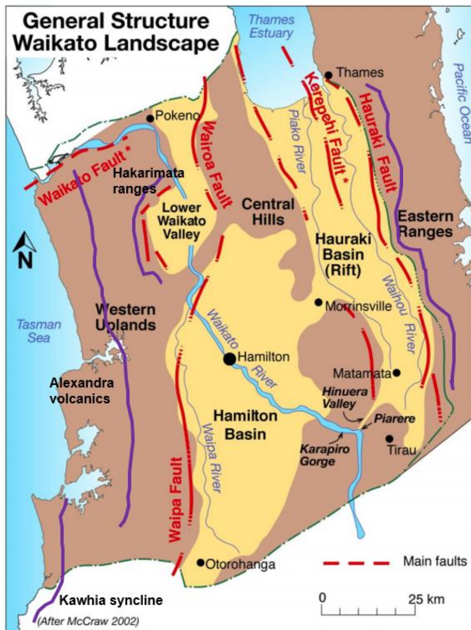
Figure 2.1. Schematic of the Hamilton Basin, detailing the general basin structure. The purple lines indicate the mountain ranges of the region, as described above (Lowe, 2010).
