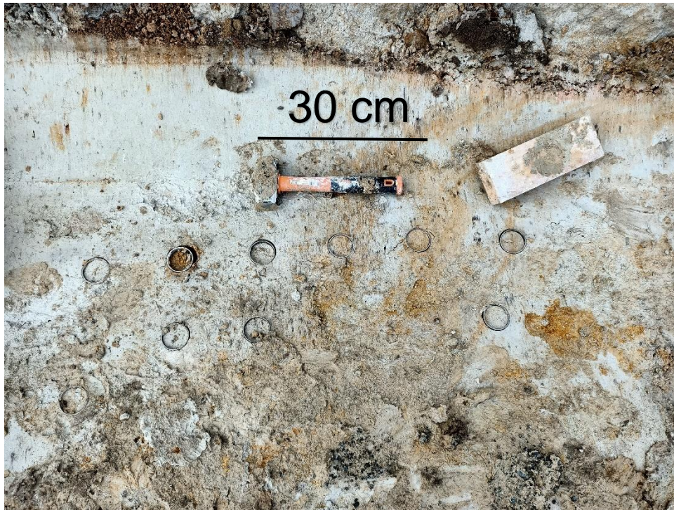
Figure 4.6. Figure showing ten of the twelve triaxial cores hammered into the cleared bench of Puketoka Formation material (30cm mallet for scale) (Kitchen, 2021).
