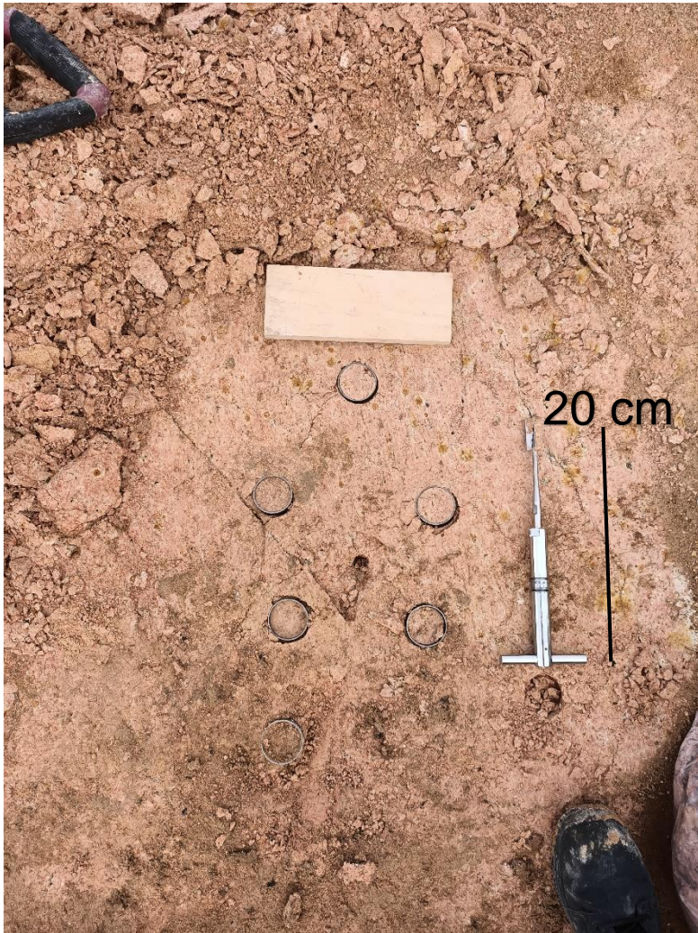
Figure 4.9. Image showing the level platform scraped prior to triaxial core extraction of the upper Puketoka Formation materials (20 cm shear vane to scale).
