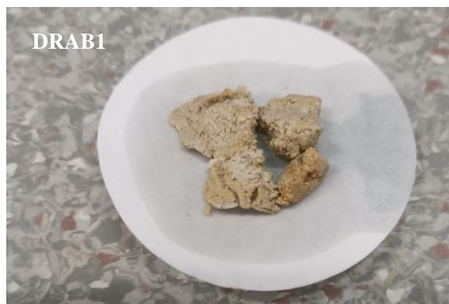
Figure 6.9. Image showing the results of the Fieldes and Perrott NaF test for allophane. The lack of pink colouration upon the paper indicates absence of allophane after 5 minutes of exposure.
