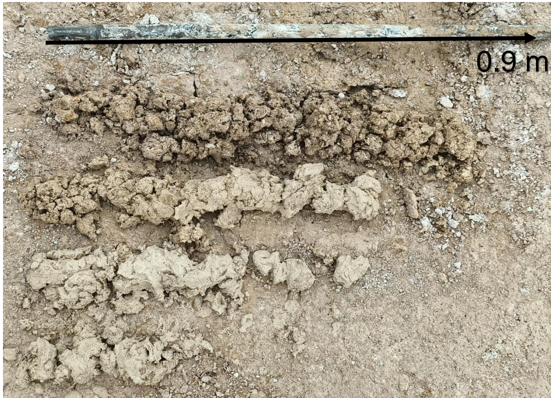
Figure 4.13. Photo showing a typical hand auger completed within the Puketoka Formation, to 3 metres depth (0.9m hand auger rod for scale), with rows laid out from left to right, in addition to field notes logging the formation, using New Zealand Geotechnical Society 2005 logging conventions.
