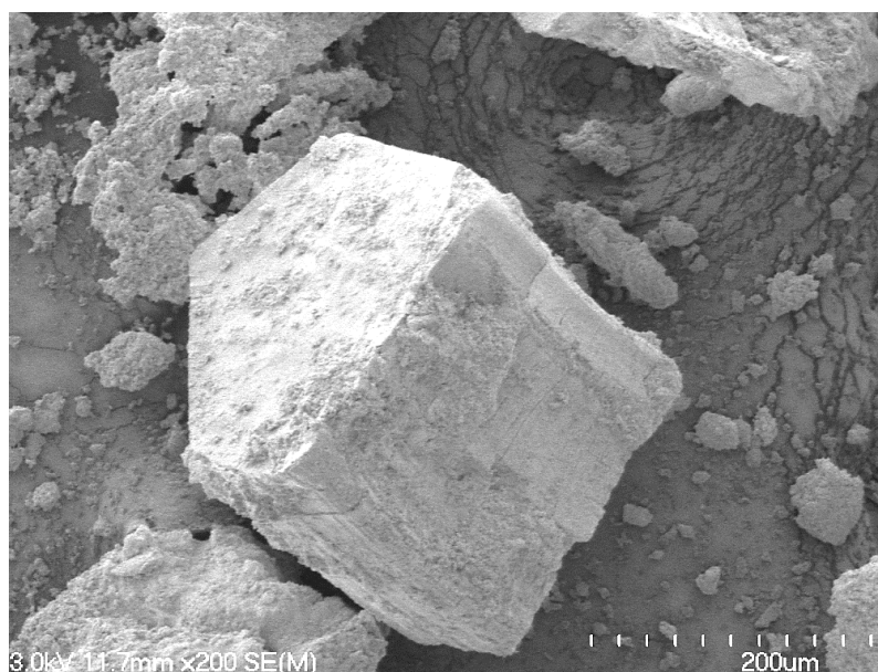
Figure 8.36. SEM image depicting a large, blocky grain identified within the more cohesive portion of the TV1 sample. The grain is 180 μm in diameter, and appears to be foliated, similar to the book formations identified in TV1 and TV2. The grain is also finely covered in grain coatings across the exposed surfaces. This grain is hypothesised to be micaceous.
