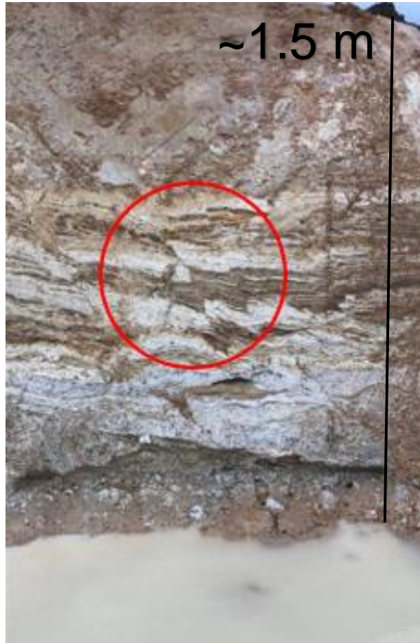
Figure 4.3. Image showing evidence of the faulting found within the Dixon Road Roundabout site cuttings, which could pose an issue to the sensitive sediments within the site if seismic activity were to occur. Note the bedding of the layers observed, separated by dark brown layers (Lethborg, 24th July 2020).
