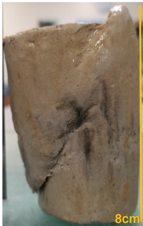
Figure 9.1. Image showing the extent of strain localisation (shear band formation) occurring within areas of manganese concentrations within a failed triaxial core sample (DRAB1 130 kPa).
