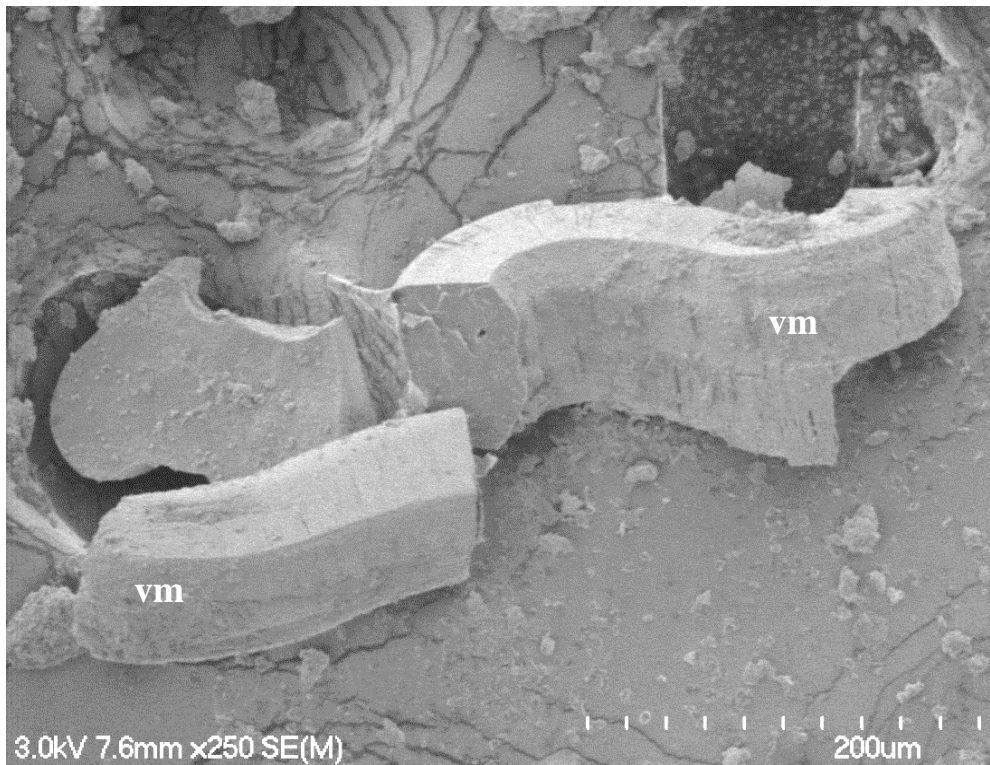
Figure 8.15. SEM image depicting the presence of two vermiform book (vm) forms radiating away from one another at a common point in TV2. The books range from 200 to 250 \mu\text{m} in size, and display face to edge contacts.
