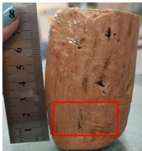
Figure 7.15. Image showing the location of the thin section taken from the TV1 230 kPa thin section, adjacent to the failure surface.
