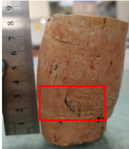
Figure 7.14. Image showing the location the 130 kPa thin section, adjacent to the failure surface.
