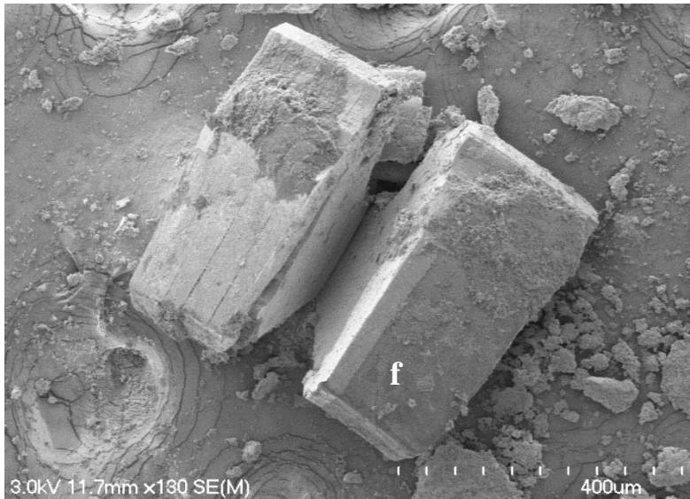
Figure 8.34. SEM image showing a hypothesised feldspar (f) grain identified within the more granular portion of the TV1 sample. This grain is extremely large in size (458 μm), and appears to have split down the middle as a result of sample preparation.
