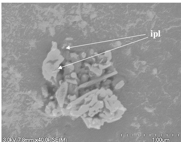
Figure 8.9. SEM image showing the presence of irregularly shaped plates within TV1, denoted by ipl. The plates range between 0.3 and 0.6 µm in TV1. Due to the limitations of the SEM it is challenging to determine the depth and true shape of the plates.
