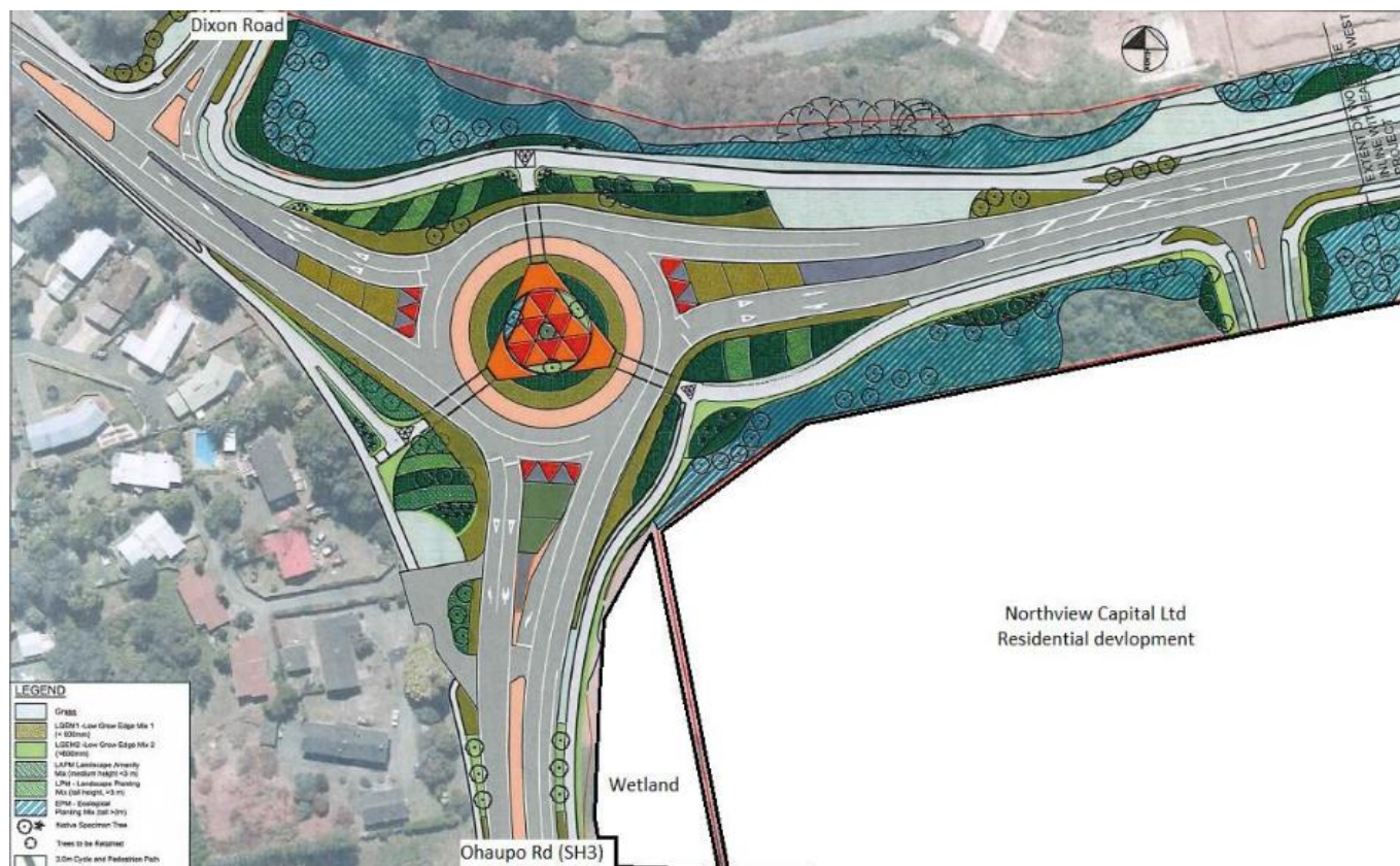
Figure 4.1. Diagram showing the site of the construction of the Peacocke State Highway 3 (SH3) roundabout in Southern Hamilton (Hamilton City Council, 2020).
