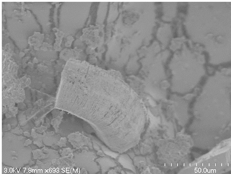
Figure 8.59. SEM image showing another example of the vermiform book formations analysed within the TV2 samples. This book formation measured 82.1 μm in length and 41 μm in diameter.
