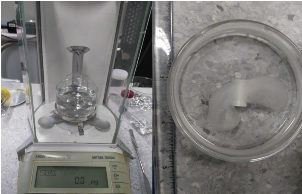
Figure 5.21: a) Archimedes setup for porosity measurement and b) evolving bubbles from the sintered sample when immersed in water
