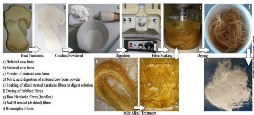
Figure 6.1: A pictorial representation of the processing steps, which summarises production of the digest solution containing calcium and phosphate ions and the soaking and calcination of the NaOH treated harakeke fibres in the solution, resulting in the production of the biomorphic fibres.
