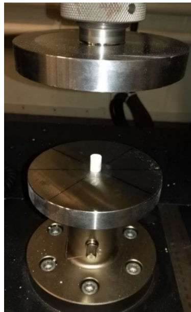
Figure 5.26: Composite sample ready to be compression tested on the universal testing machine (UTM).
