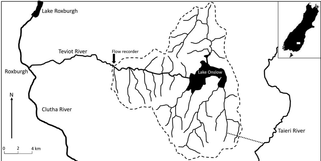
**Figure 1** – Lake Onslow and the Teviot River catchment (dashed line) upstream of the Bridge Huts Road flow recording site (vertical arrow). The dotted line is a possible tunnel location for transfer of water from the Taieri River to the Lake Onslow basin (see text).
