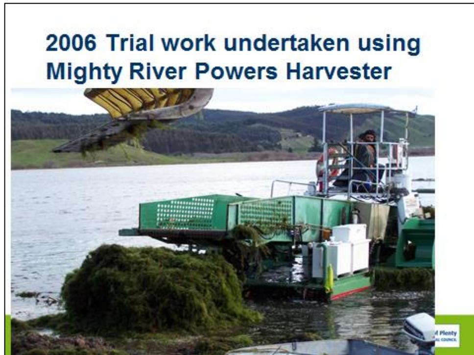
Other current initiatives which were put into place in that catchment included the land management change, phosphorus locking, artificial wetlands and aeration, but it was hoped that the end result might be the removal of 2-3 tonnes of nitrogen through harvesting as well. Harvesting operated from 2006 through to 2012 with Mighty River Power's harvester, the photo below taken relatively late in the harvesting season. Much of the weed had started to die back down and most had been removed.
