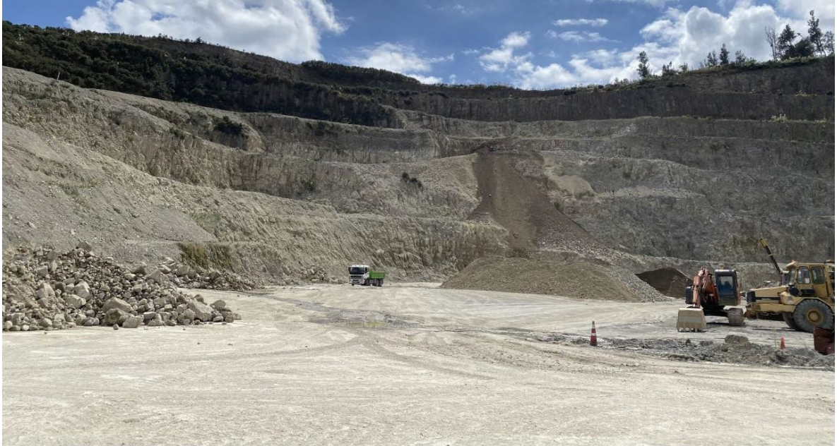
Figure 4.9: Greenpark Quarry showing a light-coloured rhyolite on the left hand side and a darker rhyolite on the right hand side, which has been previously classified as andesite.
