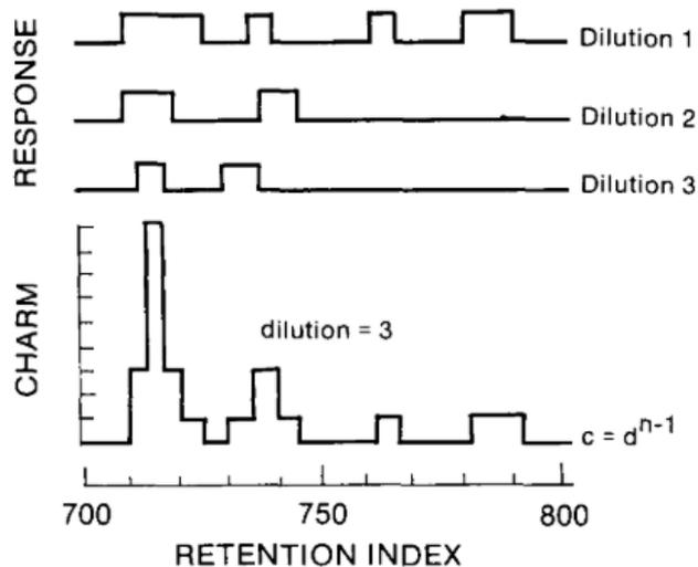
**Figure 3. A stylised charm response chromatogram produced from the relationship  $c = d^{n-1}$ , where  $d$  is the dilution constant and  $n$  is the number of coincident responses at any given index. Reproduced with permission from Acree et al. (1984).<sup>45</sup>**
