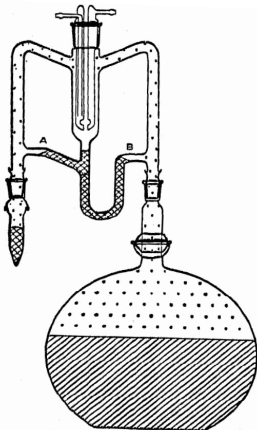
**Figure 6. Likens-Nickerson apparatus for steam distillation extraction. Reproduced with permission from Nickerson and Likens (1966).<sup>126</sup>**
