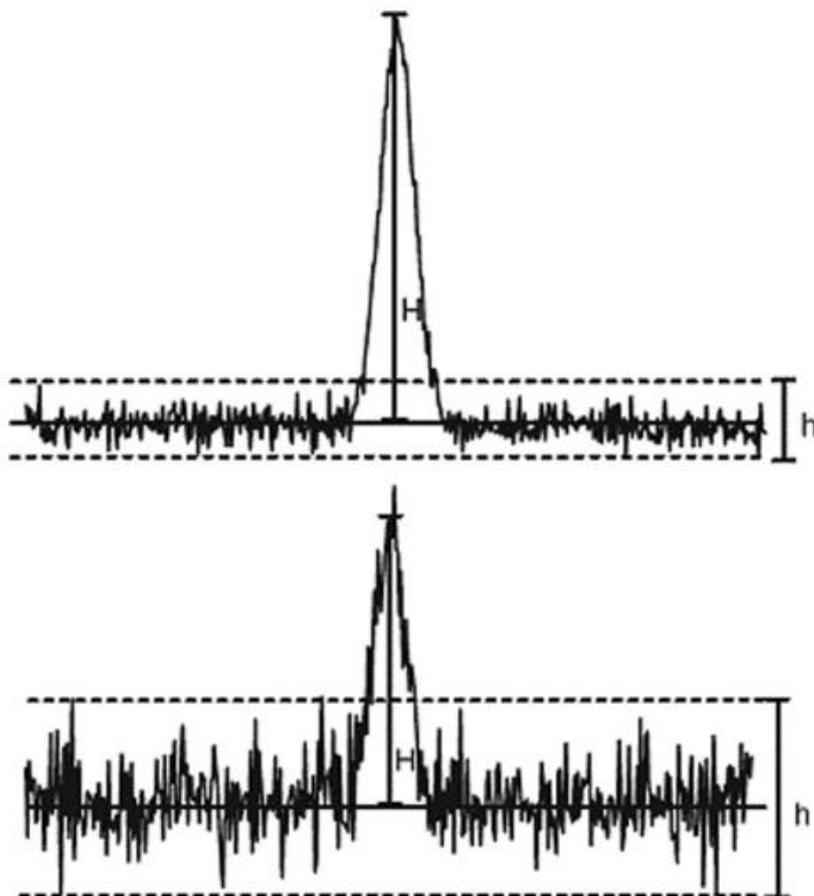
**Figure 27. Signal-to-noise examples of 10:1 (top) and 3:1 (bottom), using the method of the European Pharmacopoeia.  $SNR=2H/h$ , where  $H$  is the peak height, measured from the top of the peak to the baseline, as extrapolated over a distance equal to 20 times the peak width at half height.  $h$  is the peak height of the baseline noise observed in this region. *Reproduced from Alankar & Vipin (2011)*<sup>176</sup> (open access).**
