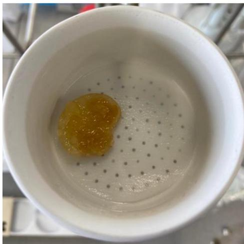
**Figure 16. Wax and water frozen and filtered from honey extract using glass microfibre filter paper.**
