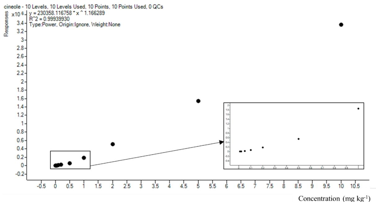
**Figure 23.** Calibration curve of cineole from  $10 \mu\text{g kg}^{-1}$  to  $10 \text{mg kg}^{-1}$ . Over such a wide concentration range, a linear relationship between concentration and instrument response could not be achieved and the slope of the graph significantly changed above  $1 \text{mg kg}^{-1}$ .
