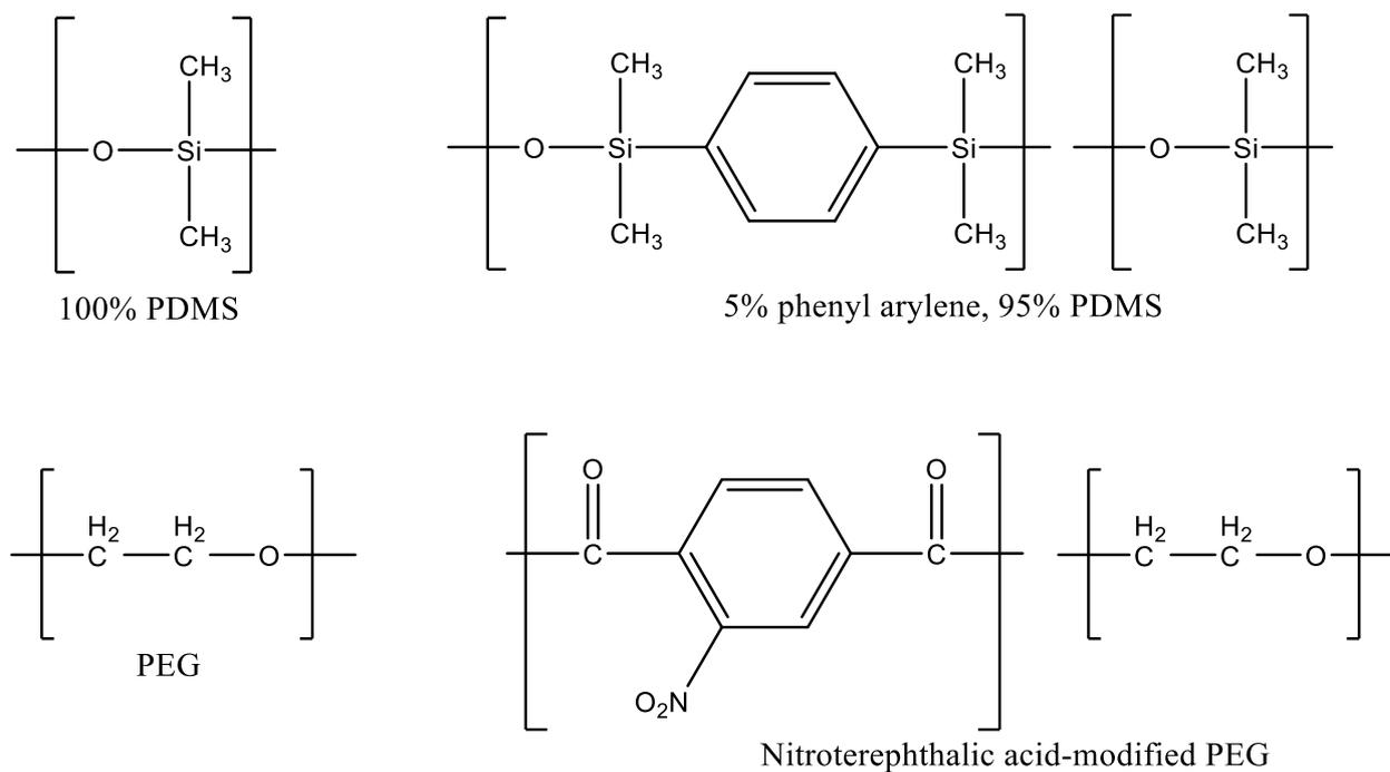
**Figure 19. Common stationary phases used for the analysis of volatile compounds in honey by GC-MS.**
