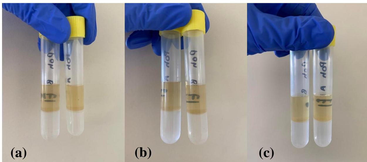
**Figure 18.** Separation of organic (bottom) and aqueous (top) phases after (a) 10 min, (b) 20 min, and (c) 30 min centrifugation at 3900 rpm at 4 °C.
