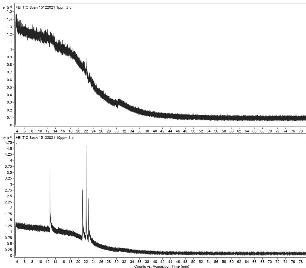
**Figure 13. Chromatograms of artificial honey containing aroma compounds spiked at 1 mg kg<sup>-1</sup> (top) and 10 mg kg<sup>-1</sup> (bottom). No peaks are visible at 1 mg kg<sup>-1</sup>, while at 10 mg kg<sup>-1</sup> benzaldehyde (12.60 min), guaiacol (21.13 min), linalool (22.02 min) and 2-phenylethanol (22.69 min) are visible.**
