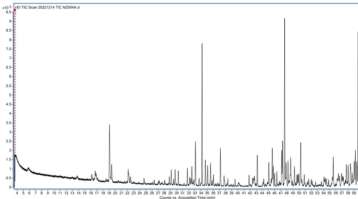
**Figure 38. TIC chromatogram of a typical kāmahi honey (NZ004). Important peaks include *D*-limonene (16.7 min), 4-oxoisophorone (24.7 min), octanoic acid (27.6 min), hotrienol (28.1 min) and 3,5-bis(1,1-dimethylethyl)-phenol (48.5 min).**
