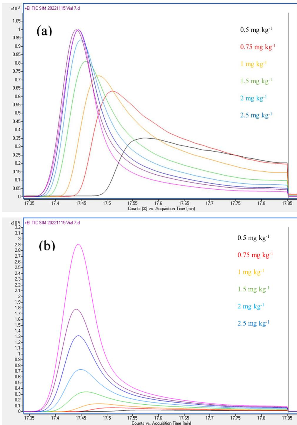
**Figure 28. The peak shape and RT of benzyl alcohol peaks varied with concentration. RT decreased with increasing concentration. The peaks also displayed significant tailing, which resulted in a portion of the peak being cut off at the end of the SIM segment (17.85 min). a) Peak height is not to scale in this figure to better display the peak shapes, b) peak height to scale.**
