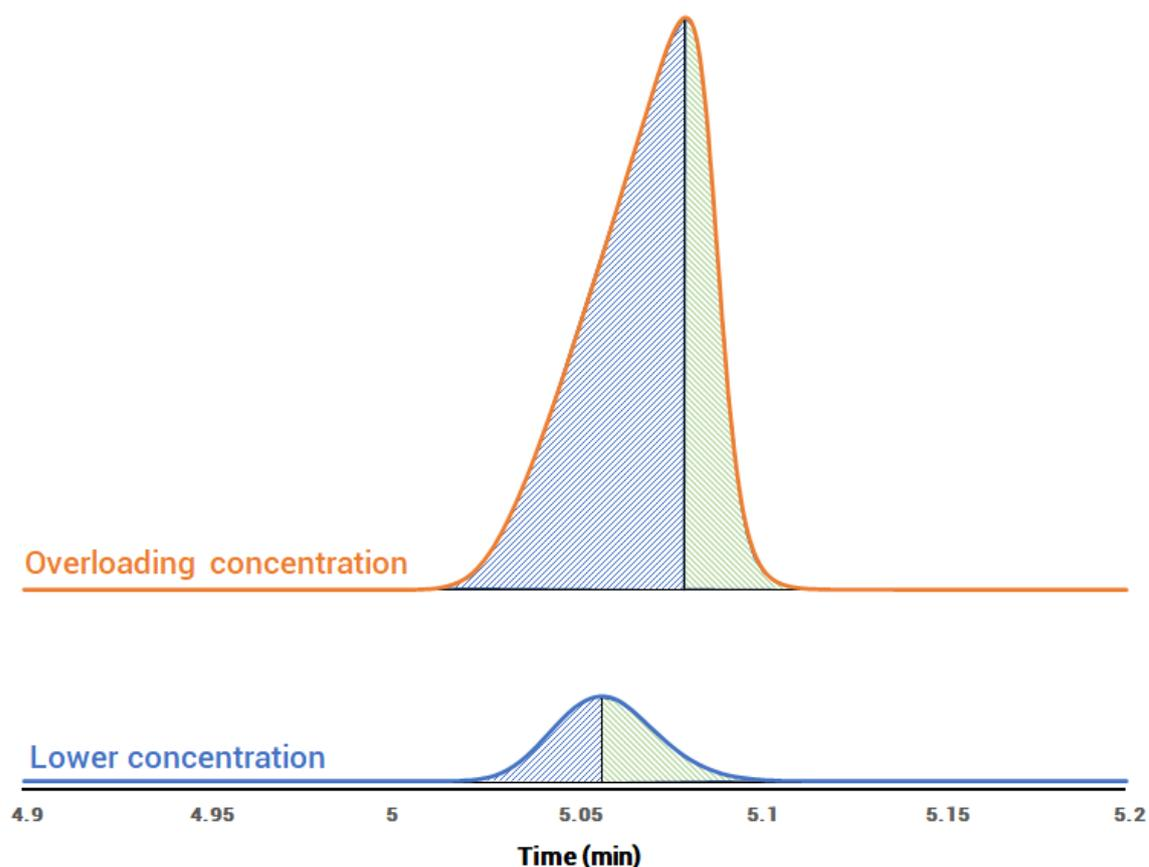
**Figure 21. Shape of a fronting peak (top) due to overloading of analyte, vs ideal peak shape obtained at a lower analyte concentration (bottom). Reproduced with permission from PerkinElmer (2022).<sup>172</sup>**
