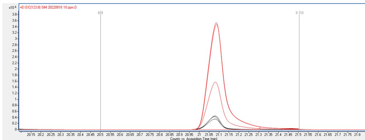
**Figure 22.** Section of the SIM chromatogram for a spiked honey sample, showing the separation of the co-eluting guaiacol (red) and linalool oxide isomer 2 (black) based on characteristic ions of each compound.
