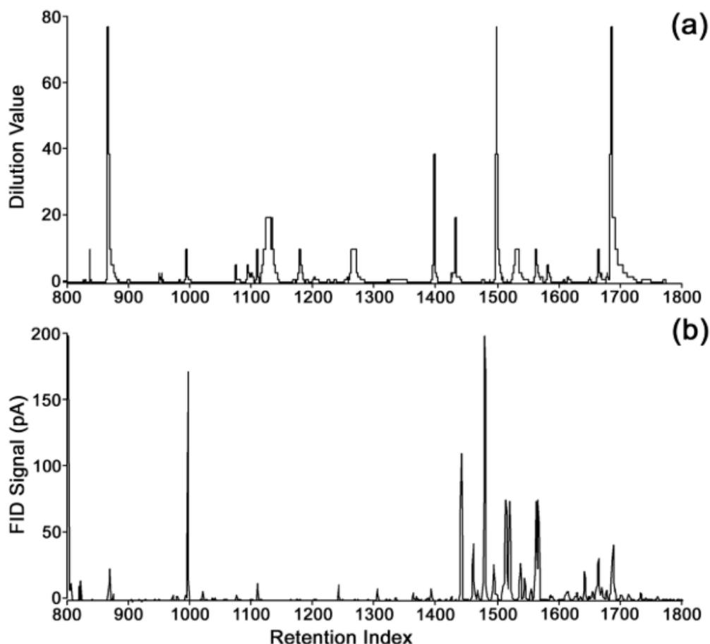
**Figure 2. Comparison of (a) the GC-O aromagram generated using charm analysis with (b) the FID chromatogram for a hop essential oil sample. Reproduced with permission from Delahunty *et al.* (2006).<sup>42</sup>**
