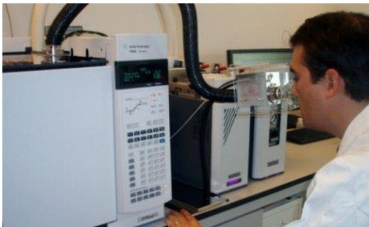
**Figure 1. Odour assessor sniffing the eluting compounds from a GC separation using an olfactometry port. Image copyright Sensnet holding BV, used with permission.<sup>44</sup>**
