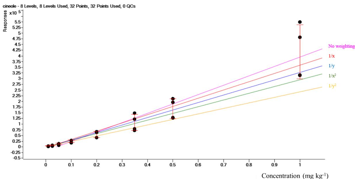
**Figure 26. Calibration curves for cineole using various weighting factors.**
