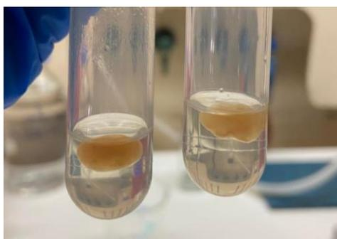
**Figure 14. Waxy emulsion layer formed during solvent extraction with DCM.**
