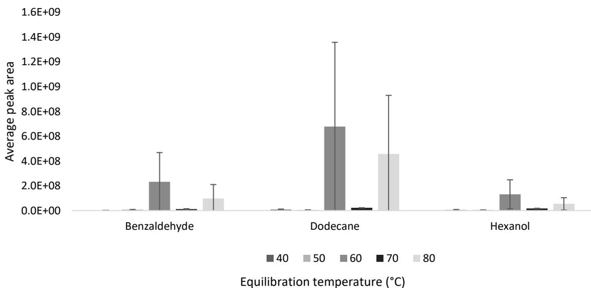
**Figure 10.** Average peak area of benzaldehyde, dodecane and hexanol at different equilibration temperatures in artificial honey (n = 3). Error bars represent one standard deviation in result.
