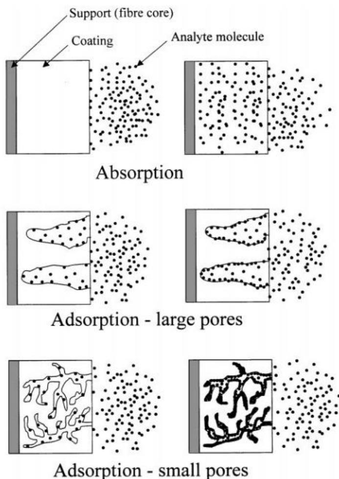
**Figure 7.** Comparison of absorption and adsorption extraction mechanisms (cross-sections of the coated fibres). Diagrams on the left illustrate the initial stages of the processes. Diagrams on the right illustrate the steady state condition. *Reproduced with permission from Górecki et al (1999).*<sup>145</sup>
