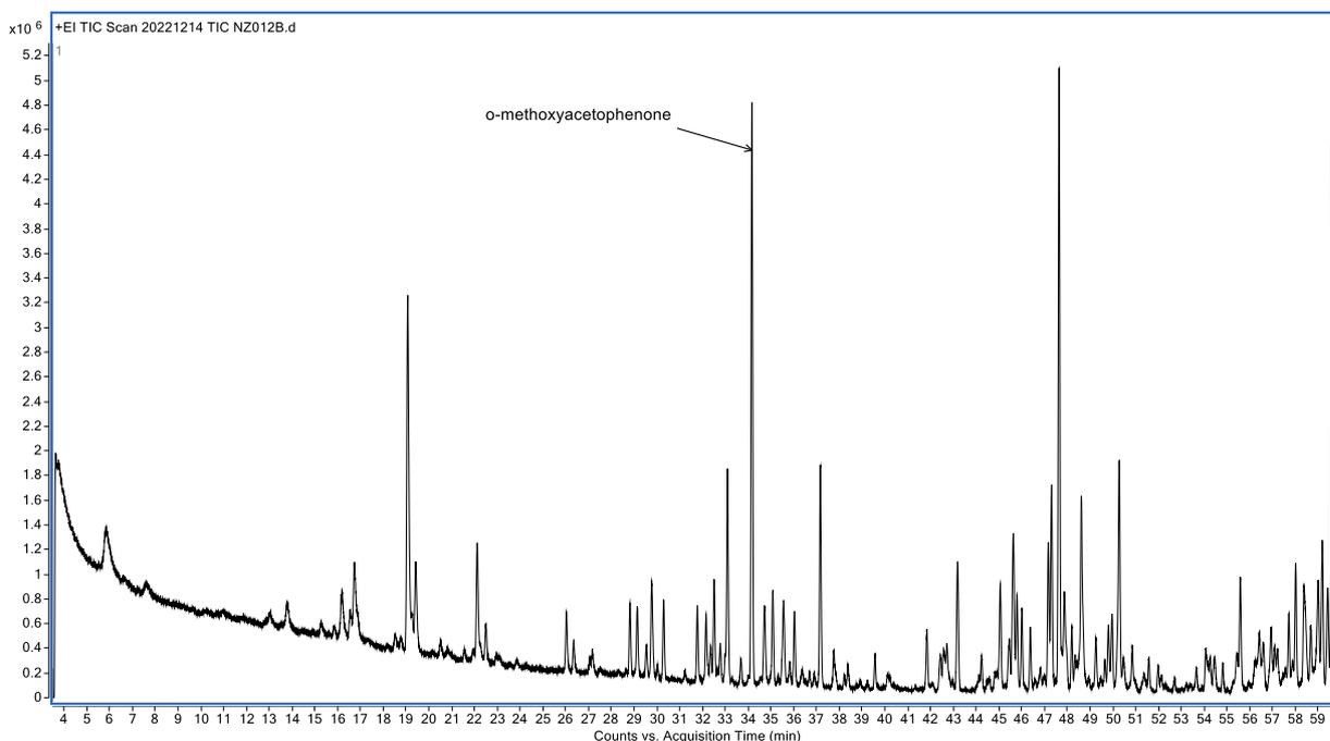
**Figure 32. TIC chromatogram of a typical mānuka honey (NZ012). Labelled peak is *o*-methoxyacetophenone (34.7 min).**
