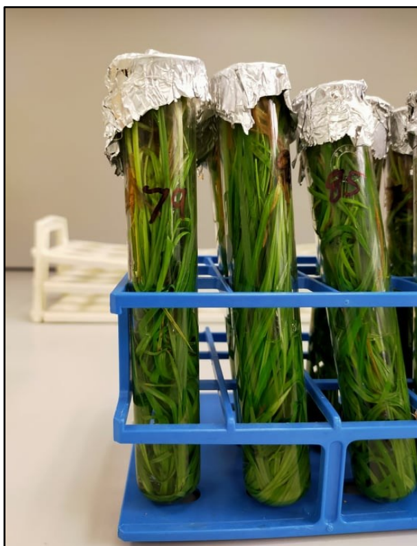
Figure 2.6: An image of the glass tube set up before sonication. Note that the ryegrass cut ends are facing upwards, with the uncut ends of the shoot facing down.
