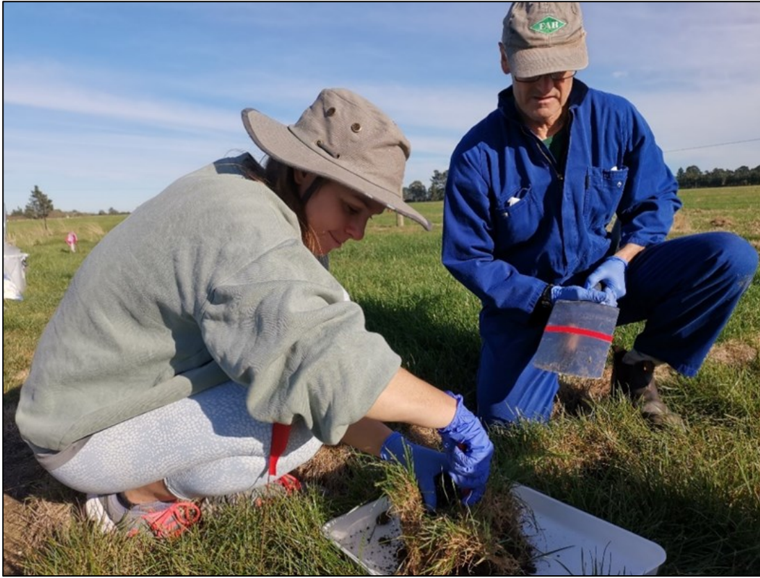
Figure 2.3: Photo of myself (Bernadette) and Mark McNeil (AgResearch) demonstrating the spade, tray and knife method (B) for extracting 10cm cores at the NFVT Burnham site.
