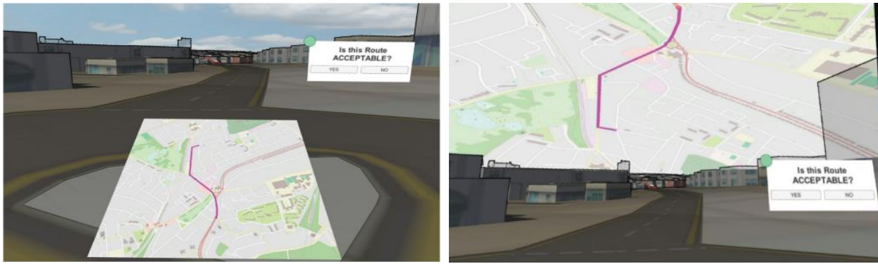
Figure 2. 49 Navigation interface displayed on the top and bottom views of the display. From “A mirror in the sky: assessment of an augmented reality method for depicting navigational information” by A. J. Reiner, J. G. Hollands, G. A. Jamieson, and S. Boustila, 2020, Ergonomics , 63(5), p. 553 ( https://doi.org/10.1080/00140139.2020.1737738 ). Copyright 2020 by Taylor & Francis.
