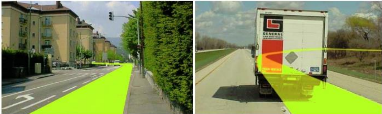
Figure 2. 32 Translucent path for navigation Reprinted with permission. From “A new visualization concept for navigation systems.” by W. Narzt, G. Pomberger, A. Ferscha, D. Kolb, R. Müller, J. Wieghardt, and C. Lindinger, 2004, ERCIM Workshop on User Interfaces for All, p. 442( https://doi.org/10.1007/978-3-540-30111-0_38 ). Reprinted with permission.
