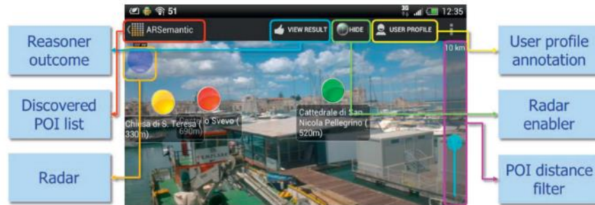
Figure 2. 52 Visual POI with the related information. From “A semantic-enhanced augmented reality tool for OpenStreetMap POI discovery” by M. Ruta, F. Scioscia, D. De Filippis, S. Ieva, M. Binetti, and E. Di Sciascio, Transportation Research Procedia , 3, p. 486 ( https://doi.org/10.1016/j.trpro.2014.10.029 ). Reprinted with permission.
