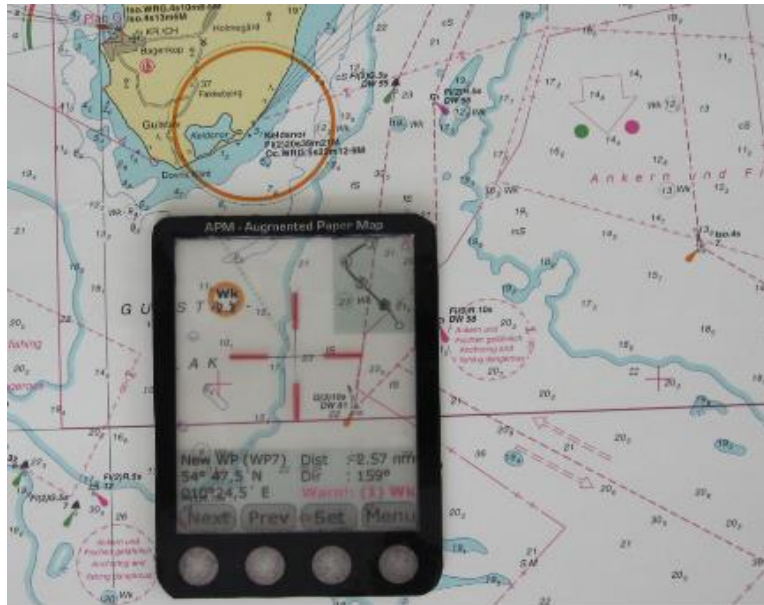
Figure 2. 7 A physical concept of the APM. From “Augmented paper maps: Exploring the design space of a mixed reality system,” by V. Paelke, and M. Sester, 2010, ISPRS Journal of Photogrammetry and Remote Sensing , 65(3), p. 261( https://10.1016/j.isprsjprs.2009.05.006 ), Reprinted with permission.
