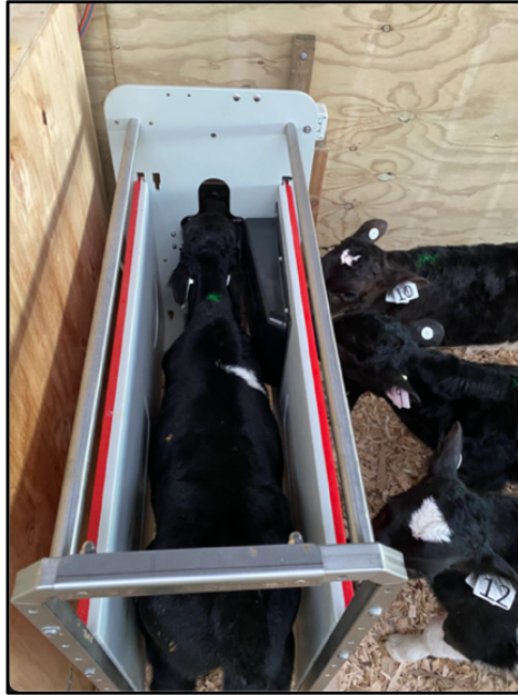
Figure 2.2. Automatic Lely calf feeder, milk drinking station setup.
