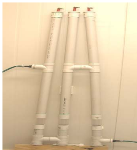
Figure 2.5. Oxygen reduction system and diagram showing oxygen stripping process.
