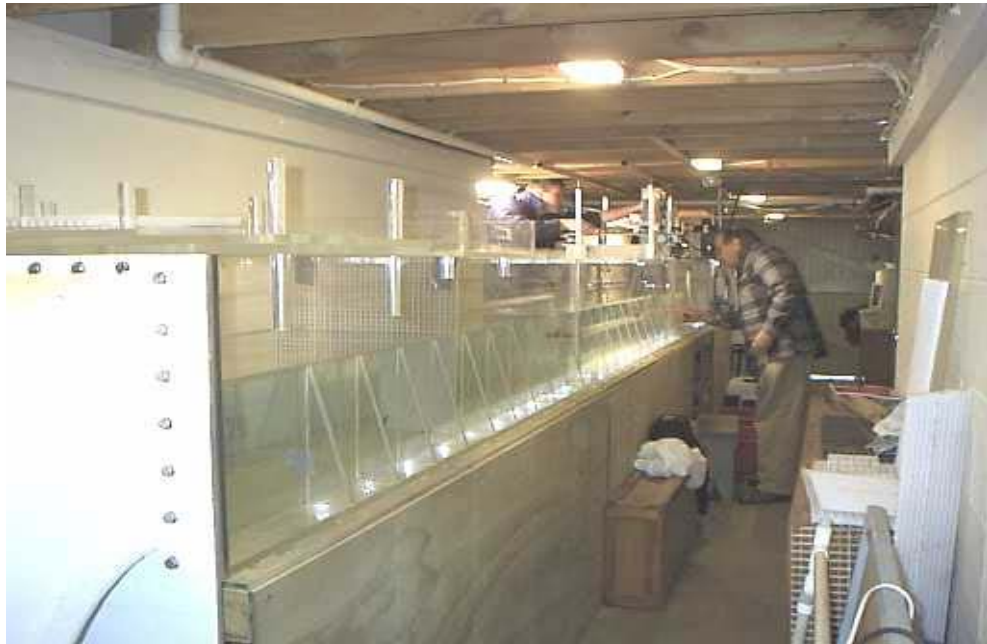
Figure 2.1. The 7.23 m long, 0.5 m wide, and 0.5 m deep acrylic flume.
