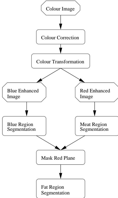
Figure 1: Block Diagram of Colour Processing
