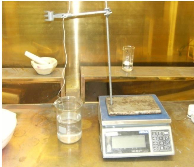
**Figure 3.5** Set-up for density measurement.
