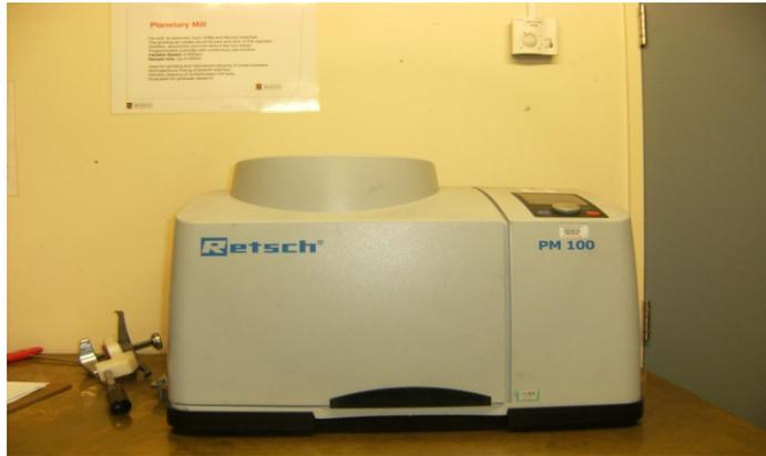
Figure 3.2 Retsch planetary ball milling machine.
