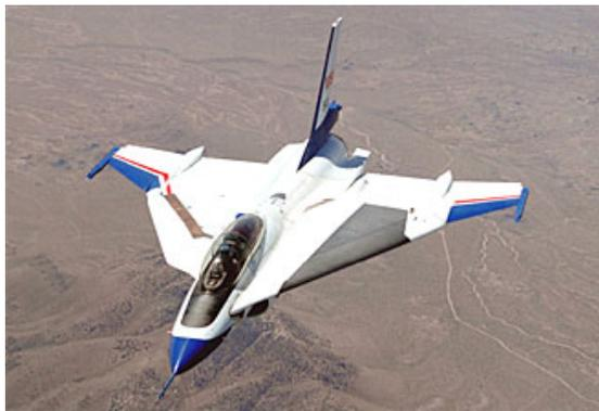
**Figure 2.2** Porous titanium LFC on the left wing of aircraft. [40]
