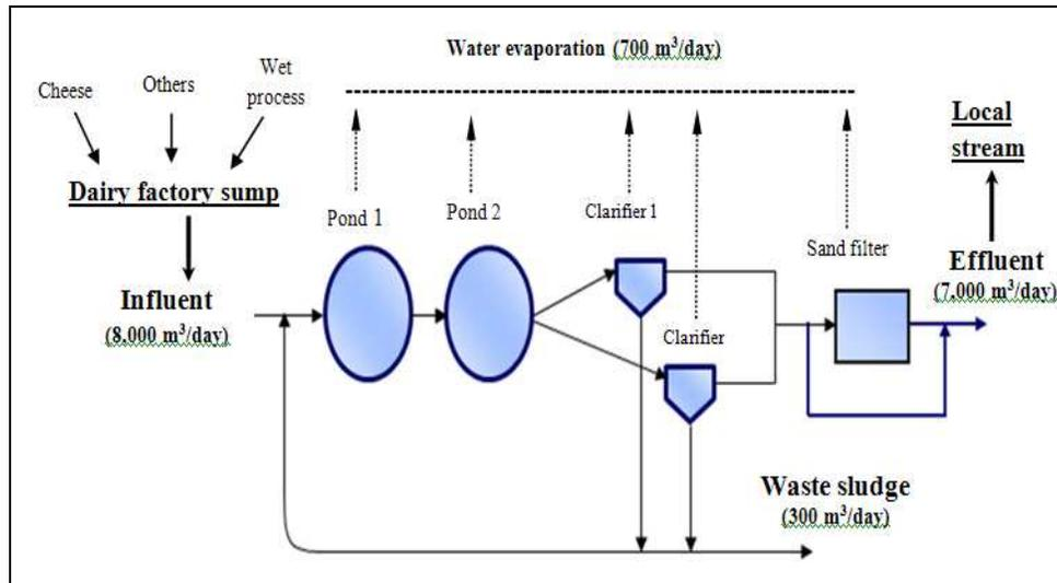
**Figure 4.2** Schematic wastewater biological treatment flow diagram in an extended aeration sludge system at the Waitoa dairy site.
