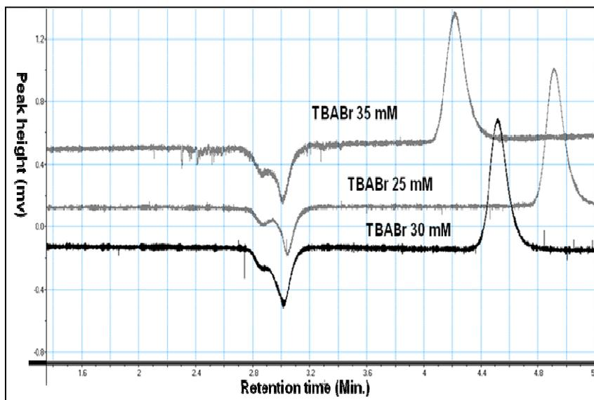
**Figure 3.5** Retention time of  $[\text{Fe(III)EDTA}]^-$  decreases with increasing the concentration of tetrabutylammonium bromide (TBABr) in the mobile phase during chromatographic separation when other parameters remain the same.
