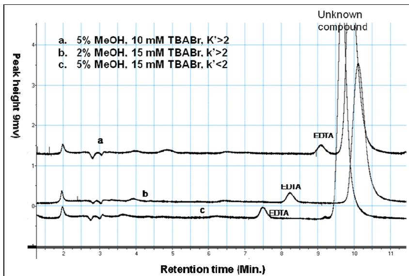
**Figure 3.8** Overlay of chromatograms during chromatographic separations by varying composition of mobile phases to ensure that  $[\text{Fe(III)EDTA}]^-$  is completely separated from other compounds for dairy wastewater samples
