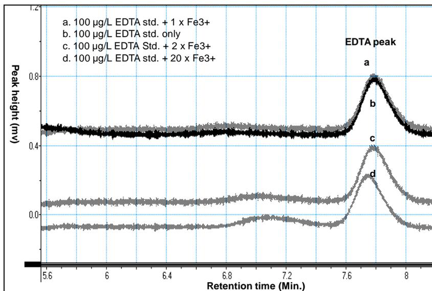
**Figure 3.14** Overlay of EDTA chromatograms to determine the effect of addition of  $\text{Fe}^{3+}$  on HPLC analysis.
