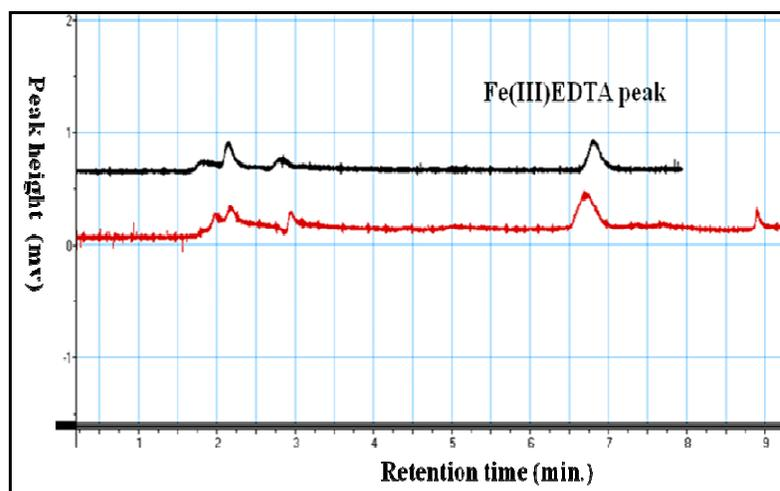
**Figure 7.15** Overlay of HPL-UV chromatograms of a 25 µg/L of EDTA standard (black line) and a groundwater sample with a pre-concentrated factor of 2.5 (red line).
