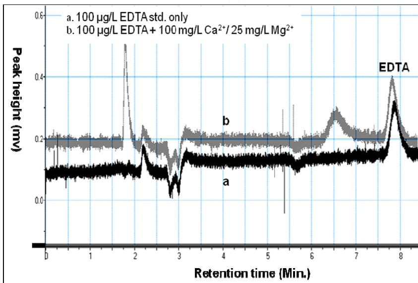
**Figure 3.13** The effect of addition of a mixture of calcium and magnesium (ratio 4:1) on HPLC analysis of EDTA.
