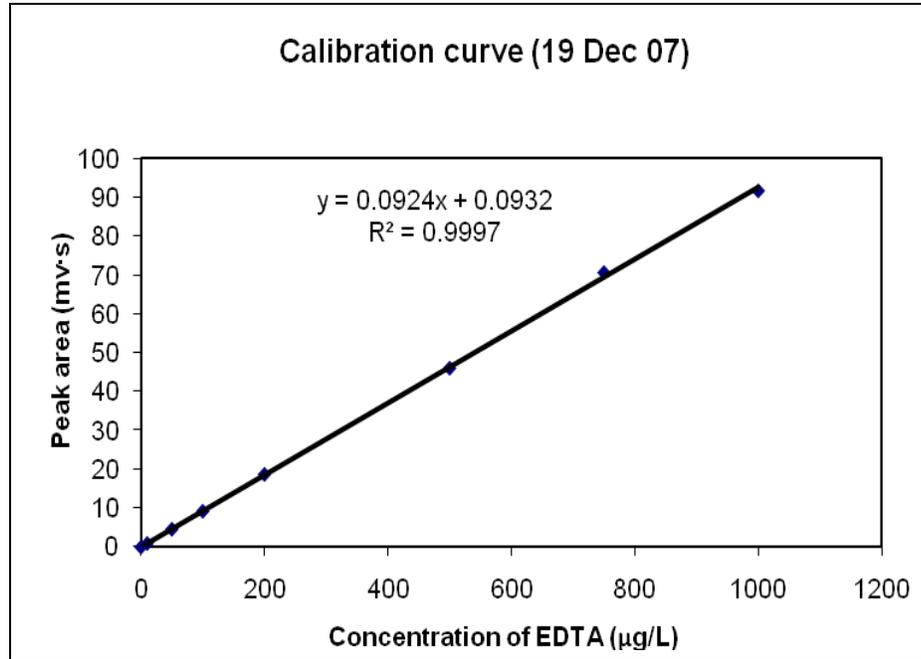
**Figure 4.11** A daily EDTA calibration curve ranging from 0 - 1000  $\mu\text{g/L}$  by HPLC-UV with freshly prepared EDTA solutions.
