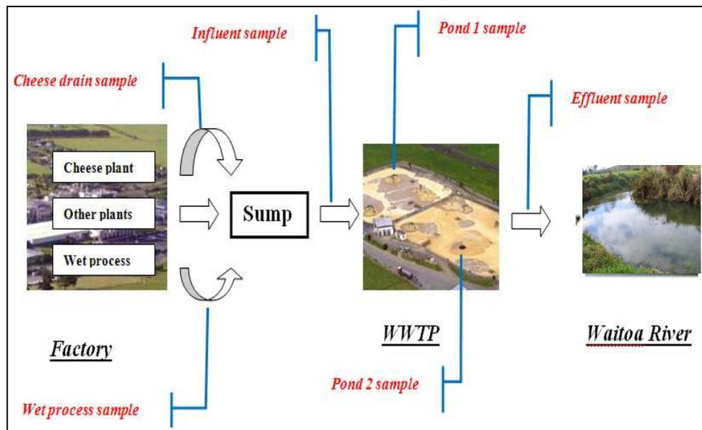
**Figure 4.8** Flow diagram of wastewater and sample collecting sites at the Waitoa dairy site, Fonterra Co-operative Group Limited
