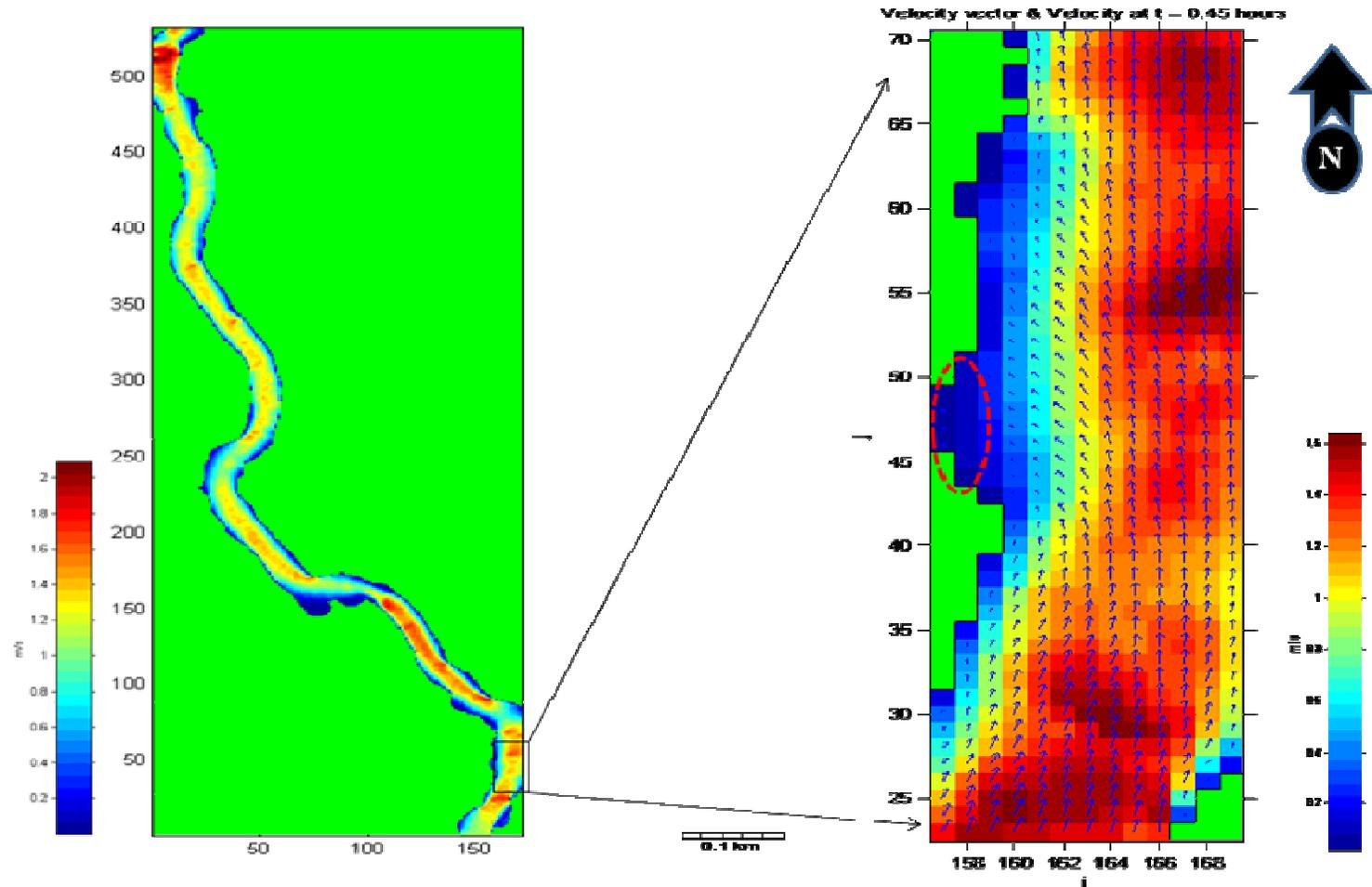
**Figure 6.15** The simulated river flow, velocity vector pattern and velocity using the 3DD hydrodynamic model at a high river velocity of 1.0 m/s for the Waitoa River. The peak velocity can be seen to reach 2.1 m/s in the modelled region, and the velocity of the dead zone caused by an eddy close to the boundary (red dash-circle) can be seen to be much smaller than the domain river velocities.
