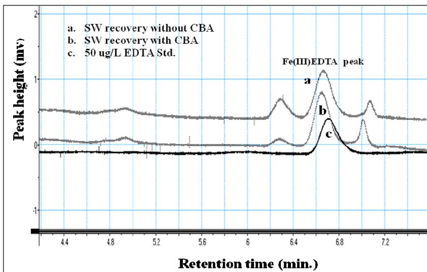
**Figure 5.8** Overlay of chromatograms of the surface water spiked by a 50  $\mu\text{g/L}$  EDTA standard with and without a CBA clean cartridge, compared with a 50  $\mu\text{g/L}$  EDTA standard solution.
