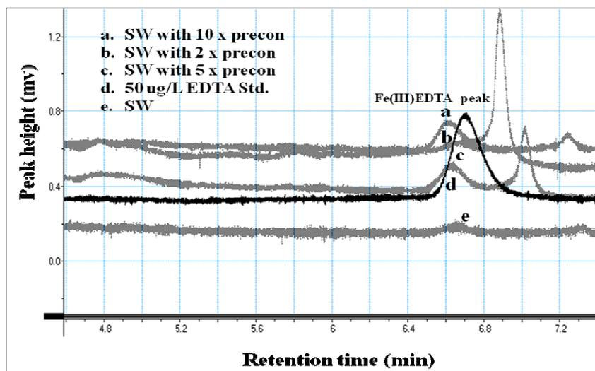
**Figure 5.6** Overlay of chromatograms of surface water (SW) samples with x1, x2, x5 and x10 pre-concentration compared with a 50  $\mu\text{g/L}$  EDTA standard solution.
