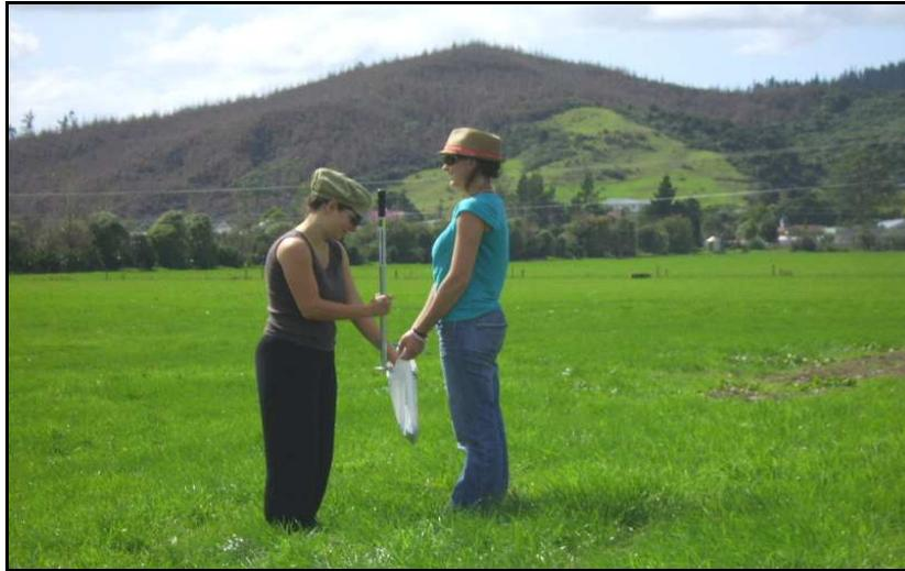
**Figure 7.8** Sample was collected with a 75 mm deep auger and pooled into a plastic bag for a composite pastoral topsoil sample.
