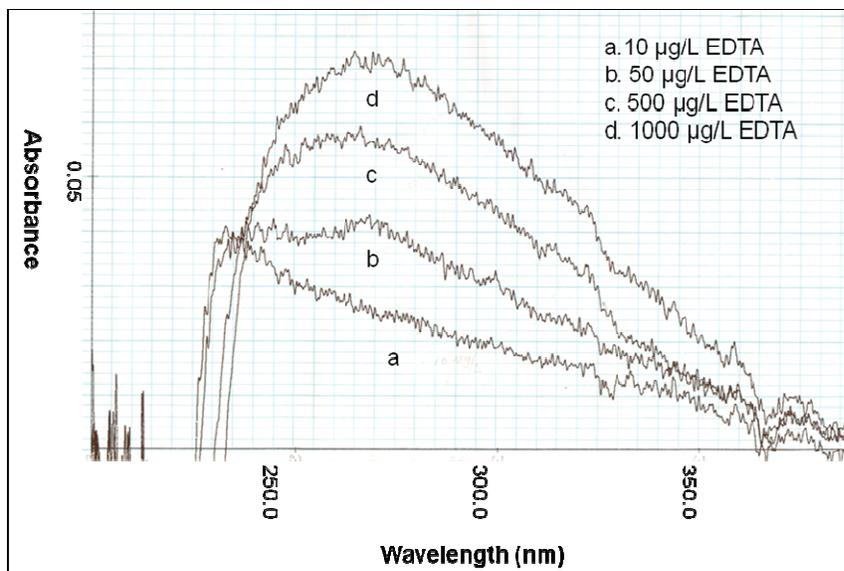
**Figure 3.9** Wavelength scan spectrophotograms of  $[\text{Fe(III)EDTA}]^-$  with different concentrations of EDTA standard solution
