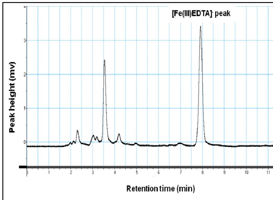
**Figure 4.12** A chromatogram of a typical dairy wastewater sample of influent from the Waitoa dairy site, Fonterra Co-operative Group Limited.
