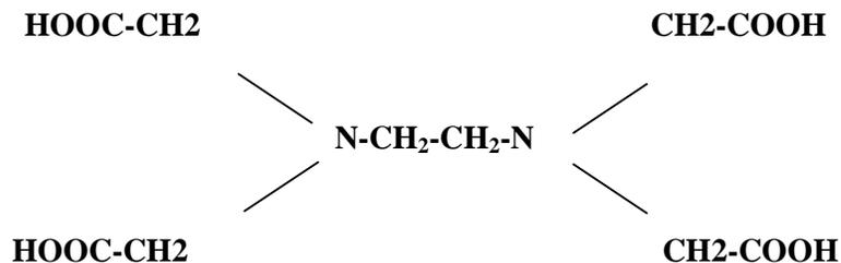
Figure 2.1 Molecular structure of EDTA.
