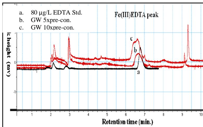
**Figure 7.14** Overlay of HPLC-UV chromatograms of an 80 µg/L EDTA standard (black line) and a groundwater sample with a pre-concentrated factor of 5 and 10 (red lines of b and c respectively).
