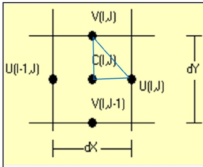
**Figure 6.10** Structure of each model ‘cell’, where  $dX$  and  $dY$  are grid size (m), the x-direction (U velocity) is positive to the east and with corresponding an increasing I, and V velocity is positive to the north and corresponds with an increasing J. Each cell is referenced by its (I, J) coordinate and the U and V velocities in the triangle corresponding to that point.
