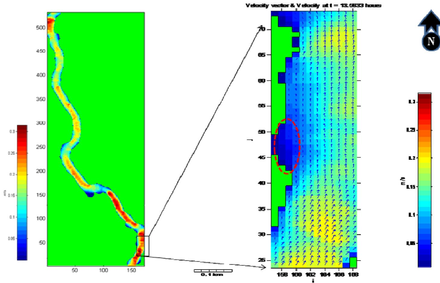
**Figure 6.14** The simulated river flow, velocity vector pattern and velocity by the 3DD hydrodynamic model at a low river velocity of 0.2 m/s (river flow of 425 L/s) in the Waitoa River. The peak velocity can be seen to reach 0.31 m/s in the modelled region, and
