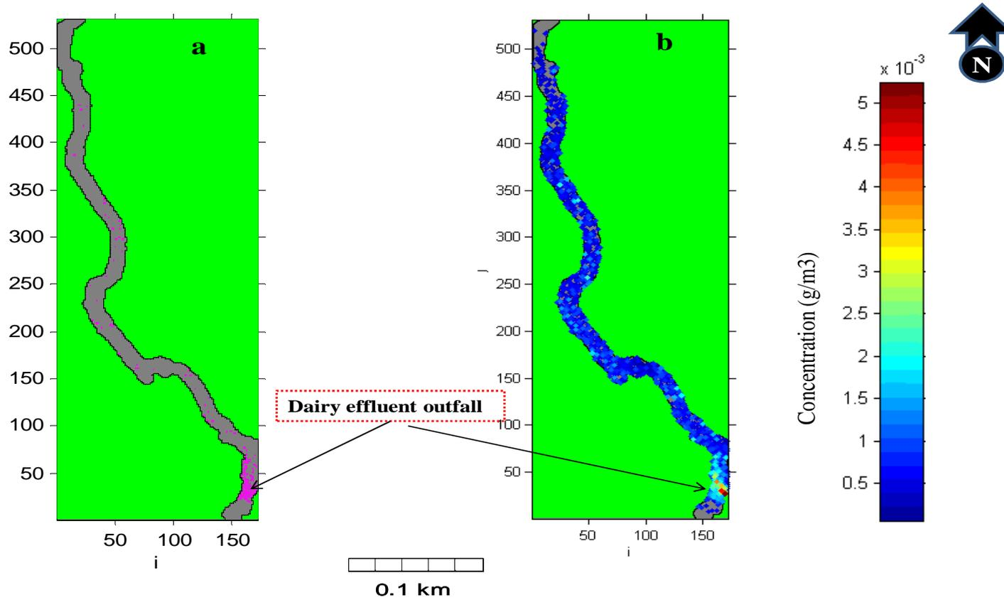
**Figure 6.16** Particle tracking result (a) and simulated EDTA concentrations ( $\text{g/m}^3$ , e.g.  $10^3 \mu\text{g/L}$ ) (b) by the POL3DD model within the Waitoa River for the monitored case, as dairy effluent discharge volume of  $0.055 \text{ m}^3/\text{s}$  at the low river velocity of  $0.2 \text{ m/s}$  (or
