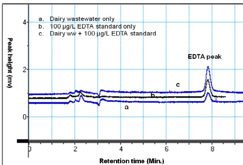
**Figure 3.17** Overlay of chromatograms of a dairy wastewater sample only, 100  $\mu\text{g/L}$  EDTA standard solution and dairy wastewater sample spiked by 100  $\mu\text{g/L}$  EDTA with 101 % EDTA recovery achieved.
