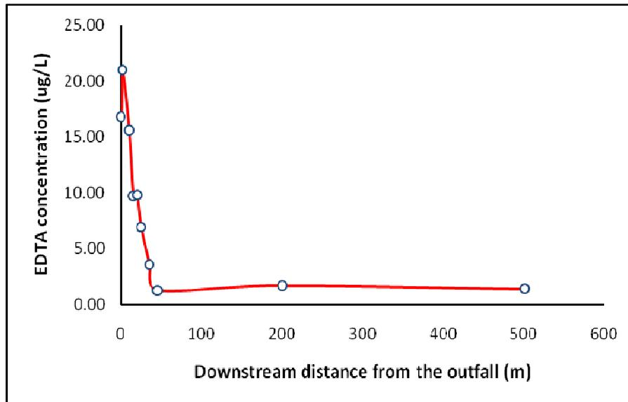
**Figure 6.20** The trend of EDTA concentrations in the Waitoa River, where the Waitoa dairy effluent discharged for the worst case of the year of 2008.
