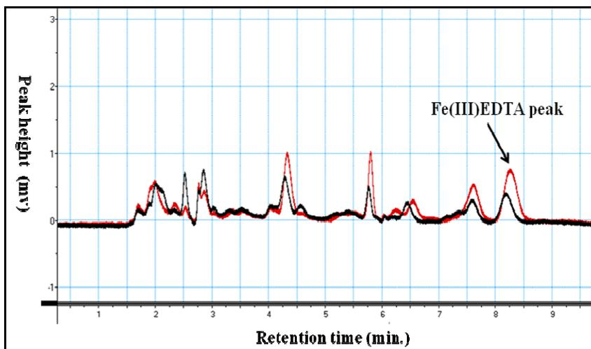
**Figure 7.12** Overlay of HPLC-UV chromatograms of a 100  $\mu\text{g/L}$  EDTA spiked soil sample (red line) and a pastoral topsoil sample only (black line) from the Hikurangi irrigated farm with dairy wastewater from the Fonterra Kauri site.
