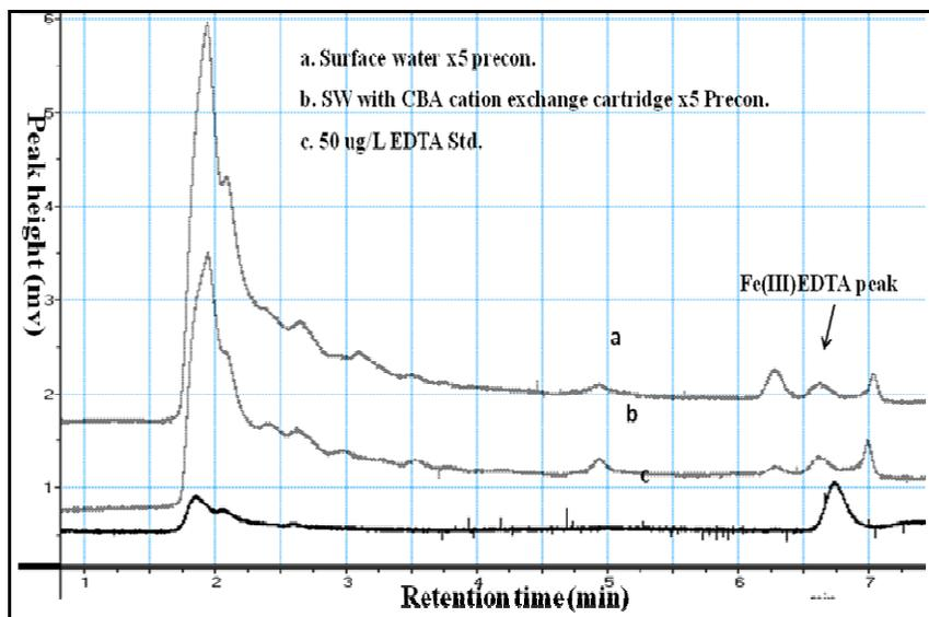
**Figure 5.7** Overlay of chromatograms of the surface water sample with and without a CBA SPE clean cartridges, compared with a 50  $\mu\text{g/L}$  EDTA standard solution.
