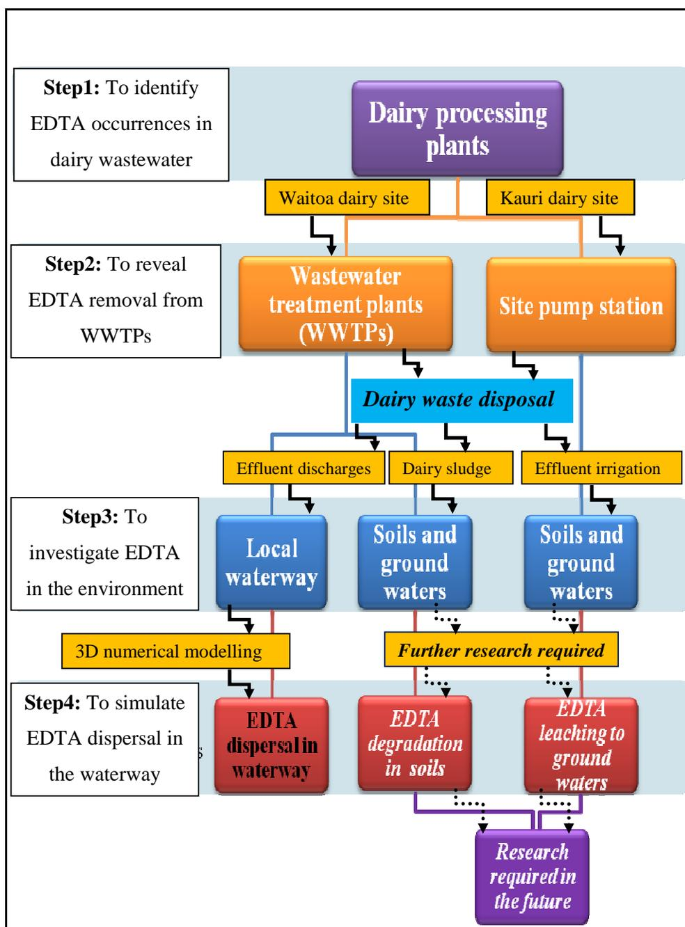
**Figure 1.5** The research approach includes four major steps to (i) identify EDTA occurrences in drainage of dairy processing plants, (ii) ascertain EDTA removal efficiency from wastewater treatment plants, (iii) investigate EDTA presence in the natural environment, and (iv) forecast EDTA potential environmental effects on waterways subsequent to the dairy wastewater discharge.
