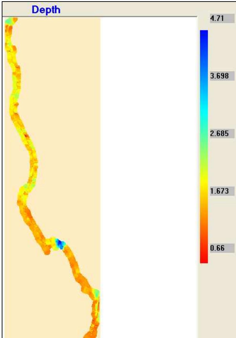
**Figure 6.11** Coverage of KNUDSEN MP 329 Dual Frequency Echo-sounder in the Waitoa River. Survey was undertaken on 15 October, 2008, river flow and height were 3460 L/s and 13.6 m (sea level), respectively.
