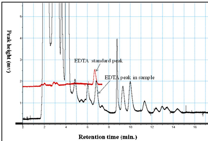
**Figure 7.16** Overlay of chromatograms of a 100 µg/L EDTA standard solution (red line) and a dairy sludge sample (black line) from the Waitoa dairy wastewater treatment plant.
