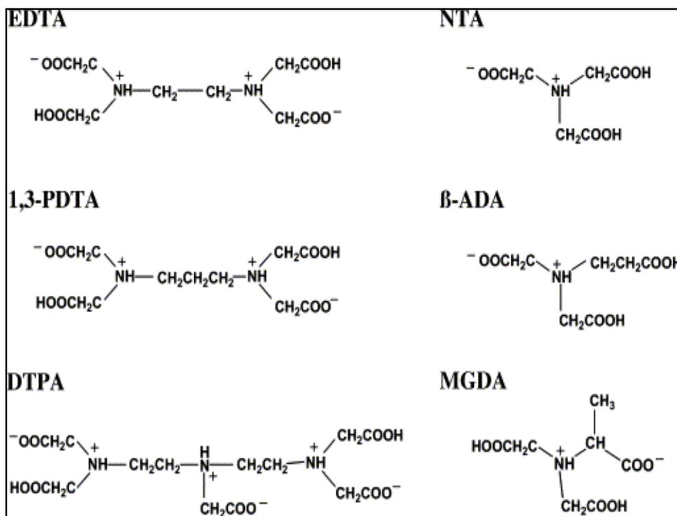
**Figure 2.2** Structural formulae of important aminopolycarboxylates EDTA = EthyleneDiamineTetraacetic Acid, NTA = NitriloTriacetatic Acid, 1,3 – PDTA = 1,3 – PropyleneDiamineTetraacetic Acid, β – ADA = β – AlanineDiacetic Acid, MGDA = MethyGlycineDiacetic Acid DTPA = DiethyleneTriaminePentaacetic Acid
