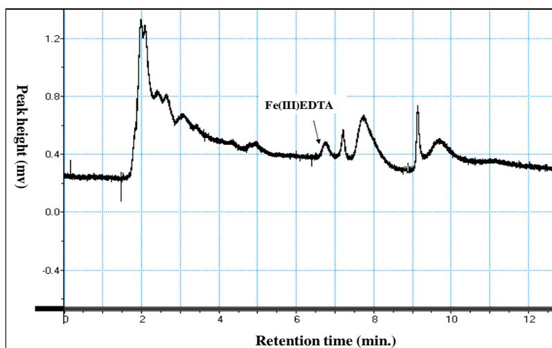
**Figure 5.9** Chromatogram of a typical surface water sample from the Waitoa River.
