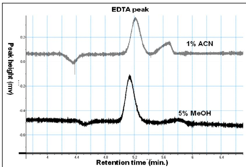
**Figure 3.3** A similar  $[\text{Fe(III)EDTA}]^-$  retention time obtained using a lower percentage of ACN (1%) than MeOH (5%) during chromatographic separation when other parameters remain the same.
