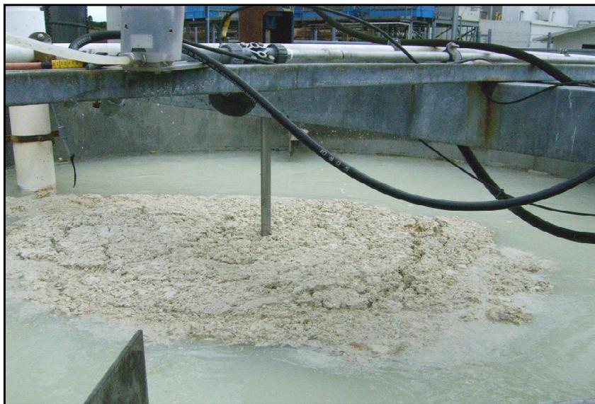
**Figure 7.4** Wastewater pre-treatment by the dissolved air flotation (DAF) process prior to the land spray irrigation at the Fonterra Kauri dairy site.
