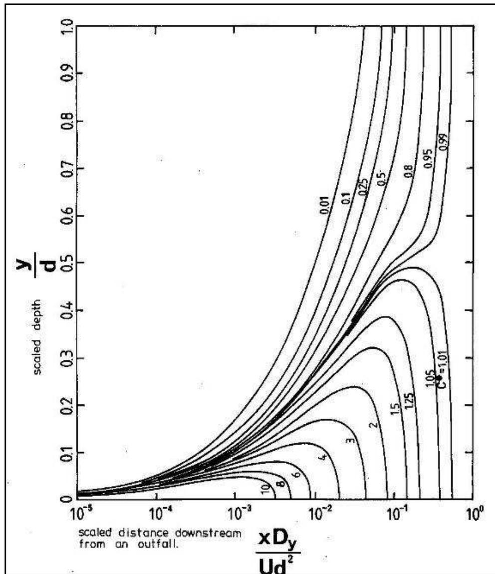
**Figure 6.5** Concentration contours downstream from a steady transverse line source, applicable to the Waitoa dairy wastewater discharge, located on the channel bed of the Waitoa River.
