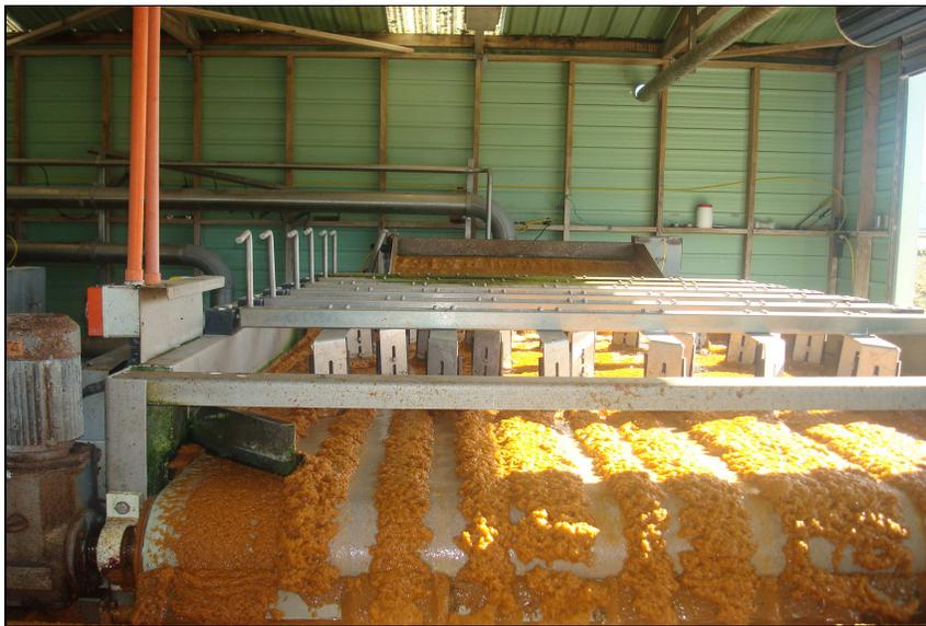
**Figure 4.7** Gravity belts operate to thicken the sludge before being trucked away and spread onto nearby pasture land at the Waitoa dairy wastewater treatment plant.
