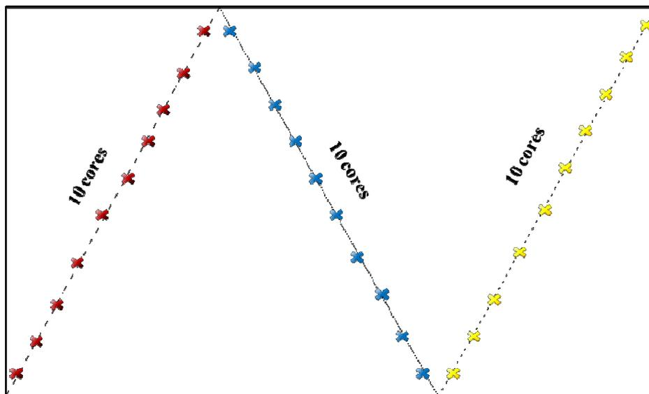
**Figure 7.7** A pattern of approximately 10 cores (1.5 m apart) per arm of a 0-75 mm deep 'z' shape of across to give a total of 30 cores were taken and pooled to produce one composite pastoral topsoil sample.
