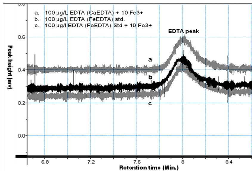
**Figure 3.16** Overlay of chromatograms of 100 µg/L EDTA from independent solutions of standard EDTA as  $[\text{Fe}(\text{III})\text{EDTA}]^{-}$ , converted  $[\text{Ca}(\text{II})\text{EDTA}]^{2-}$  and pre-treated standard as  $[\text{Fe}(\text{III})\text{EDTA}]^{-}$ .
