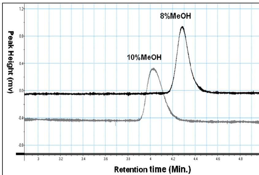
**Figure 3.4** High composition of solvents shortened the  $[\text{Fe(III)EDTA}]^-$  retention time during chromatographic separation when other parameters remain the same.
