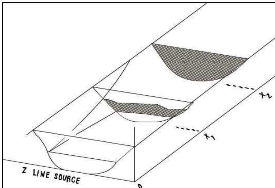
**Figure 6.4** Diagram of quasi one-dimensional vertical mixing of EDTA from a steady uniform transverse line source, as for example from the Fonterra Waitoa dairy wastewater into the Waitoa River.
