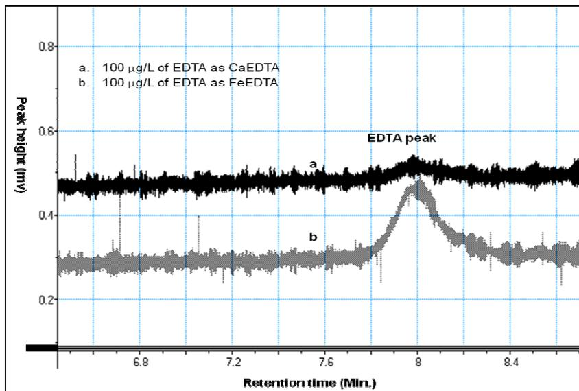
**Figure 3.15** Absorbance comparison of 100 µg/L EDTA as  $[\text{Fe}(\text{III})\text{EDTA}]^{-}$  and  $[\text{Ca}(\text{II})\text{EDTA}]^{2-}$ .
