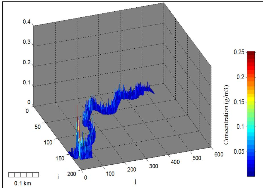
**Figure 6.18** The simulated EDTA concentrations by the POL3DD model illustrated in three dimensions within the Waitoa River for the worst scenario of high volume discharge ( $0.081 \text{ m}^3/\text{s}$ ) and low river flow ( $425 \text{ L/s}$ ). It can be seen that the instantaneous EDTA concentration reached  $0.25 \text{ g/m}^3$  at the immediate vicinity of the dairy effluent outfall.
