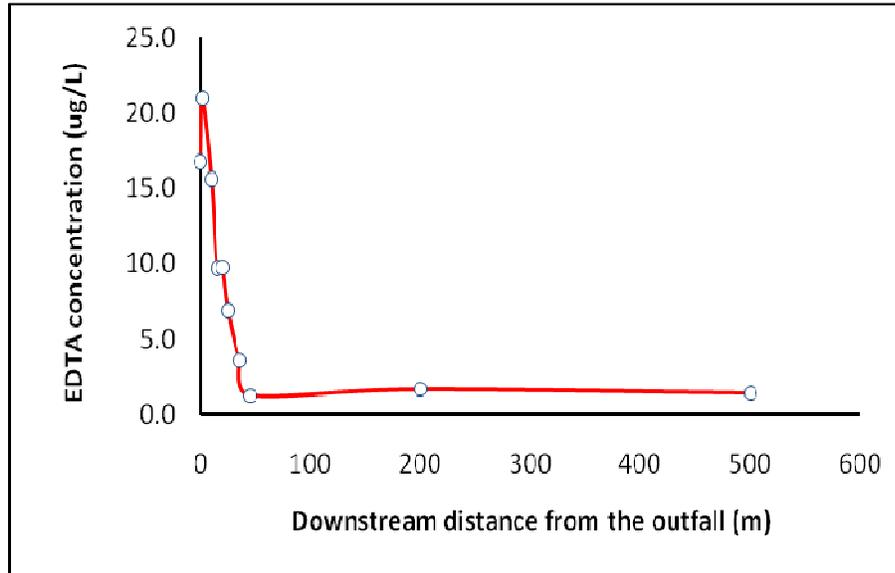
**Figure 6.19** The trend of EDTA concentrations in the Waitoa River, where the Waitoa dairy effluent discharged for the monitored case of 30 May 2008.
