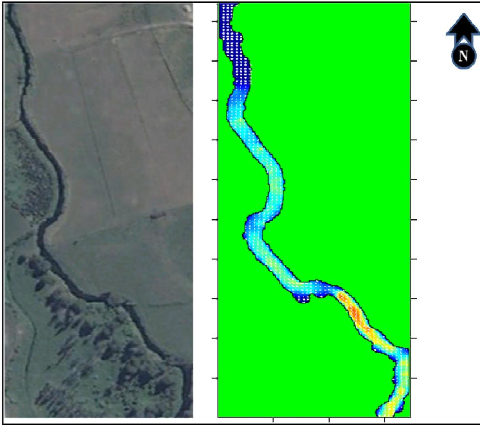
**Figure 6.12** A comparison of the created bathymetry for the 3DD hydrodynamic model with the aerial photo of the investigated region in the Waitoa River from the Google Earth.
