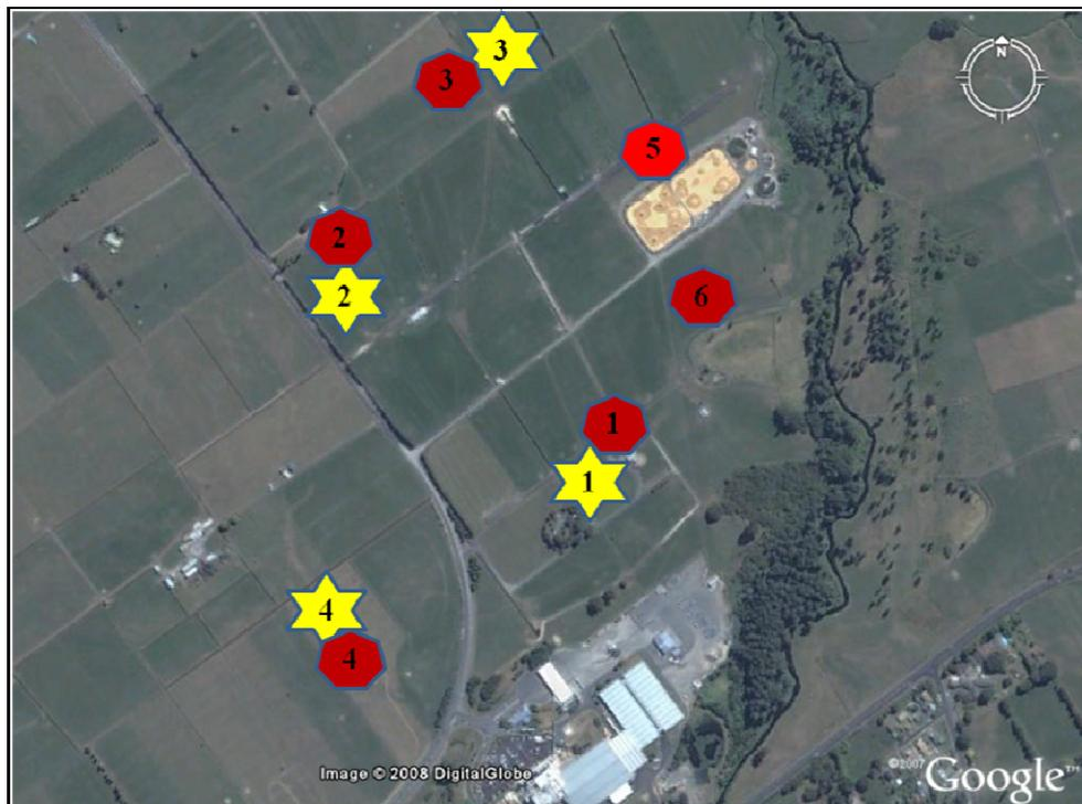
**Figure 7.9** Layout of paddocks for soil sample collection and groundwater wells near the Fonterra Waitoa dairy site, where paddock 4 was a reference site as no dairy biomass had been applied, and paddock 5 was the heaviest dairy biomass spread paddock.
