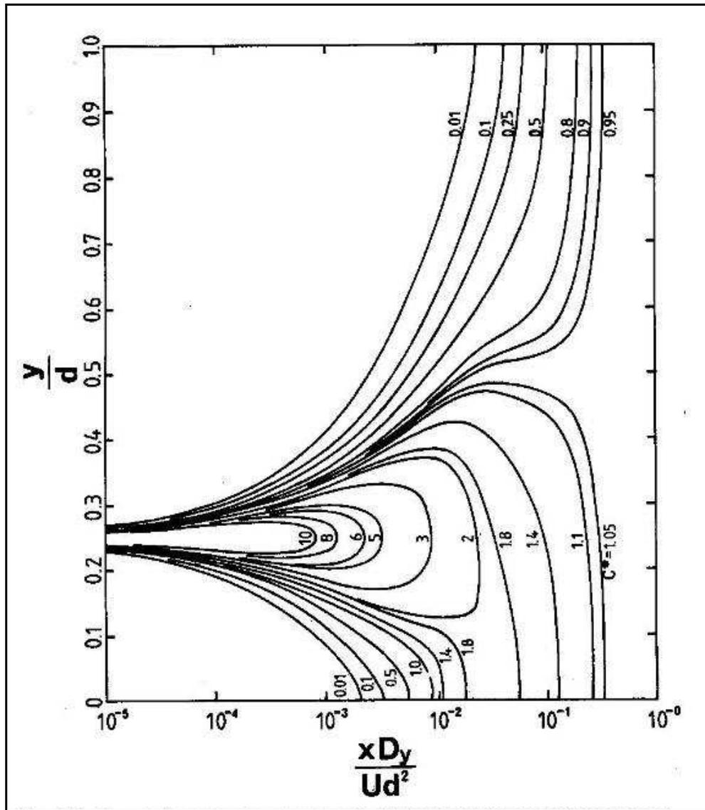
**Figure 6.6** Concentration contours downstream from a steady transverse line source, applicable to the Waitoa dairy wastewater discharge, located at three-quarters depth of the river channel of the Waitoa River.
