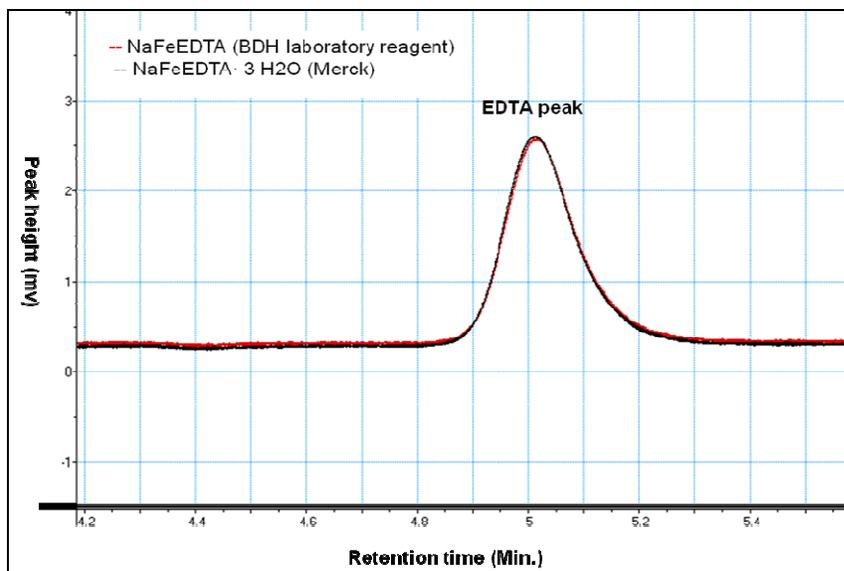
**Figure 3.18** Overlay of chromatograms at the concentration of 1 mg/L EDTA as NaFeEDTA manufactured by different companies.
