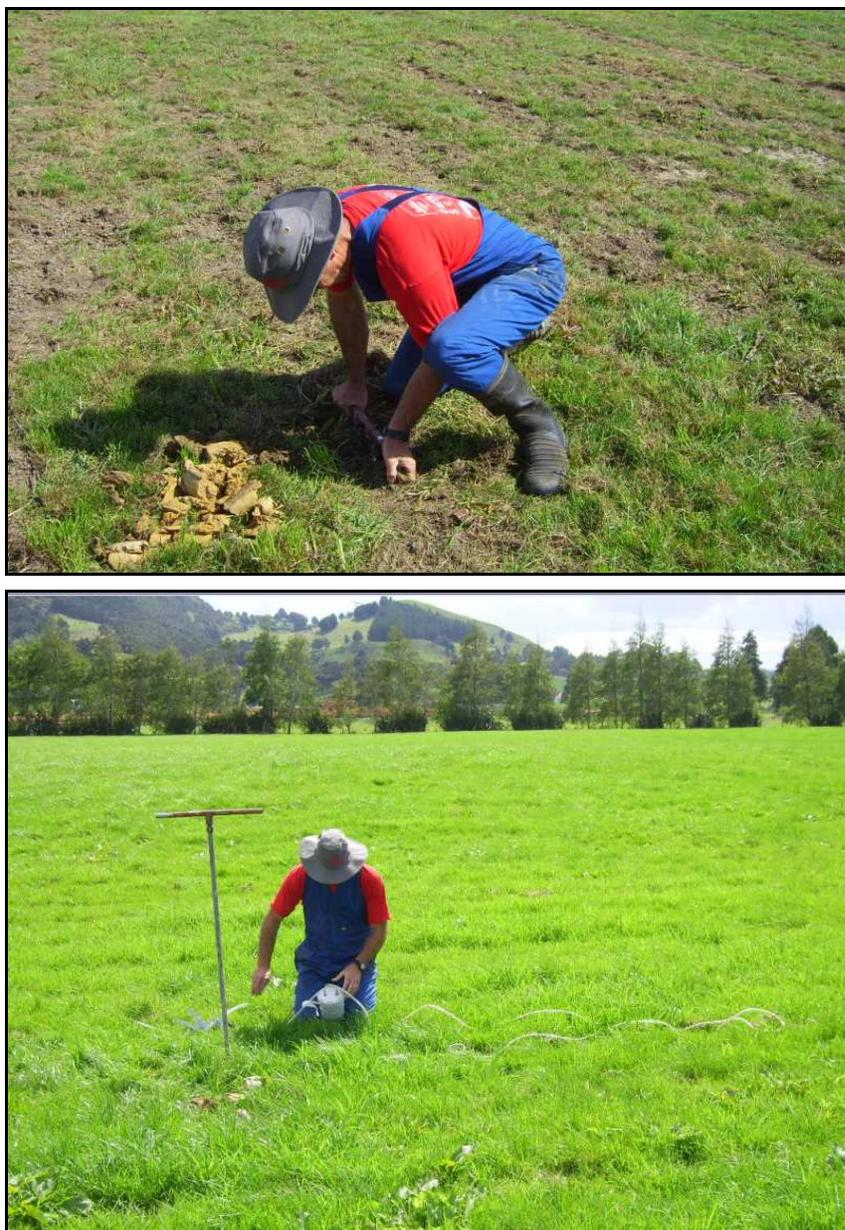
**Figure 7.13** Groundwater sample was collected at both the Hikurangi and Kauri farms near the Fonterra Kauri dairy site by digging a hole to reach the groundwater and drawing it through a plastic tube to a container.
