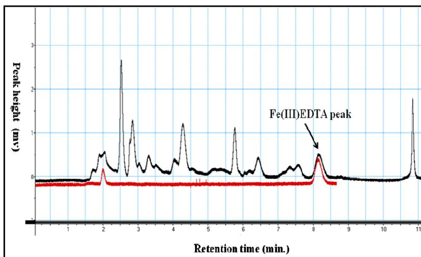
**Figure 7.11** Overlay of chromatograms of an 80 µg/L EDTA standard (red line) and a pastoral topsoil sample (black line) from the Hikurangi irrigated farm with dairy wastewater from the Fonterra Kauri site.
