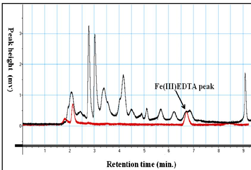
**Figure 7.10** Overlay of chromatograms of a 50 µg/L EDTA standard (red line) and a pastoral topsoil sample (black line) from the Hikurangi irrigated farm with dairy wastewater from the Fonterra Kauri site.
