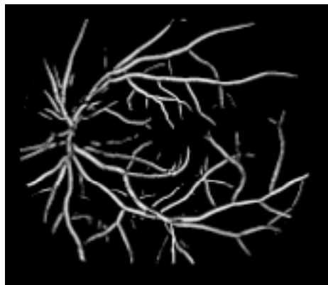
Figure 4. The same image after adaptive thresholding on the probability of each pixel being part of a vessel.
