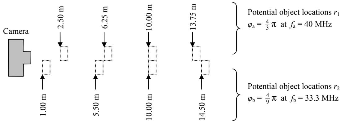
Figure 2: A single object produces multiple ambiguous range values for a single modulation frequency. By comparing two different modulation frequencies, the true object location (10.00 m) can be resolved.
