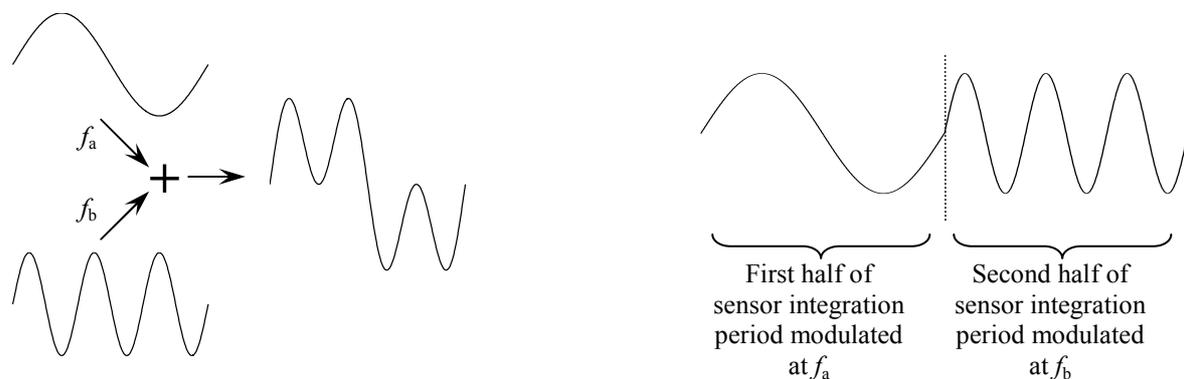
Figure 3: Left: Two sinusoidal waveforms at frequencies  $f_a$  and  $f_b$  are superposed to create the sensor and light source modulation waveform. Right: The same effect can be created by dividing the sensor integration period in two, and switching between  $f_a$  and  $f_b$  for each captured image.
