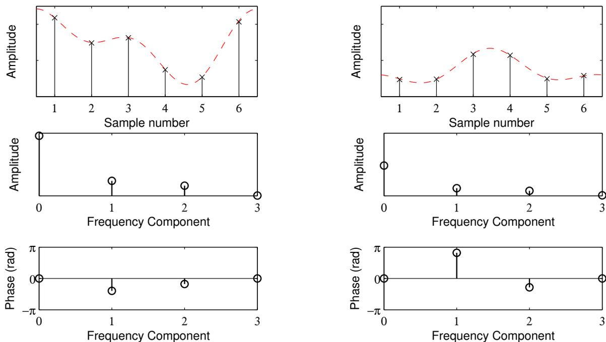
Figure 5: Top: Raw captured data for a single pixel located at object 2 (left) and object 4 (right). The dashed line illustrates the reconstructed received illumination waveform. Centre and bottom: Amplitude and phase calculated using a DFT on the six samples.
