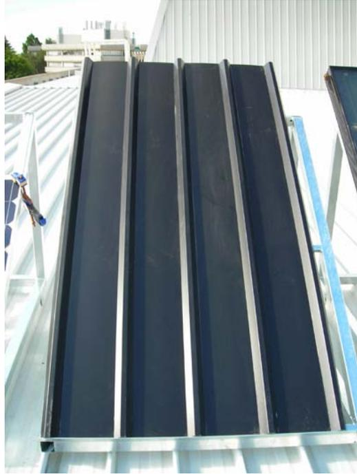
Fig. 3 Prototype building integrated solar collector
