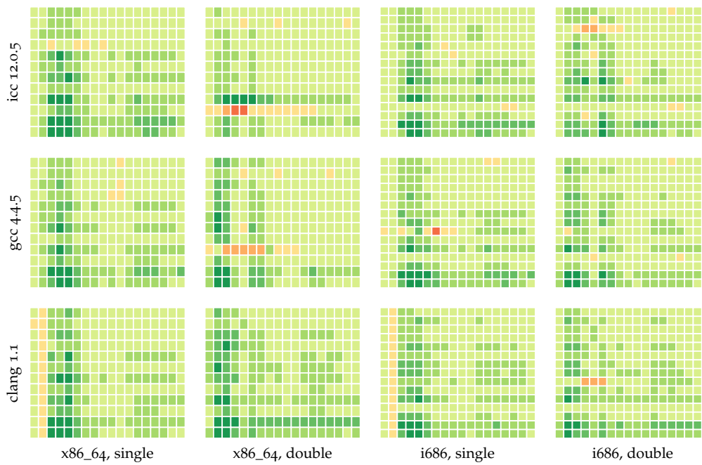
Figure 15: Performance comparison between SFFT and FFTW 3.3 in estimate mode on SSE machines
