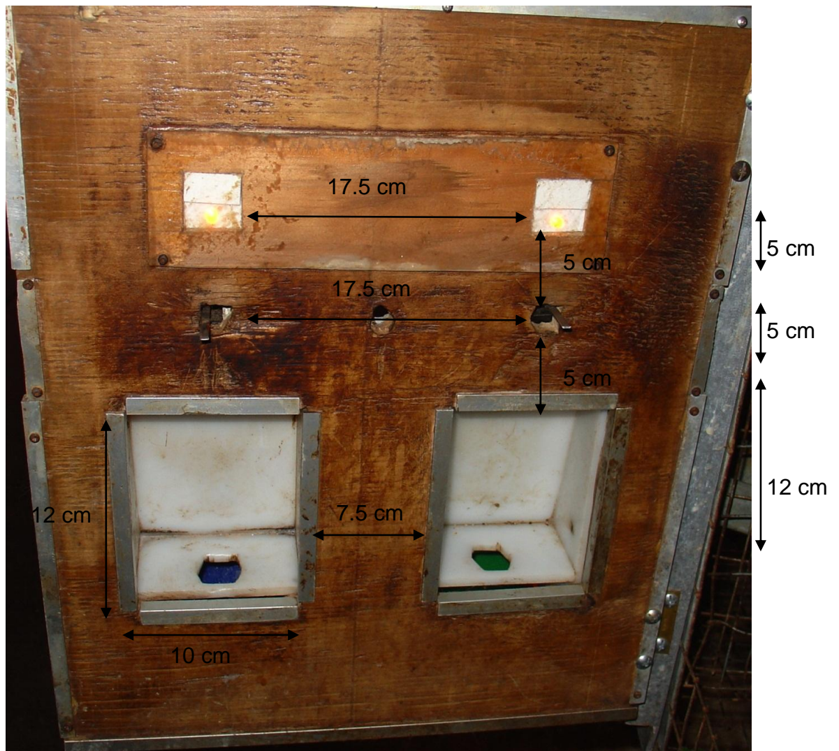
Figure 9. Photo of the response panel for Caper, Peppi, Screech and Norrin showing the positions of the lights, response levers and magazine openings.
