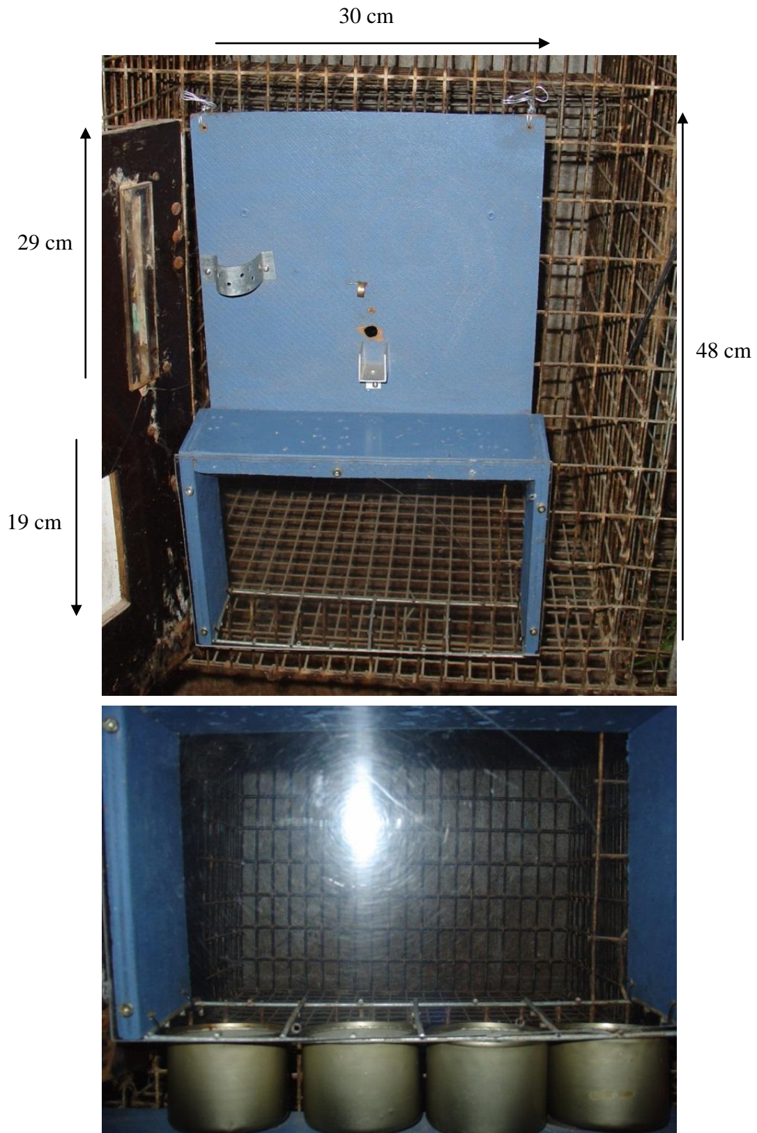
Figure 2. The preference apparatus. The top panel shows the panel attached to a possum's home cage, and the bottom panel shows four tins raised up to the apparatus, as in the multiple-stimulus without-replacement (MSWO) assessment.
