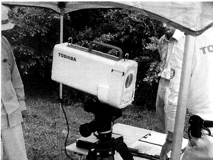
*Fig. 1. The Toshiba "Gamma Camera" (under shade cover because of hot, bright sunny weather). (Lowe)*
