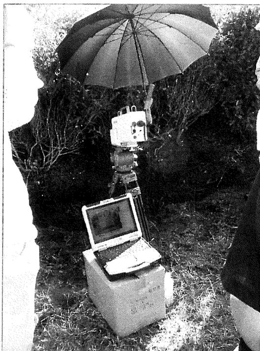
The intensity and direction of gamma rays are displayed in the form of colour-coded pixels superimposed on the target image, ranging from blue (low) through greens and yellows to red (high) levels (Fig. 3). Portable shielding in the form of multiple sheets, each containing 10 kg of lead, can be hung on frames around, and placed beneath, the camera to help reduce background levels even further, both in the field and in the laboratory (Figs. 4 and 5). The camera has fixed a 60-degree view angle.
