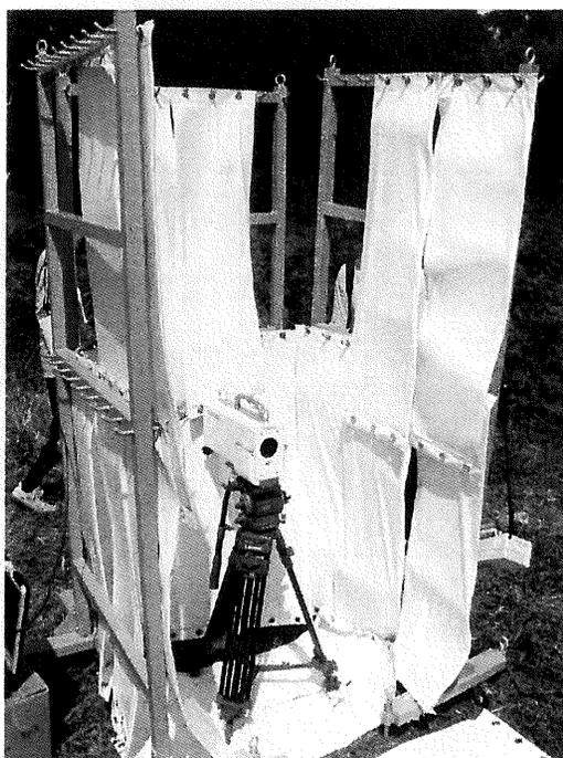
*Fig 4. Lead shielding being placed under and around the gamma camera in the field to help reduce natural background radiation levels so that the camera is more efficacious. (Lowe)*
