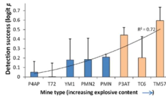
Figure 3. Mean detection success (logit *p*) calculated across trials for each mine type. Anti-personnel mines are shown in blue, and anti-tank mines in orange. A polynomial curve was fitted to the data, and error bars represent the mean's standard error.
