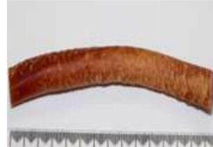
Extrudate flowed well out of extruder with moderate pressures and torque. Extrudate was flexible and rubbery and its surface was reasonably smooth. Some surface defects such as small cracks, powder and shark skinning were present.
