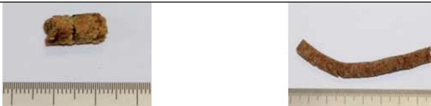
There was no melt formation and extrudate exited the extruder as powder or small sections of compressed powder. The sections of compressed powder had high amounts of surface defects and broke apart easily if bent or compressed.
