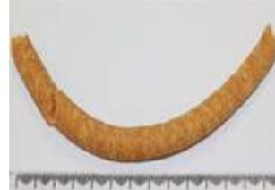
Extrudate flowed well out of the extruder with moderate pressures and torque. Extrudate was flexible and rubbery but had large sections with defects such as voids, cracks, compressed powder sections and shark skinning. They also broke easily when bent or compressed.
