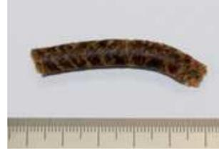
No melt formation and extrudate flowed poorly out of the extruder causing high pressures and torque. Extrudate was not flexible or rubbery and broke when bent. Surface defects such as voids, cracks and shark skinning were also present.
