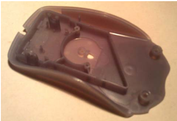
Figure 3: Base of a standard MS Optical Mouse (front at left).
