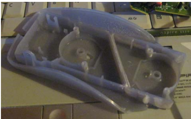
Figure 4: A second detector frame glued onto the rear of the first mouse.
