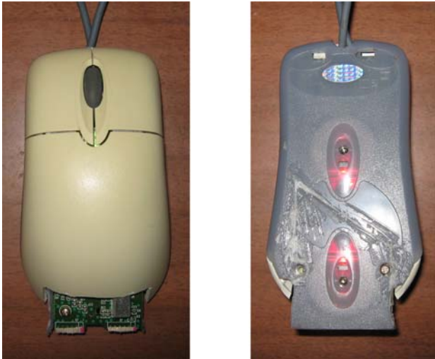
Figure 1: Top and bottom views of the prototype Orienting Mouse showing dual optical sensor.
