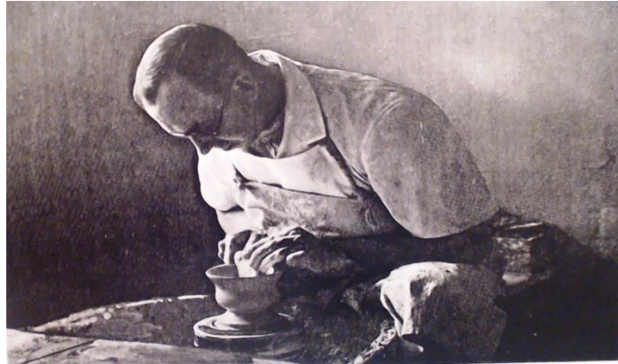
Figure 8: The revolving wheel on which the clay takes the form under the pressure of the thrower's skilful fingers (Shelly, 1937)
