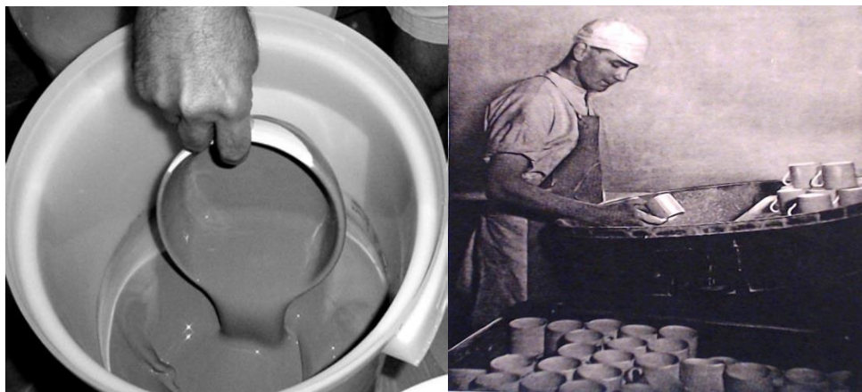
Figure 9: The Dipper applying Glazes , The liquid glaze used is borax- flint –lead glass (Retrieved from (Lehman, 2002; Shelly, 1937)
