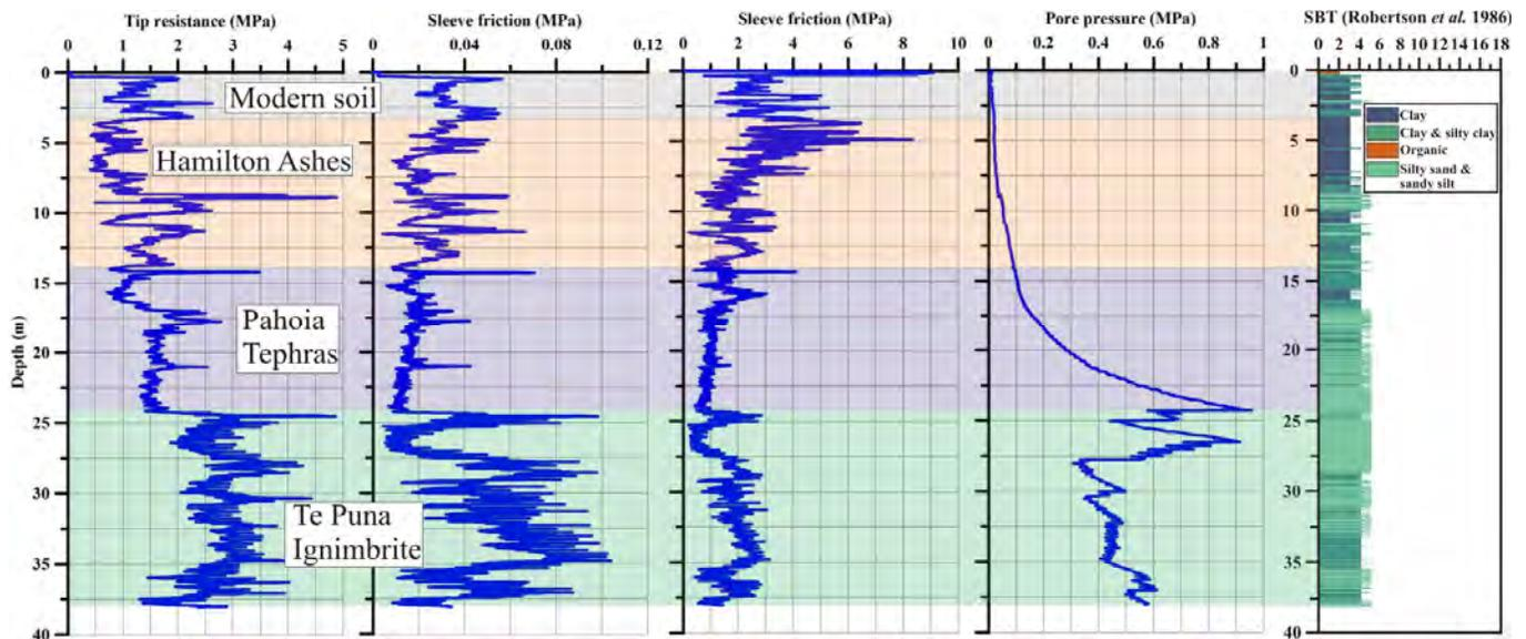
Figure 6. CPTu and soil behavior type results from the Omokoroa landslide. Tip resistance and pore pressure are after Moon *et al.* (2013).
