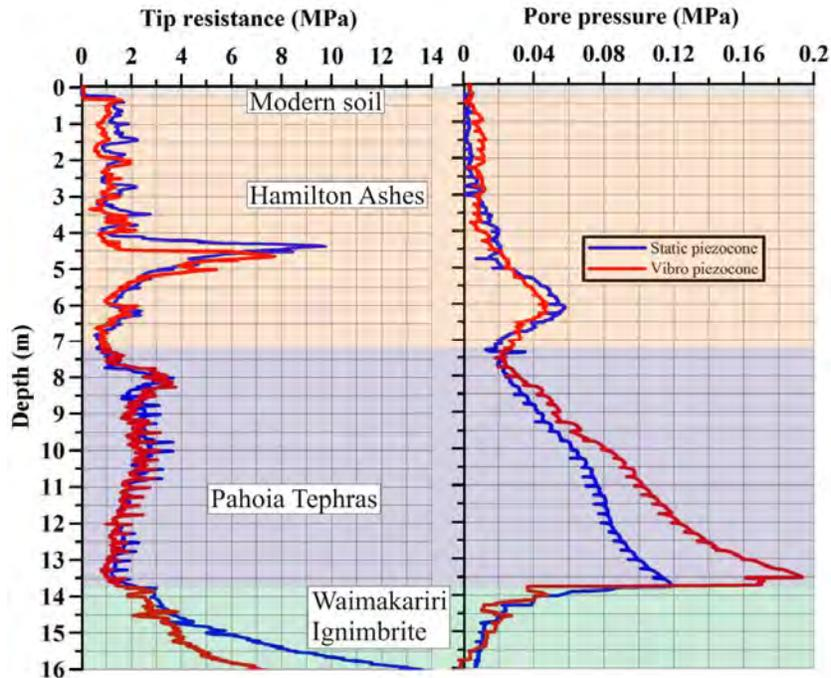
Figure 5. Comparisons of static and vibratory CPTu test results (after Jorat *et al.* 2014).
