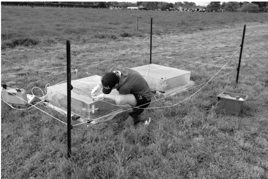
Appendix 2d Chamber set up with two Perspex chamber used in experiment two. Two Perspex chambers and four additional chambers construct with a frame and plastic sheeting were used during experiment three.
