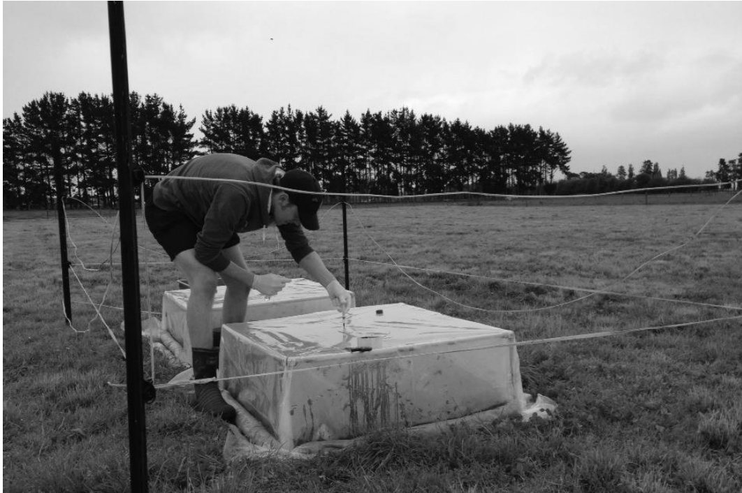
Appendix 2c Chamber set-up following installation of plastic sheeting over framing and injection of acid to evolve CO 2 . Sandbags were placed around base of plastic sheeting to seal to ground.
