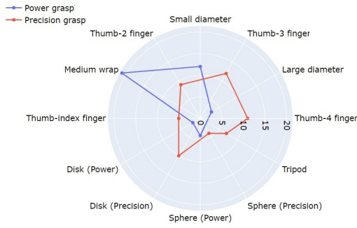
Fig. 3. Occurrence of each grasp type. The radar plot shows the number of times each grasp type is employed to grasp the objects during the experiments. Power grasps are mostly employed when the user requires a grasp that provides more security and stability, whereas precision grasps are employed when an emphasis on dexterity and sensibility is needed.
