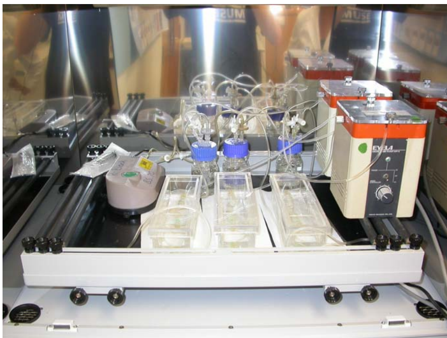
Figure 3.2. Ex vivo perfusion model: Three chambers are set up running along side each other, peristaltic pump( Eyela Microtube Pump MP-3) producing a flow rate through the umbilical vein of 3\text{ml}\cdot\text{min}^{-1} , dissolved gas content was maintained by pumping air into reservoir through a syringe filter (Millex-HV 0.45\mu\text{m} Filter Unit,SLHV025LS).
