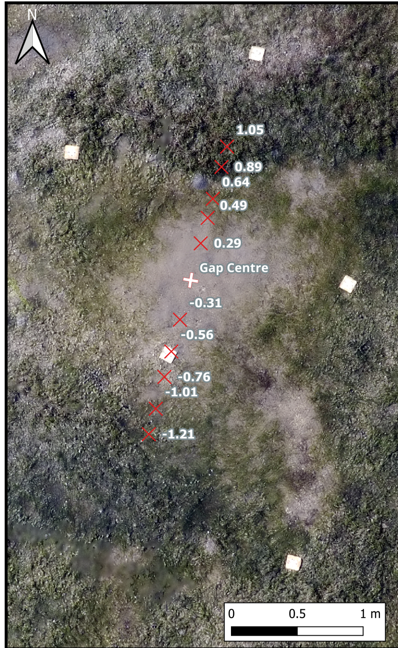
Figure C.1: Locations of the dynamic measurements within and around the gap. The instrument at the Gap Centre was kept in a fixed location throughout. The outer instruments, ('seagrass', positive coordinates and 'gap Edge', negative coordinates) were moved during the several tides. Data was captured over windows of 10-20 min at each location. The coordinates are expressed in meters.
