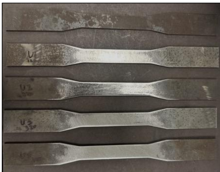
Figure 3.2 - Gradual Sanding to P800, top to bottom
