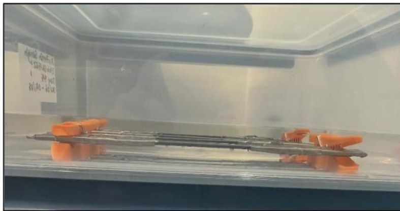
Figure 3.5 – Side view of the testing coupons depicting that the gauge section is lifted off the container to ensure corrosion occurred on all unwrapped exposed surfaces.
