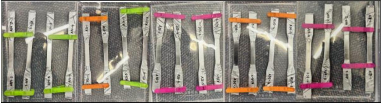
Figure 3.4 – Preparation of 4 nos. of steel coupons for testing at Day 14 to 42 at 7-day intervals for immersion corrosion of the samples.
