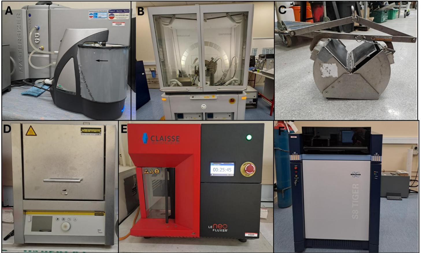
Figure 9. Machinery and equipment used to collect and analyse data. A. Mastersizer 2000 particle sizer used for grain size analysis. B. Panalytical Empyrean Series 2 XRD used in XRD analysis. C. Ponar grab sampler used for sediment sampling the FMTZ of the Waihou River. D. Furnace used for loss on ignition analysis. E. The Neo Fluxer Furnace used to create the fusion beads for XRF major element analysis. F. Bruker S8 Tiger used in XRF major and trace element analysis.
