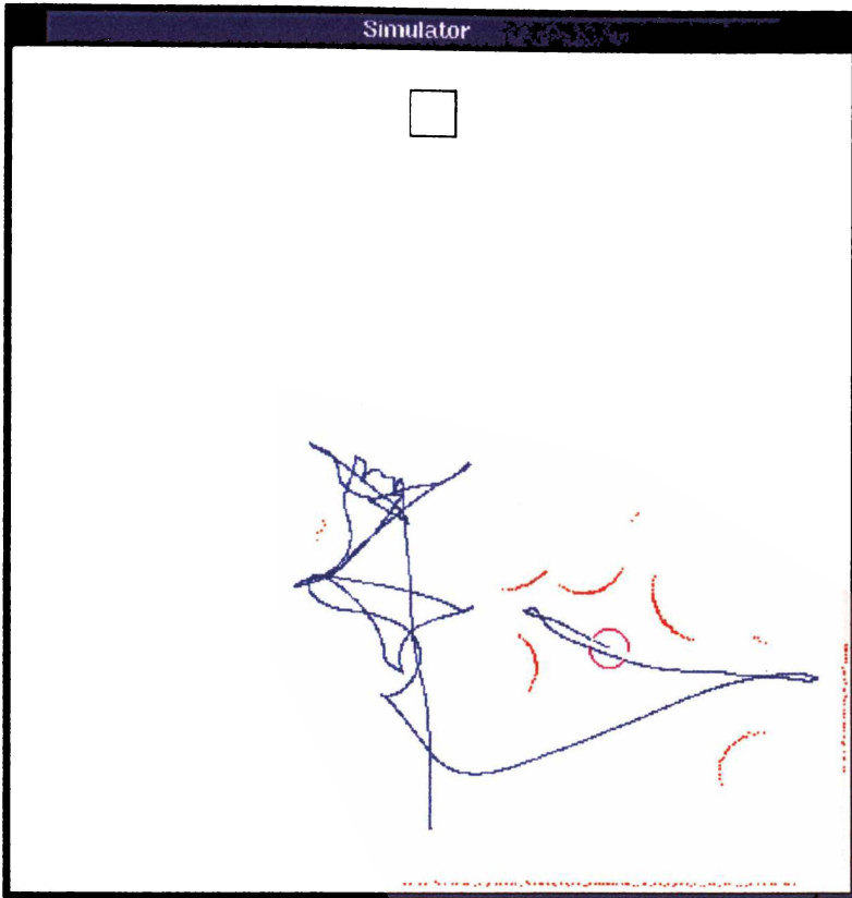
Figure 6-19 The position and trajectory of the AMR after seventy seconds of exploring in World No. 135, Obstacle density 15%.
