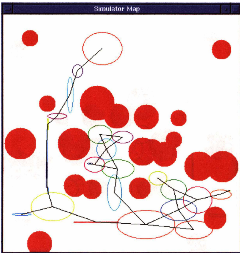
Figure 6-30 The topological map generated by the AMR after 110.9 seconds of exploring in World No. 135, Obstacle density 15%.
