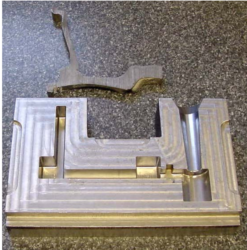
Figure 3-6: One half of the casting mould with the section of alloy wheel its design was based upon.
