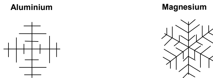
Figure 6-4: Schematic illustration of the different dendritic structure of an aluminium (left) and magnesium (right) alloy casting. The finer dendritic network of the magnesium alloy casting makes interdendritic feeding more difficult.
