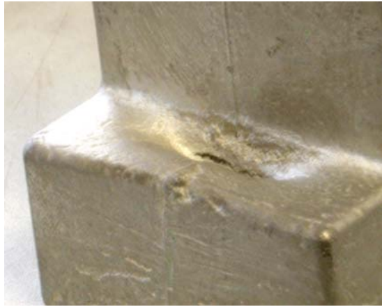
Figure 10-2: Example of a grade 2 surface slumping defect.
