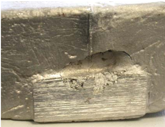
Figure 10-3: Example of a grade 3 externally visible shrinkage porosity defect.
