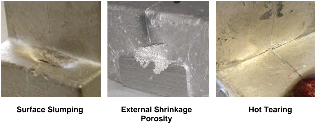
Figure 3-9: Examples of the three types of externally visible casting defects experienced during the experimental casting trials.
