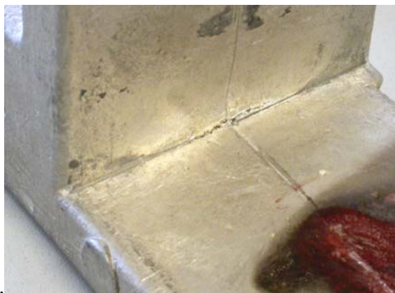
Figure 10-4: Example of a grade 1 hot tearing defect.
