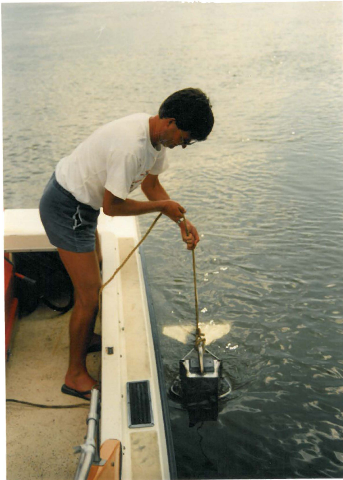
Figure 4.3 : Deployment of bedload traps. A - using a gauging crane off a bridge , B - by hand from the side of the boat.
