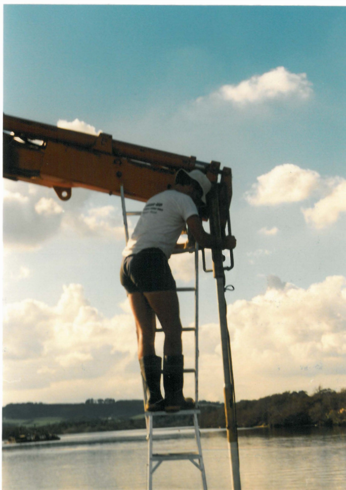
Figure 5.2 : Driving the core tubing into the river bed.
