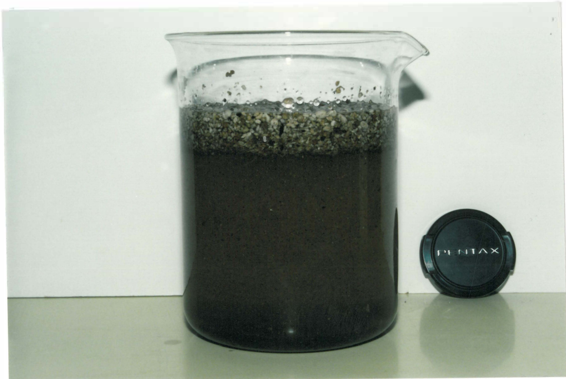
Figure 5.5B : Pumice (light aggregate) settles at the surface after standing for 20 minutes.
