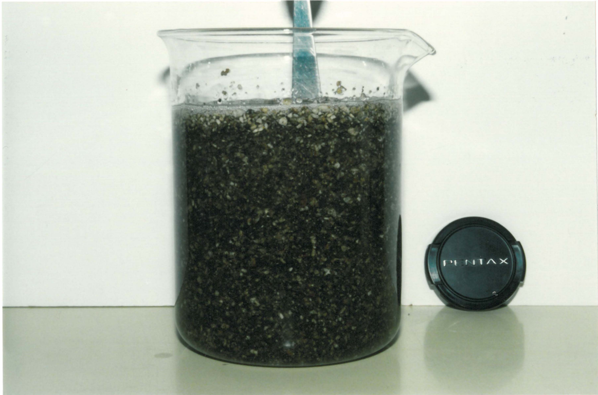
Figure 5.5A : Stirring sand sample vigorously into the \text{ZnCl}_2 solution.
