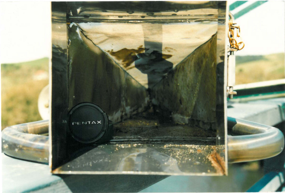
Figure 4.4 : Algae clogged mesh in the bedload trap. During summer low flow algae severely limited the efficiency of the traps.
