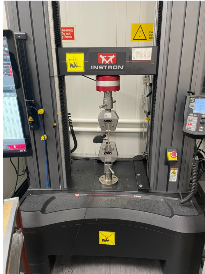
Figure 3.13: The Instron 5982 universal testing machine for destructive tensile testing, detailing the 50 mm gauge extensometer affixed test coupon for strain monitoring.
