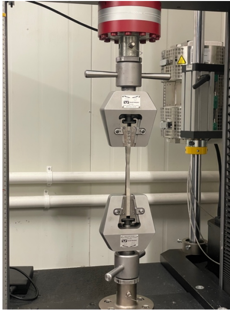
Figure 3.14: The tensile apparatus applying terminal plastic strain to the steel coupon prior to ultimate fracture.
