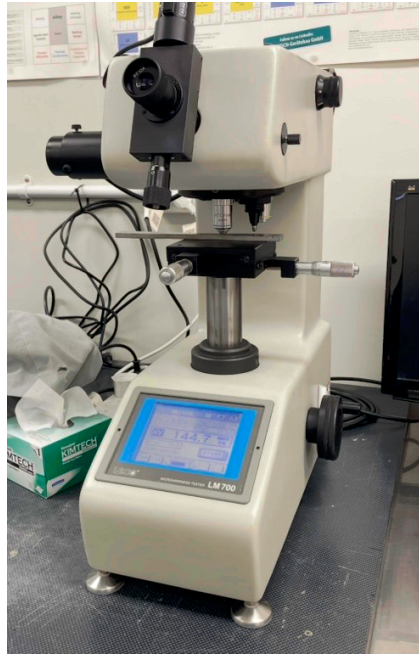
Figure 3.10: The LECO LM700 machine for Vickers (HV1), demonstrating the testing of one of the coupons.
