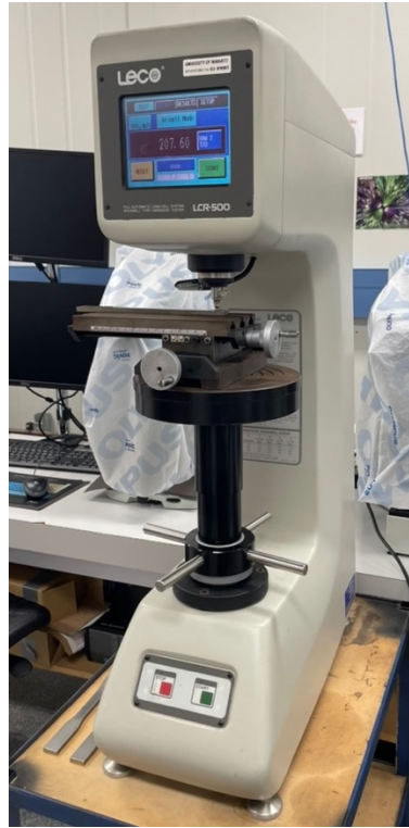
Figure 3.12: Leco LCR 500 dual tester for Rockwell and Brinell Hardness
