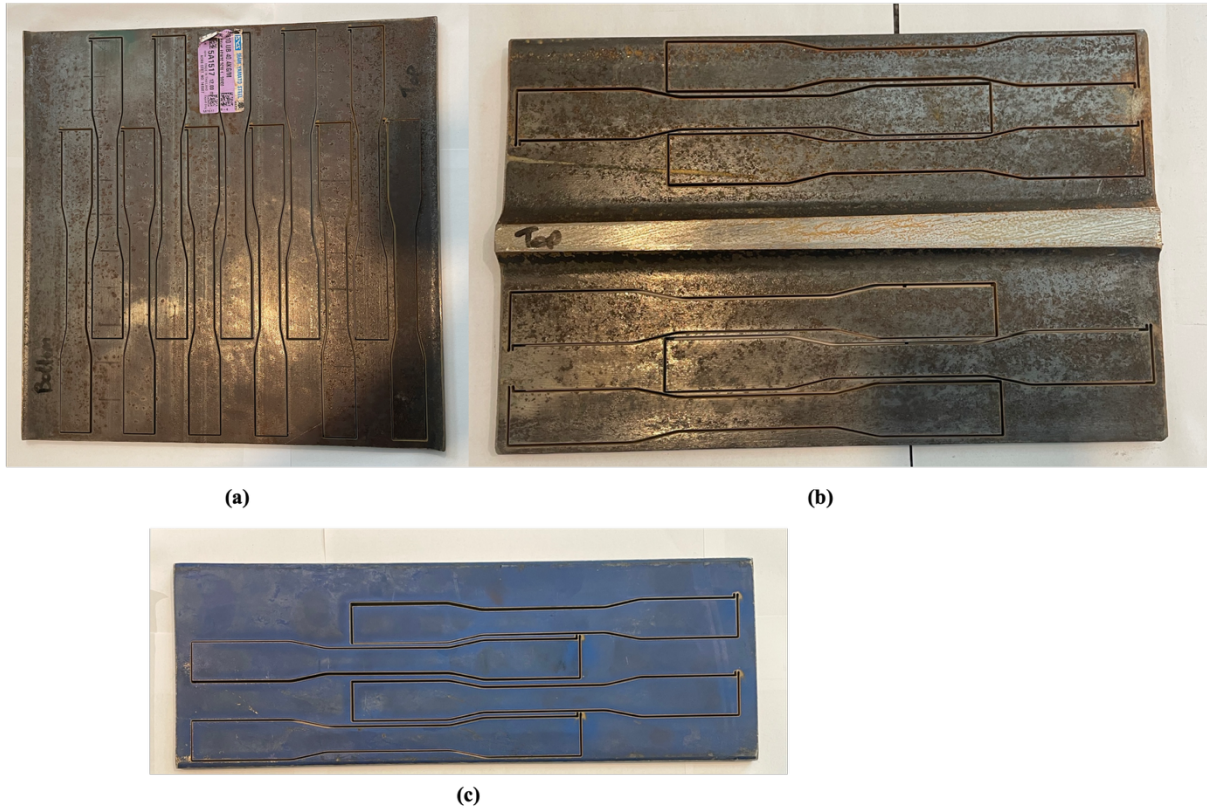
Figure 3.3: Specimen extraction layouts via water jet cutting to preserve microstructural integrity (a) UB Web (b) UB Flange (c) SHS
