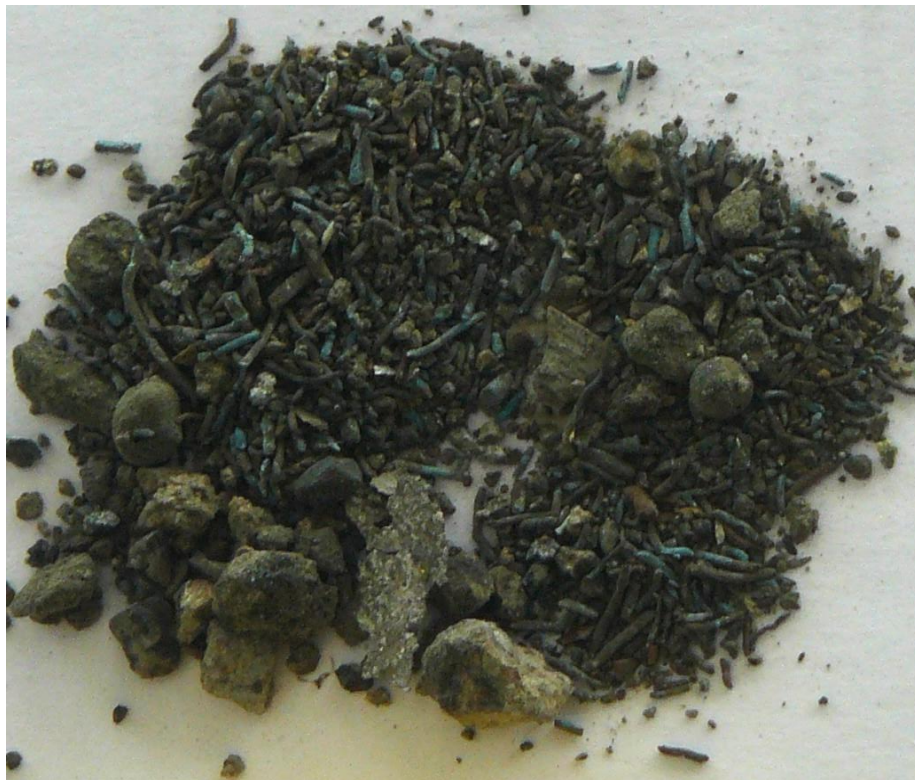
Figure 3-1. Rena polluted reef sediment sourced from high impact area on Otaiti. Copper filings can clearly be seen.
