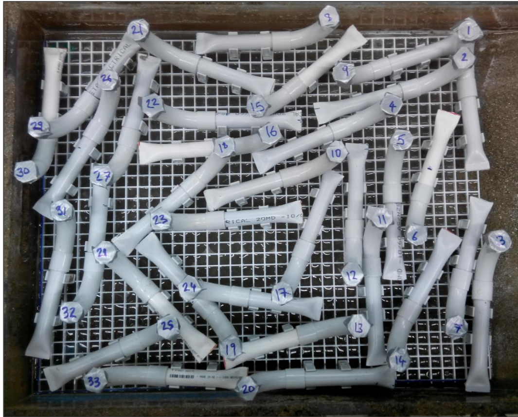
Figure 7: Crab burrow array in flume before burial showing positions of artificial burrows. Flow direction is from right to left.
