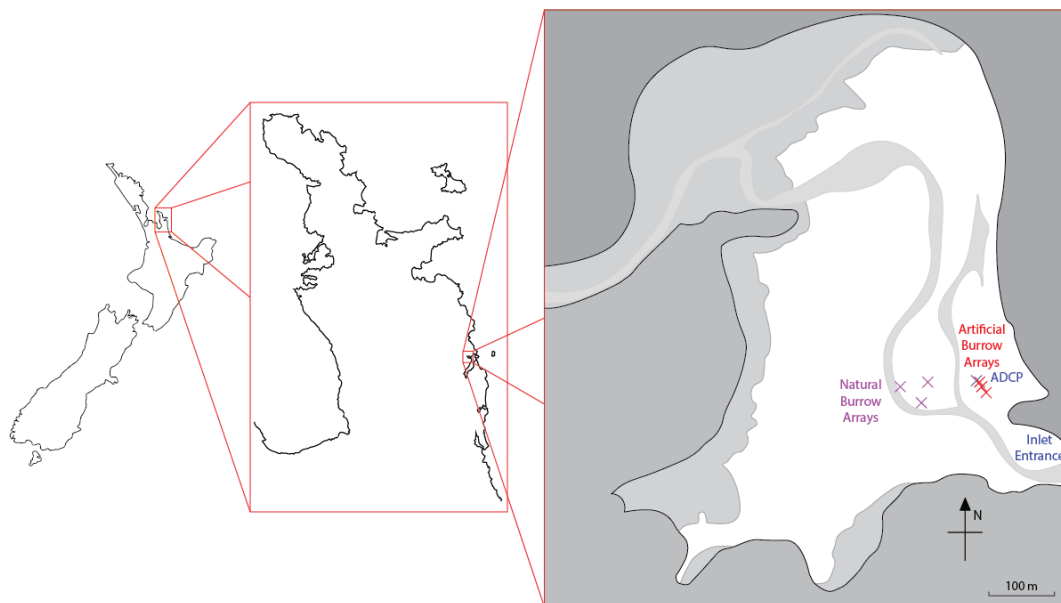
Figure 9: Site map of Pepe Inlet in Tairua Harbour, Coromandel, New Zealand. Red crosses show Vectrino Profiler positions above artificial crab burrows. Magenta crosses show Vectrino Profiler positions above natural crab burrows. The blue cross shows the location of the ADCP.
