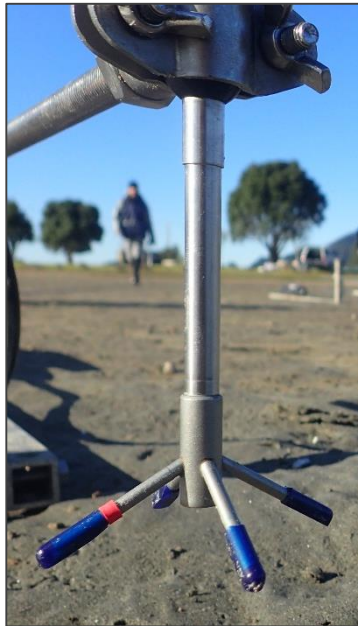
Figure 5: Probe end of the Nortek Vectrino Profiler Acoustic Doppler Velocimeter used for all experiments. The red tine indicates the x flow direction.
