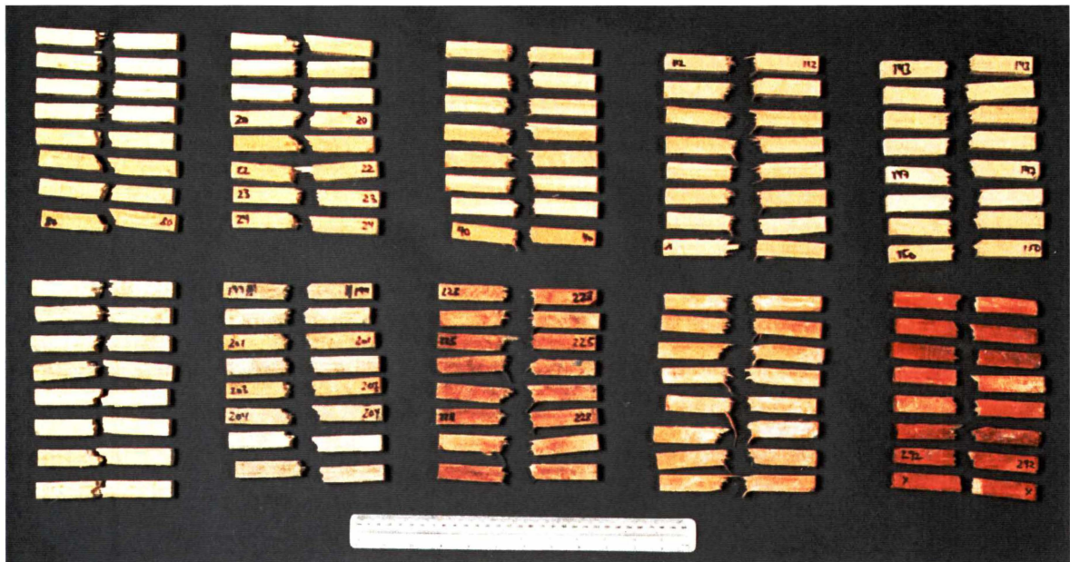
Figure 5.9: Radiata pine samples after toughness test (experiment II). Top row: controls; bottom row: matching samples, from left to right: O. piceae #272, L. procerum #1852, O. ips #308, S. commune and G. trabeum (moderately decayed).
