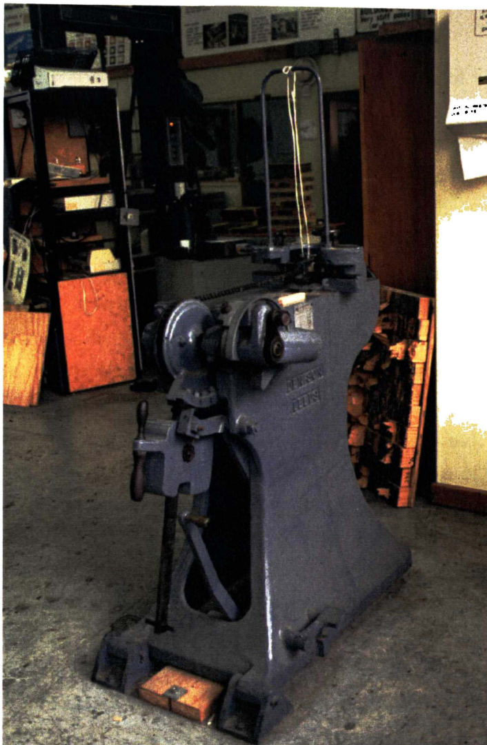
Figure 5.4: DENISON toughness tester in Forest Research Timber Engineering Laboratory, Rotorua.
