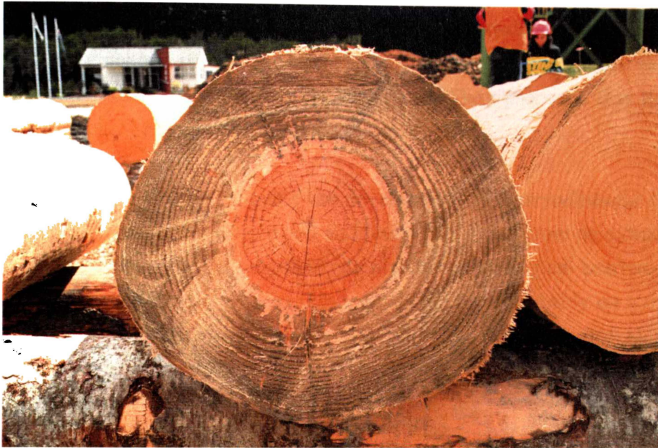
Figure 1.7: Discolouration of radiata pine sapwood by sapstaining fungi.
