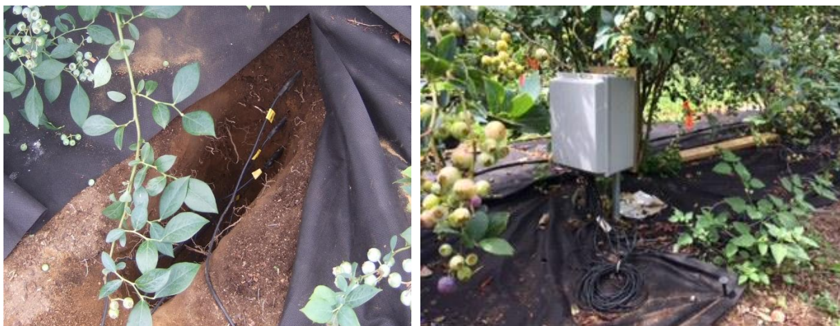
Figure. 3. Installation of soil moisture sensors at the depth of 10, 20, 30, and 50 cm (left) and a data logger (right).
