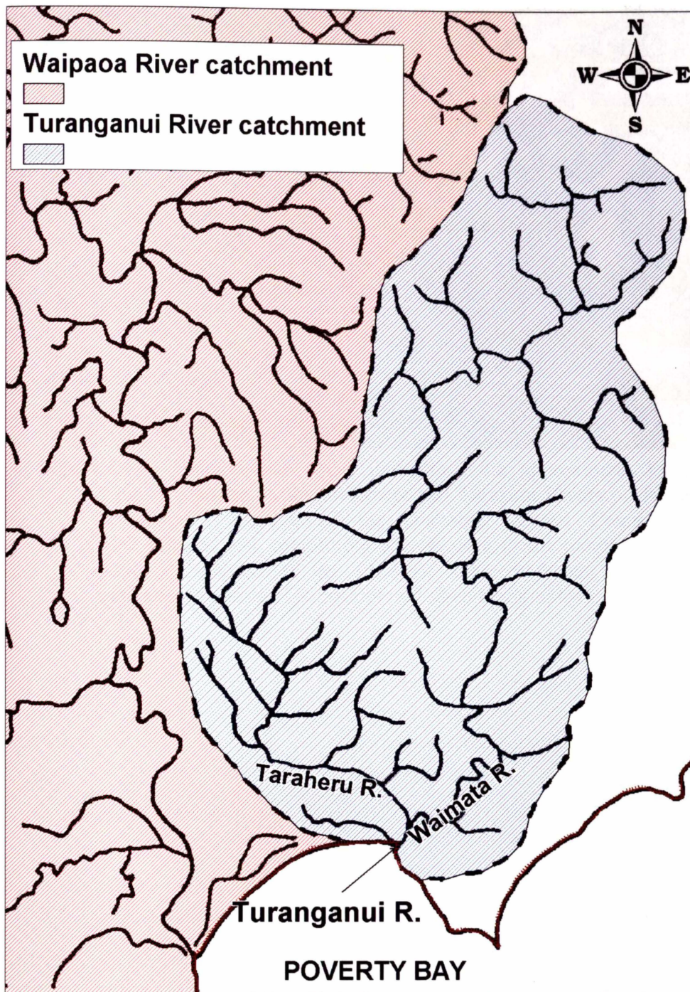
Figure 8.03 Turanganui River catchment, including the Waimata and Taraheru River catchment areas. The catchment consists of approximately 220 km 2 of highly erodible and faulted Tertiary sandstone and mudstone and crushed Cretaceous argillite (adapted from Kensington, 1990).
