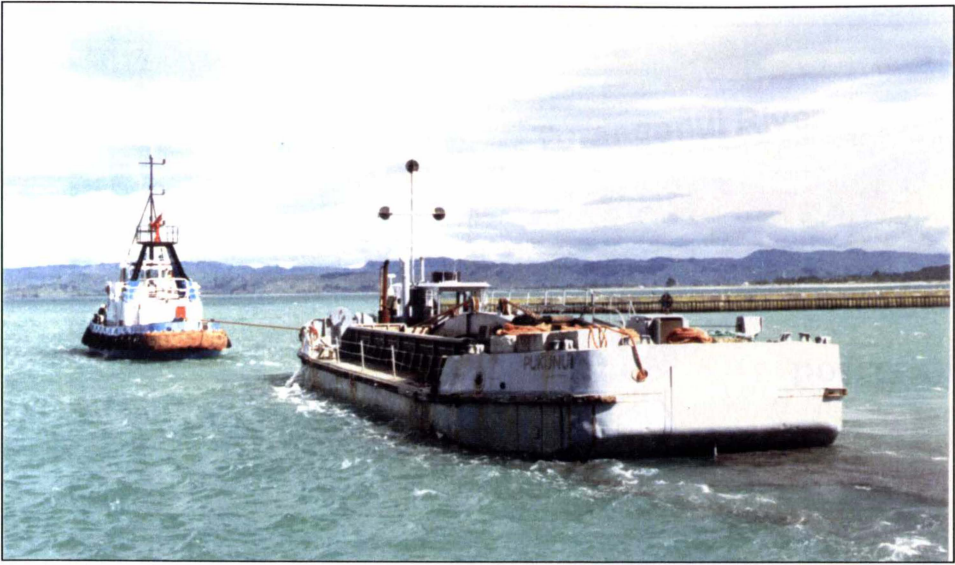
Figure 9.04 The cutter-suction dredge the Pukunui operated by Adsteam International; the maintenance-dredging contractors. The Pukunui is used to maintain the design depth of the shipping channel.
