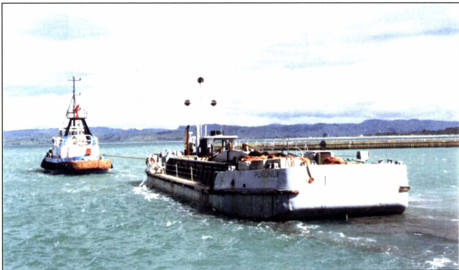
Figure 4.08 Cutter-suction dredge 'Pukunui' operated by Port Gisborne Ltd. for maintenance dredging of the shipping channel at the port of Gisborne.
