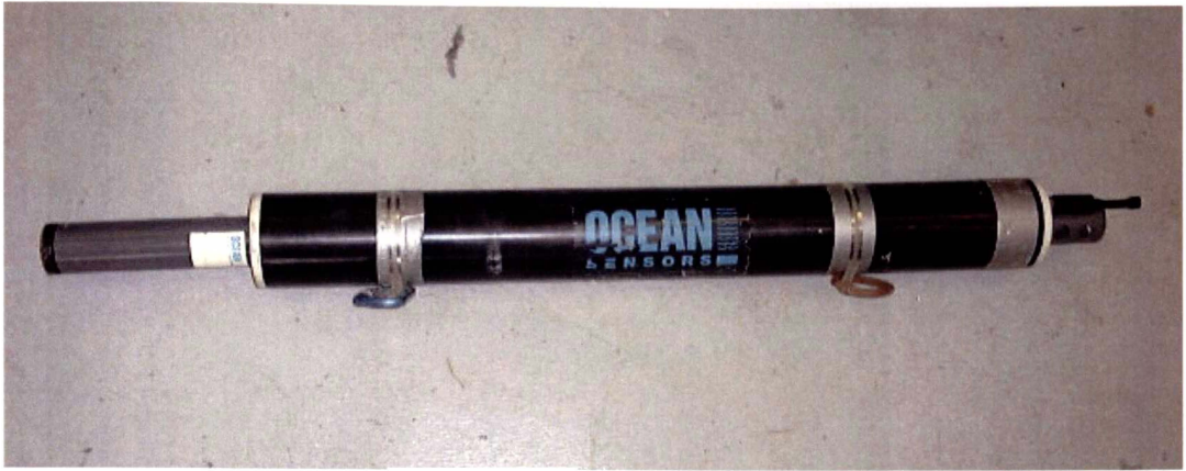
Figure 8.06 The Ocean Sensors CTD (Model OS200) instrument used to measure conductivity and temperature profiles in the port of Gisborne environs. The sensor is approximately 1.5 m in length. Cast locations are illustrated in Figure 8.05
