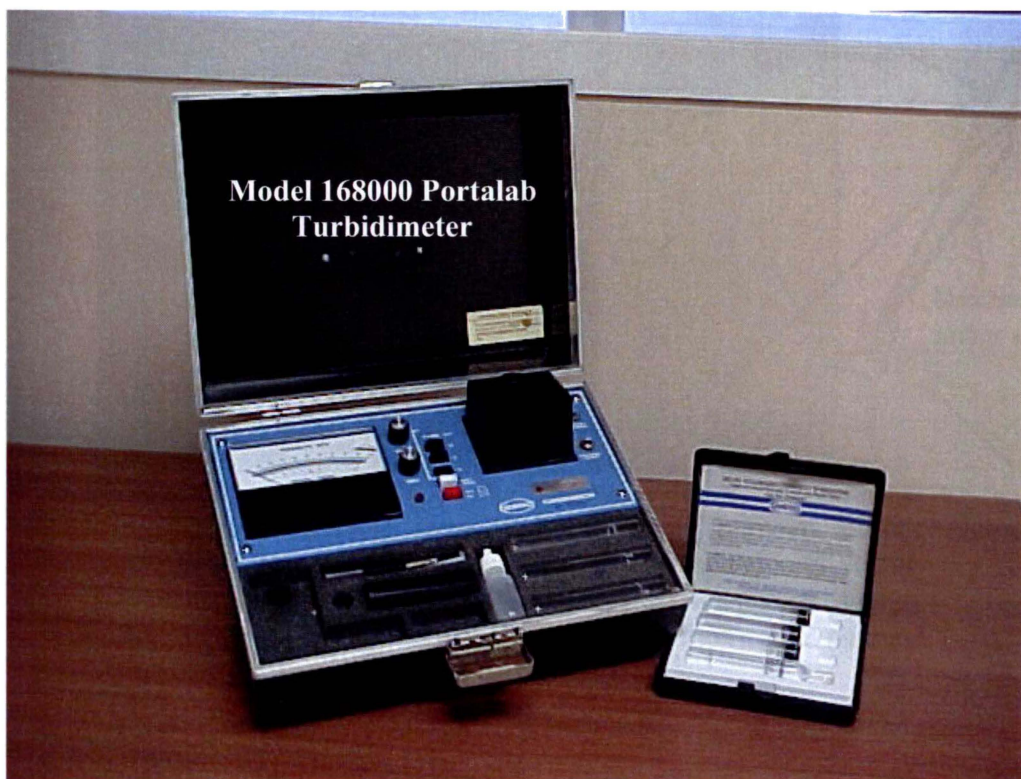
Figure 8.09 The Hach Portalab Turbidimeter (model 16800) and turbidity standards used to determine the relative turbidity of a solution in either field or laboratory conditions. The turbidity is measured in nephelometric turbidity units (NTU).
