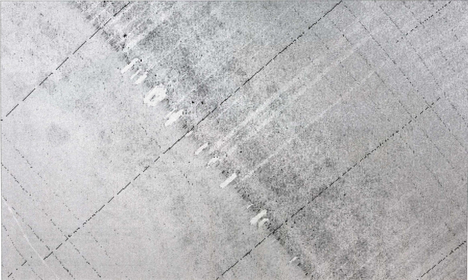
Figure 3.10 Close-up of the undifferentiated silty sand facies as identified from side-scan sonar record. The image shows lack of any large bedforms or rocky reef outcroppings.
