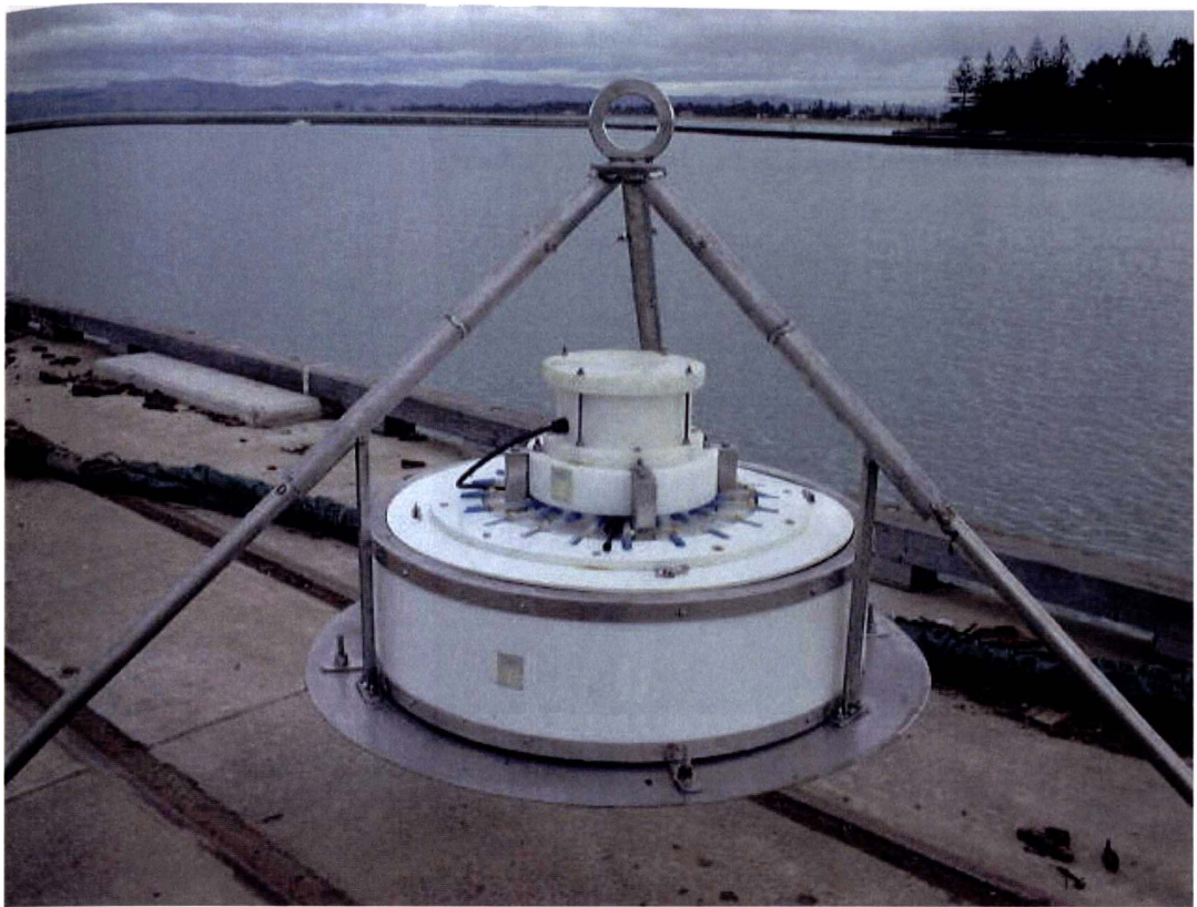
Figure 7.02 The Hydrocamel™ autonomous water sampler used to collect water and sediment samples for determination of the suspended sediment concentration and the near-bed reference concentration.
