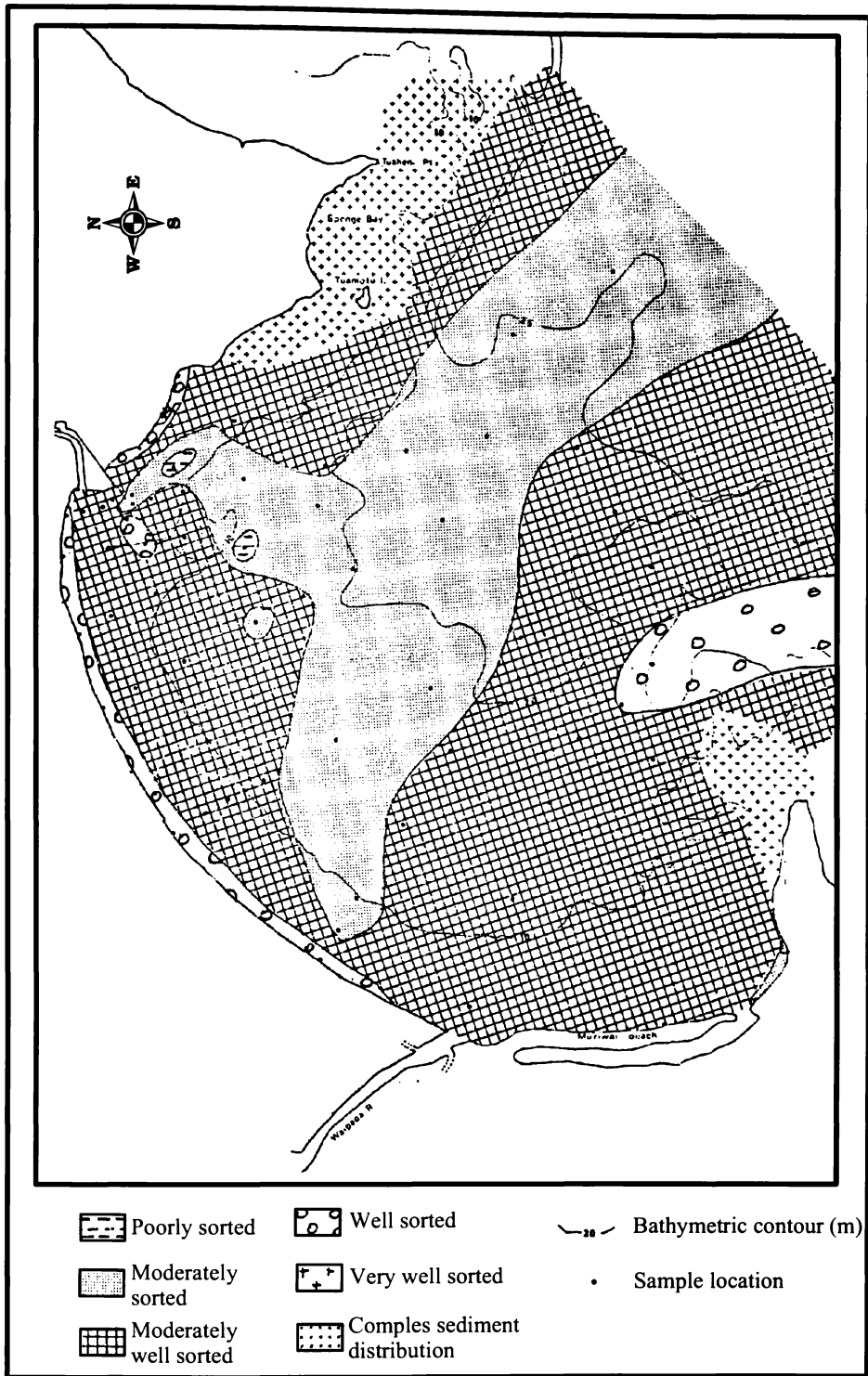
Figure 3.41 Map illustrating the spatial distribution of the surficial sediment sorting characteristics as measured by Miller, (1981). Miller determined that the majority of sediment within Poverty Bay (including northern Poverty Bay) was classified as being moderately well sorted, which is in contrast to the data collected as part of this study (Figure 3.23)
