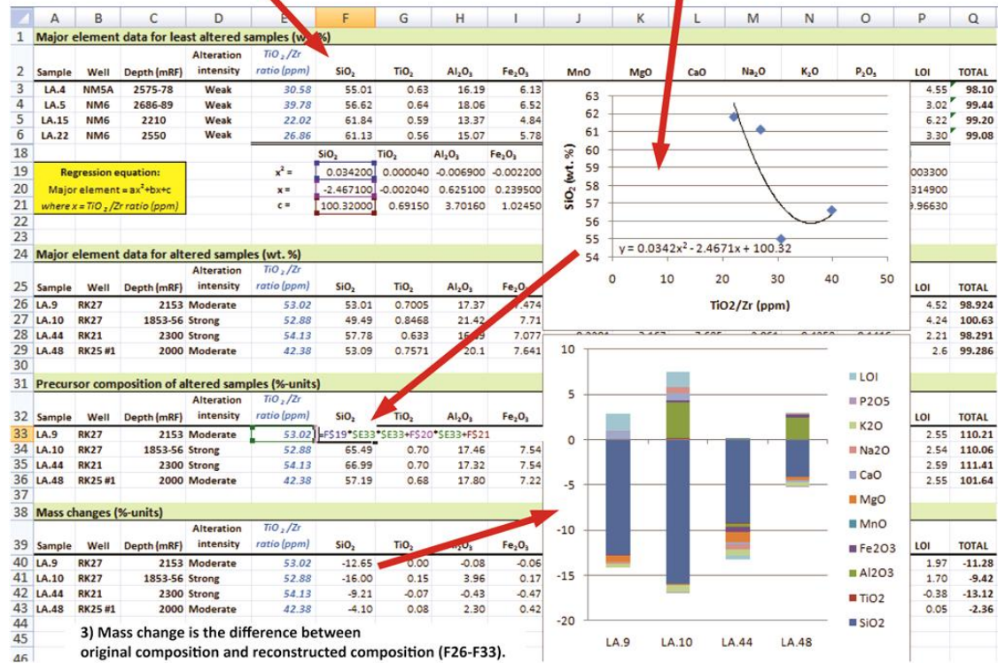
Figure 5.17: Example of layout and calculation of mass changes by multiple precursor method for 4 samples from Ngatamariki and Rotokawa fields.
