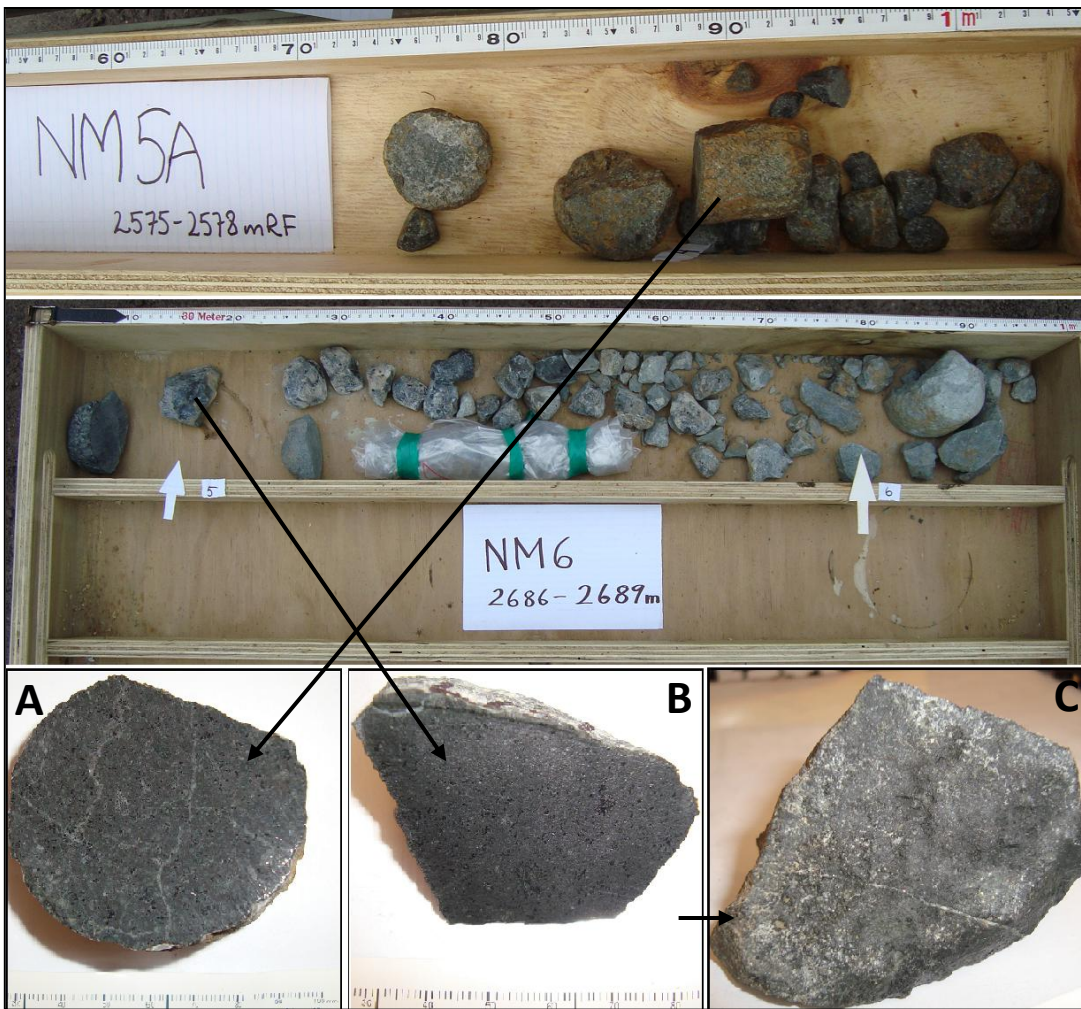
Figure 3.4: Box containing cores of andesite lava from a) NM6/2686-89 mRF sample LA.4, and b) NM5A/2575-78 mRF sample LA.5. c) Core surface of LA.5, showing patches of green chlorite, flaky white calcite and a calcite vein.
