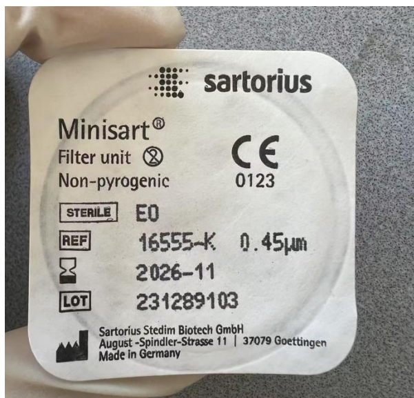
Figure 3.5. 0.45 µm Minisart® syringe filter (Sartorius, Germany) used for algae removal.
