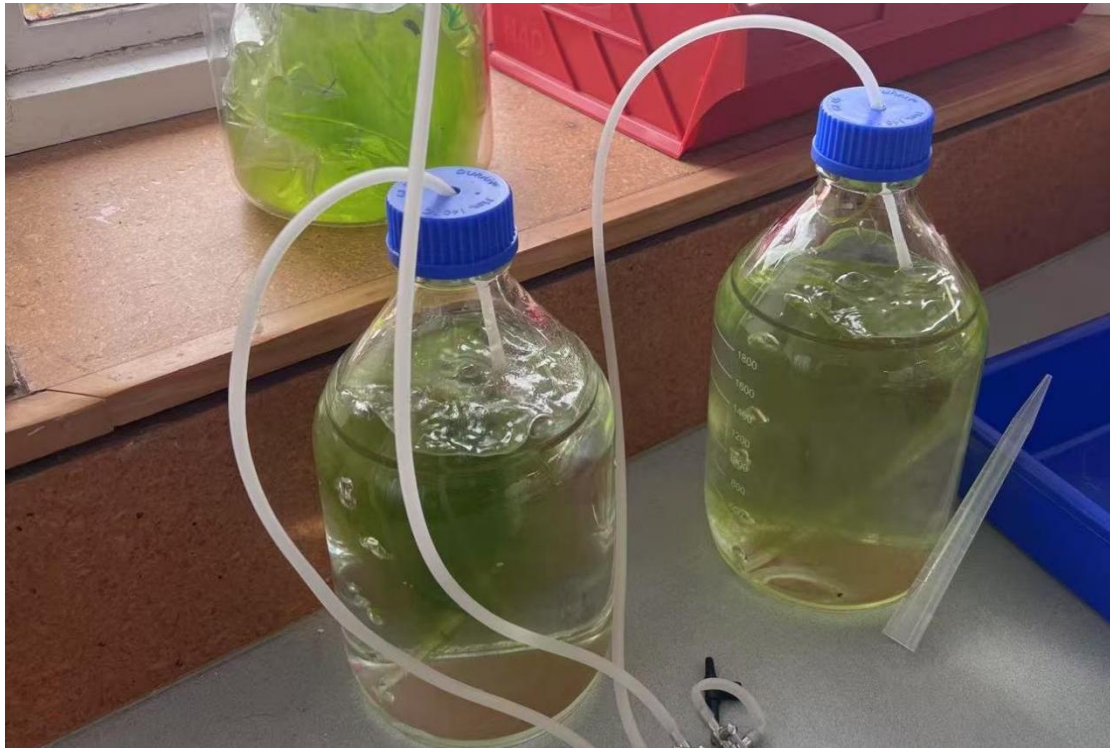
Figure 3.1. The first algal growing arrangement with 2-L glass bottles (Bottles No. 1 and 2) attached to an air pump.
