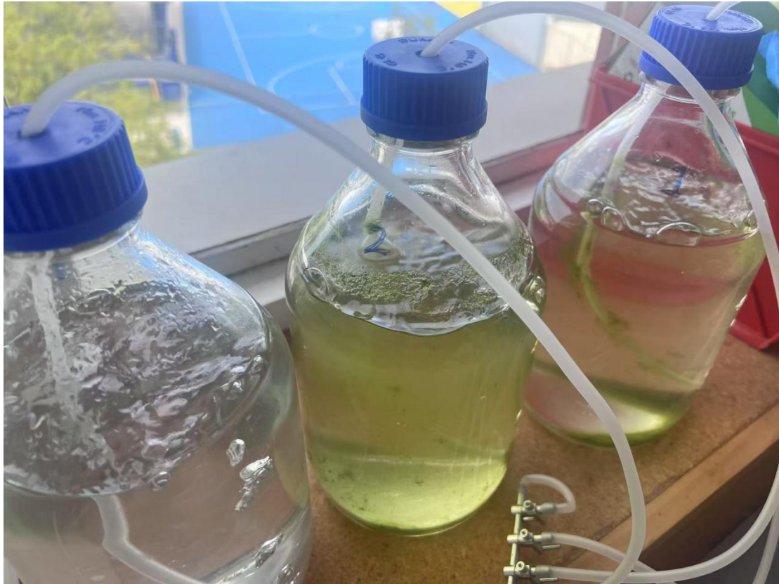
Figure 3.2. Algal propagation stage with the introduction of a third 2-L glass bottle (Bottle No. 3).
