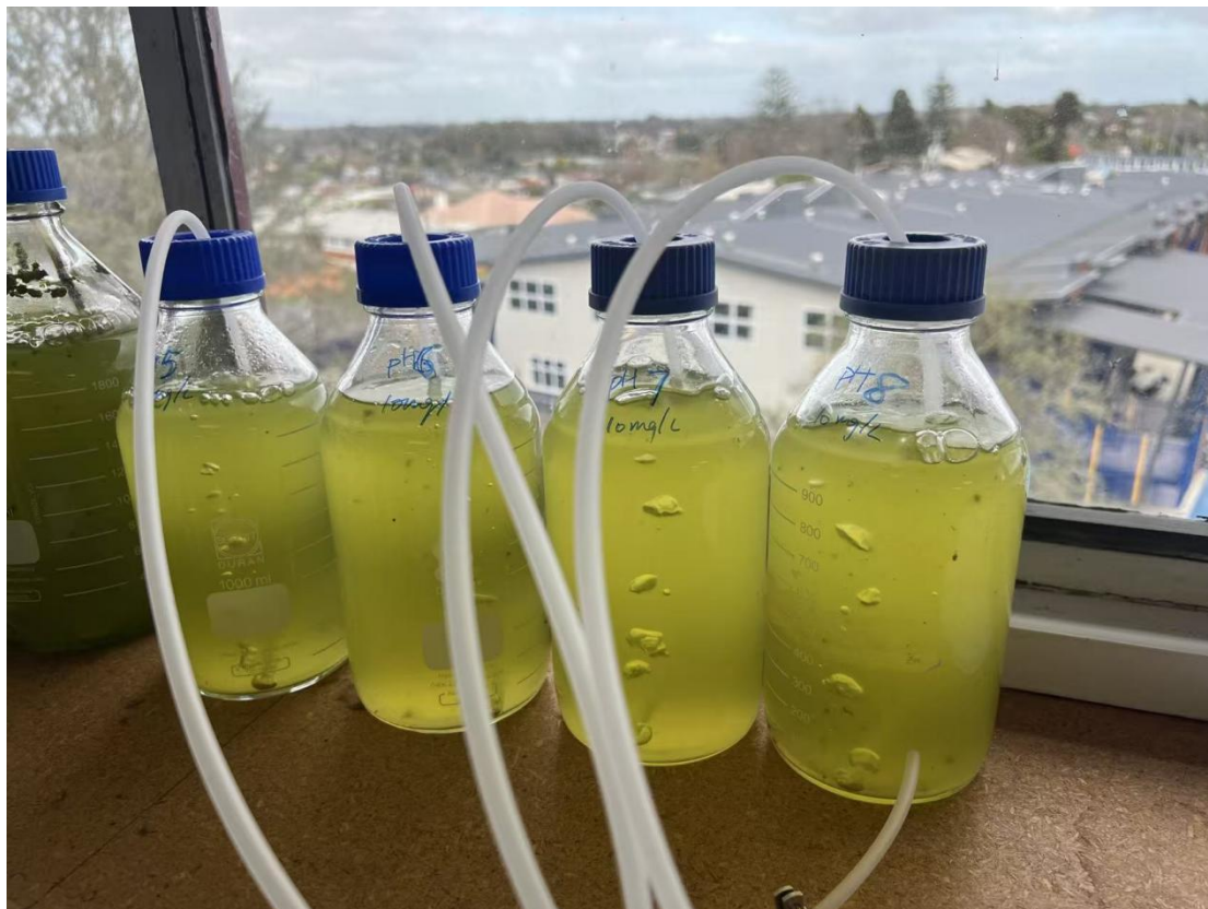
Figure 3.15. Four 1 L glass bottles for the algal treatment groups, under continuous aeration, in the initial pH buffered by phosphate buffers at 5, 6, 7, and 8. Estrone (E1) at an initial concentration of 10 mg/L
