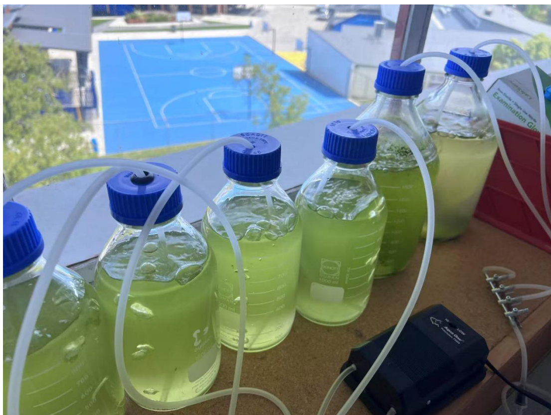
Figure 3.3. Stabilized algal cultures before experimental trials, grown in four 1-L experimental bottles with continuous aeration.
