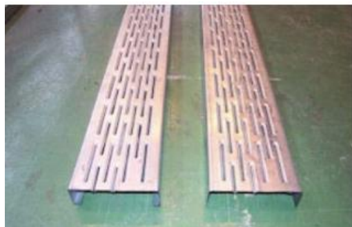
Fig.1- 1. Cold-formed steel stud with slits after Laboube [4]
