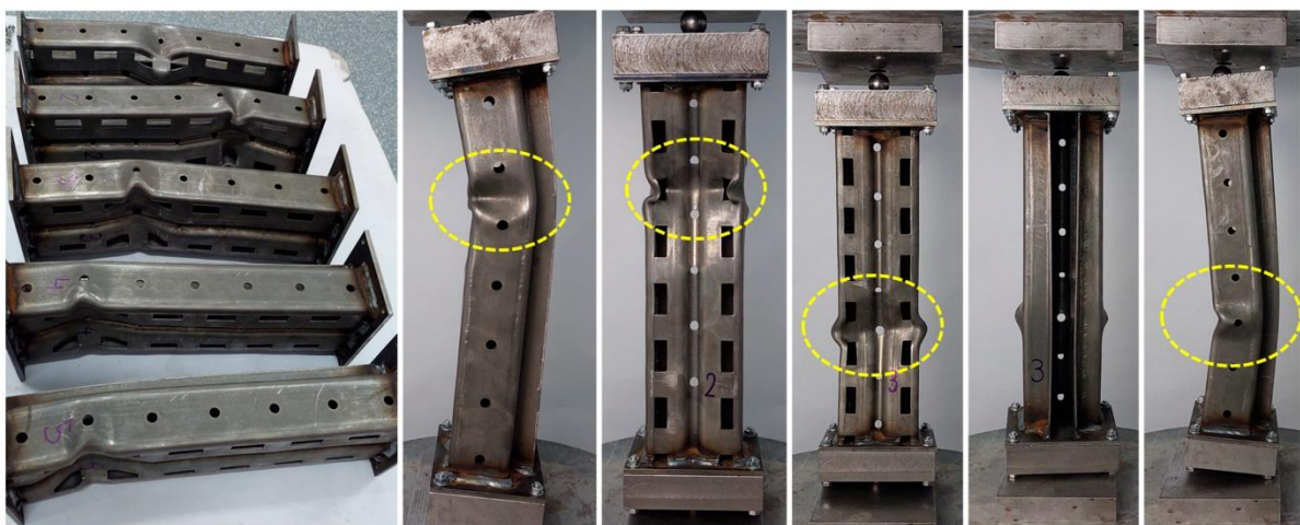
Fig. 2- 17. Influence of the perforation location on the local buckling mode as reported by Xiang et al. [56]
