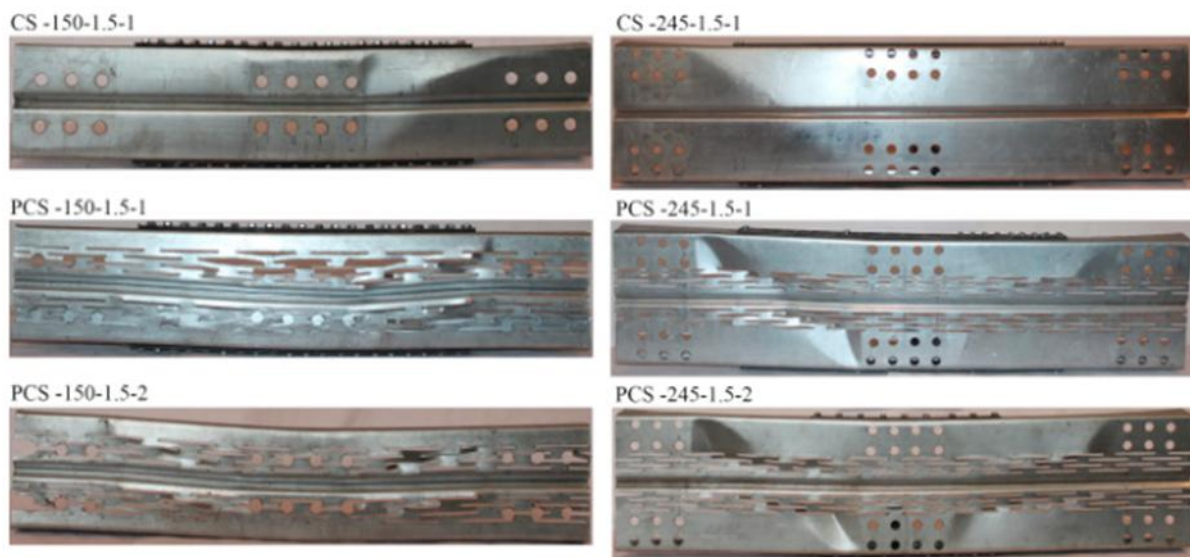
Fig. 2- 26. Failure modes of test specimens with stiffened webs [87].
