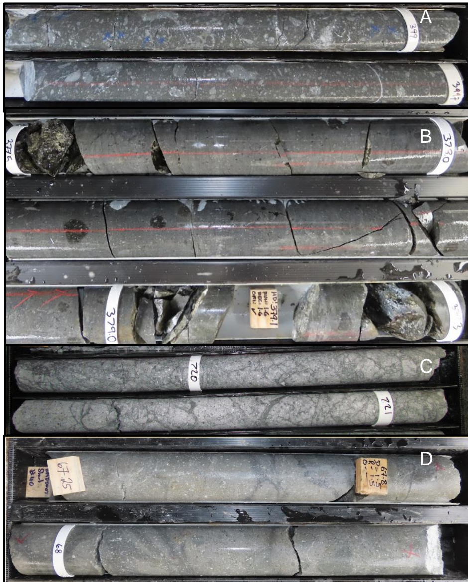
Fig. 4.5. Brecciated facies: (A) discrete brecciation, (B) sparse discrete brecciation, (C) mosaic brecciation, (D) weak mosaic brecciation.
